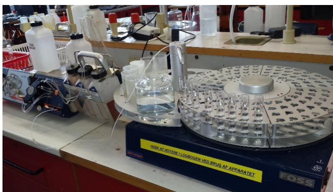
Figure C-3: FIAstar 5000 analyser and auto-sampler used for determination of total N.
