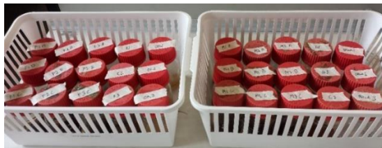
Figure D-6: Soil samples prepared for autoclaving at 120°C in 30 minutes and subsequent ICP-analysis.
