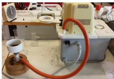
Figure F-12: All samples were vacuum filtered hot through Whatman 42 filter paper.
