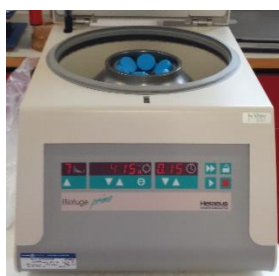
Figure I-3: The samples were centrifuged several times in a centrifuge at 2000 RPM for 15 minutes.
