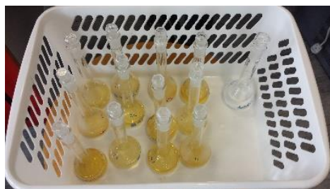
Figure F-13: All samples were added 4 drops of 1 M HNO 3 after filtration to prevent metal precipitation.
