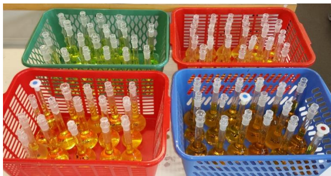
Figure H-5: Samples prepared for ICP-OES analysis of Cu and Zn concentration.
