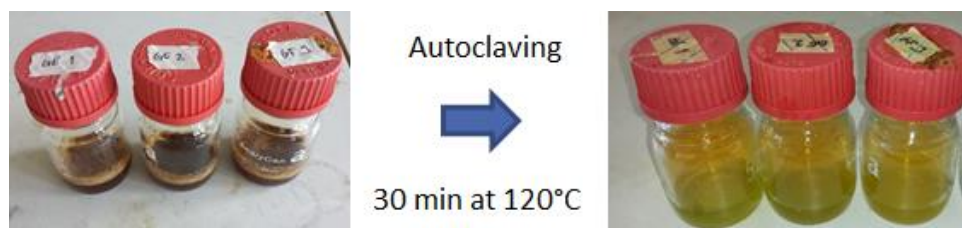
Figure C-6: Some manure samples before and after digestion.
