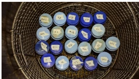
Figure D-8: Samples ready for autoclaving for 30 minutes at 120°C.
