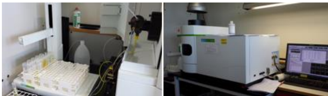
Figure A-2: ICP-OES used for metal analysis with auto sampler seen to the left.
