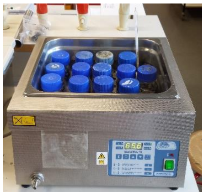
Figure F-11: The dried soil were mixed with 0.01 M CaCl 2 and heated at 90°C for 30 minutes.
