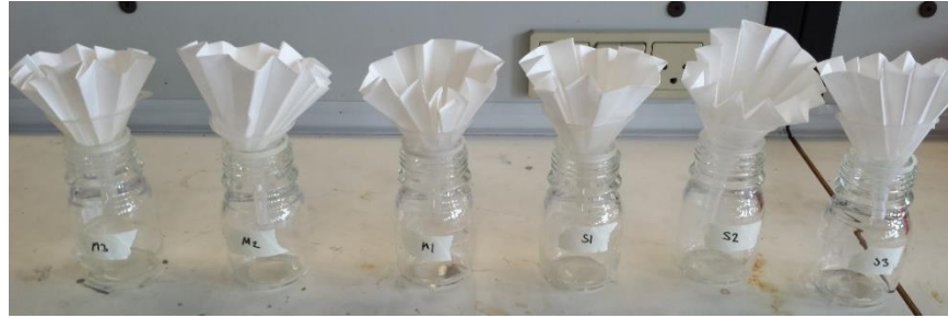
Figure I-6: Filtration of magnesium sulphate supernatant.
