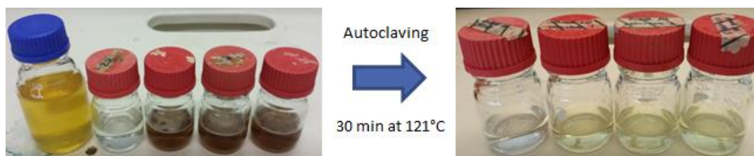
Figure A-1: Digestion of three sample of urine with \text{HNO}_3 and a blank made with demineralised water and \text{HNO}_3 .
