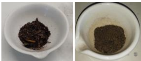
Figure C-2: The dried manure was transferred to a mortar and milled to a homogenous sample.
