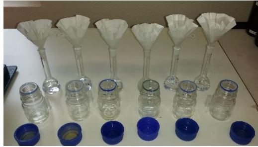
Figure C-5: All samples were filtered after autoclaving and diluted to 50 mL with demineralised water.
