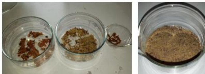
Figure B-2: Foodstuffs after drying (left) and milled tuna (right) prepared for digestion with nitric acid.
