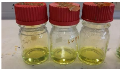
Figure B-3: Digestion solution with dried, milled tuna in nitric acid after autoclaving.
