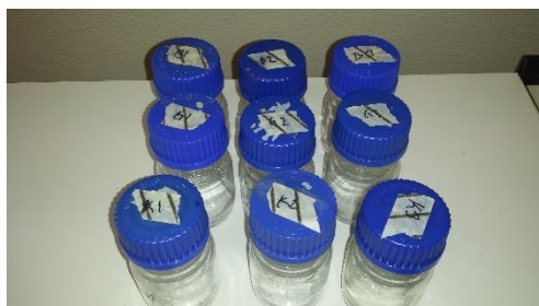
Figure C-4: Samples prepared for digestion with potassium peroxodisulphate solution.
