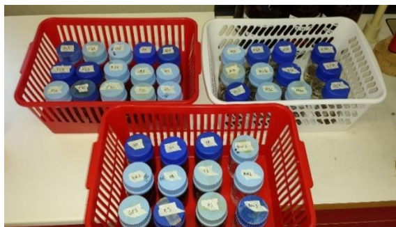
Figure D-7: Soil samples prepared for digestion with demineralised water and digestion solution (potassium peroxodisulphate solution).
