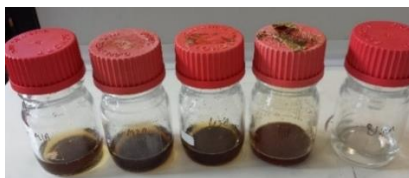
Figure D-5: Soil samples after drying, weighed and added 20 mL 7M HNO 3 for digestion.
