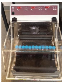
Figure I-2: Shaking incubator used for shaking of samples in the saturation and displacement procedure.
