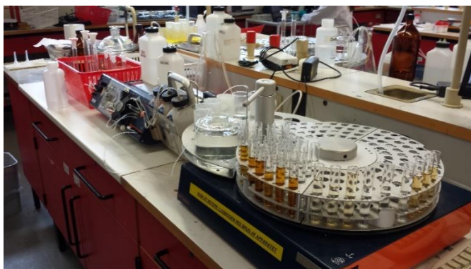
Figure D-9: Soil samples being analysed by FIAsstar 5000.
