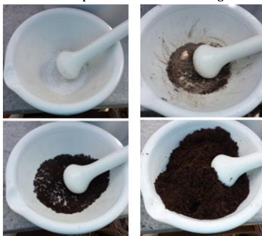
Figure F-1: The chemicals were added by thorough mixing with a continually increasing amount of soil in a mortar.
