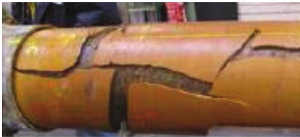
**Figure 1.3:** Failure of the outer layer of the flexible pipe [55].
