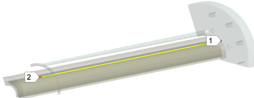
**Figure 8.8:** Path throughout the length of the bend stiffener.
