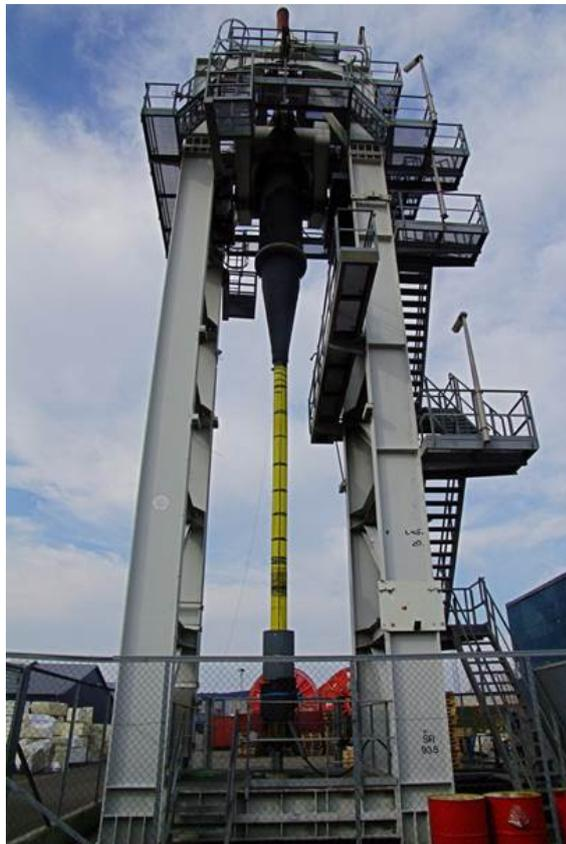
**Figure 2.14:** Test setup for testing the bend stiffener with different load cases [46].
