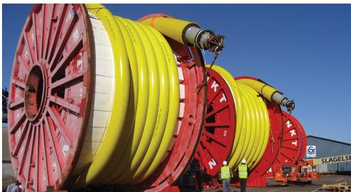
(a) Cable drum with pipe and bend stiffener [43].
