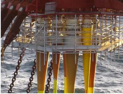
(a) Closeup of a collection of bend stiffeners [53].
