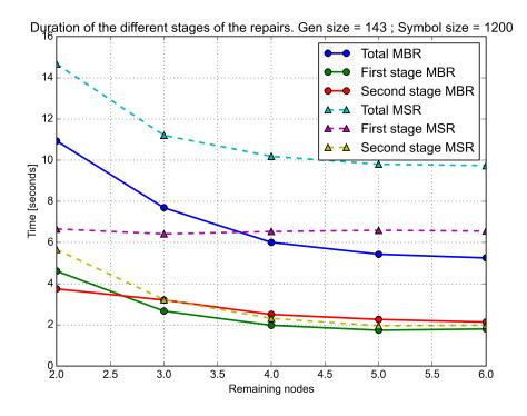
Figure 5.4: Comparison of the time spent in the different repair stages using MSR and MBR codes.
