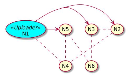
Figure 4.2: Upload session seen without the logical distinction of the *uploader* entity.
