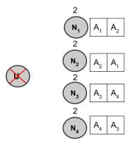
FIGURE 3.2: When the uploader disconnects, the nodes must take actions and copy the pieces they are storing into other nodes.
