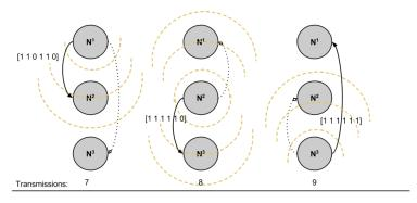
Figure 3.13: Final three transmissions of a repair session using broadcast messages.
