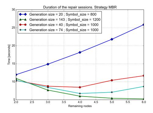
Figure 5.3: Total time spent in the repair sessions for different generation sizes and symbol size using MBR codes.
