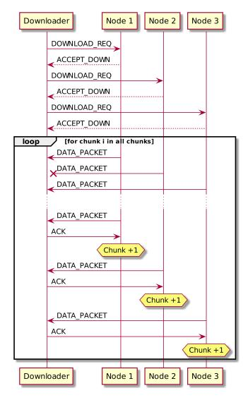
Figure 4.5: Example of messages exchanged between a downloader and three target nodes.
