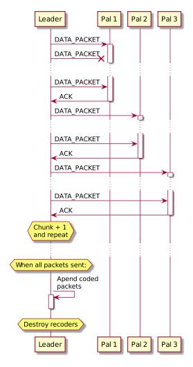
FIGURE 4.12: Example of the message sequence of the third stage of the repair with one leader and three pals. Each pal stores the received coded packets.
