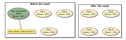
Figure 4.14: Actions that the reconnected peer must perform during the repair session when it must delete coded packets.
