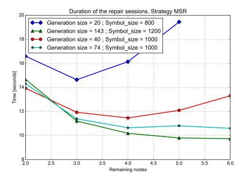
FIGURE 5.1: Total time spent in the repair sessions for different generation sizes and symbol sizes using MSR codes.
