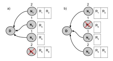
FIGURE 3.4: Example shows that when using coding 50% of redundancy can guarantee 100% reliability when any node disconnects. In both cases the file can be recovered.
