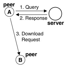
FIGURE 2.2: Search process in Napster. Image source: [23].
