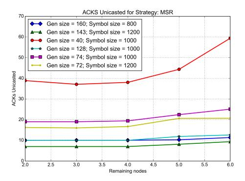
Figure 5.10: Total number of ack messages unicasted in the different repair sessions using MSR codes.
