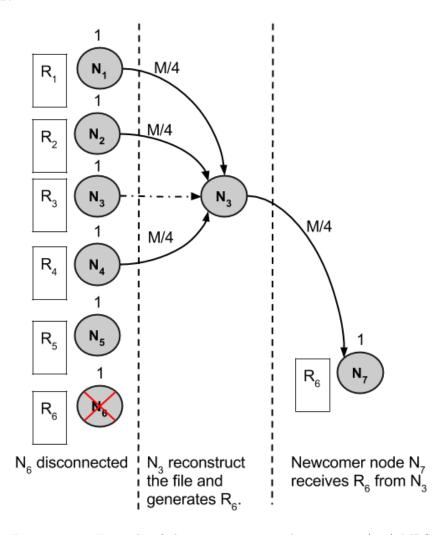
FIGURE 3.5: Example of the repair process when using a (6,4) MDS code. The whole file must be transferred over the network.
