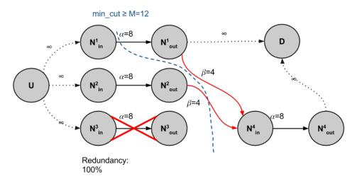
FIGURE 3.7: Example showing the information flow graph for MBR codes and a file of 12Mb stored in 3 nodes. All sizes are in Mb.
