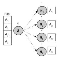
FIGURE 3.1: A node splits a file into four pieces and stores them into four different nodes.
