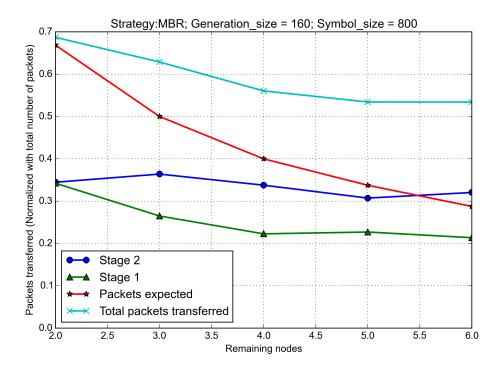
Figure 5.9: Total number of packets transferred (normalized) in the repair sessions using MBR codes.
