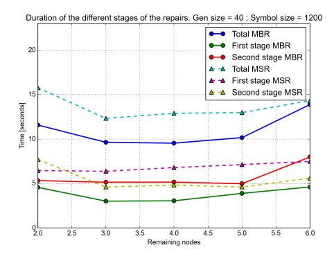
Figure 5.5: Comparison of the time spent in the different repair stages using MSR and MBR codes.
