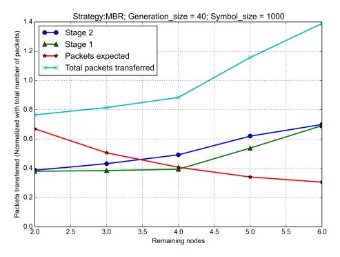
FIGURE 5.7: Total number of packets transferred (normalized) in the repair sessions using MBR codes.
