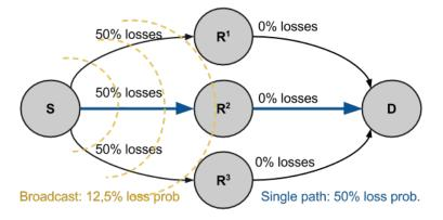
Figure 3.10: Example showing the advantages of spatial diversity in wireless networks
