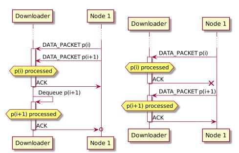
FIGURE 4.7: Scenario where multiple ACK messages are needed due to losses in the channel.
