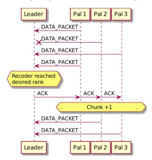
FIGURE 4.11: Example of the message sequence of the second stage of the repair with one leader and three pals.
