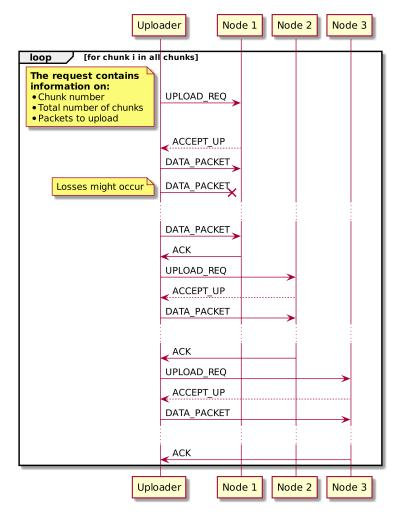
FIGURE 4.3: Example of messages exchanged between an uploader and three target nodes.
