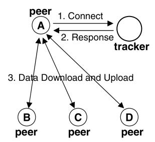
FIGURE 2.5: Search process in BitTorrent. Image source: [23].
