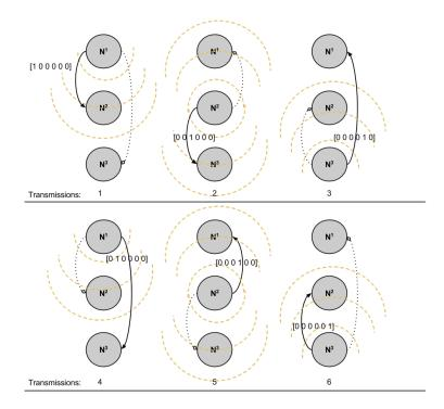
Figure 3.12: Initial six transmissions of a repair session using broadcast messages.
