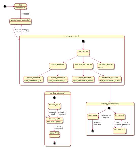
FIGURE 4.9: State diagram of the node object. It is the base of the application.
