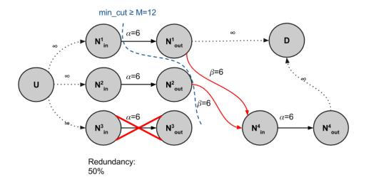
FIGURE 3.6: Example showing the information flow graph for MSR codes and a file of 12Mb stored in 3 nodes. All sizes are in Mb.
