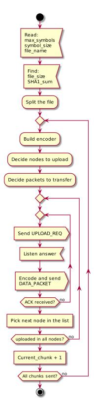
FIGURE 4.4: Flow diagram of the uploader object.
