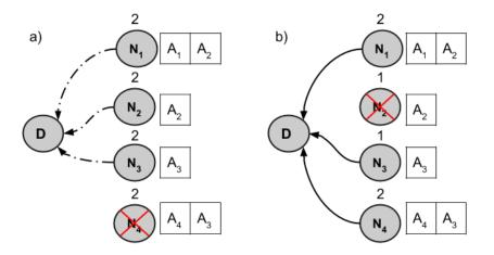
FIGURE 3.3: Example shows that 50% of redundancy cannot guarantee 100% reliability when any node disconnects. In case a) the file is not recoverable, in case b) the file can be recovered.
