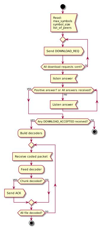
FIGURE 4.8: Flow diagram of the downloader object.
