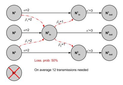
Figure 3.11: Example showing a simplified information flow graph of the repair session performed by 3 nodes storing a file of 6 pieces using MSR codes.
