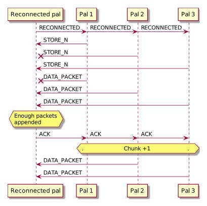
Figure 4.16: Messages sequence for a repair session due to reconnection where the reconnected peer must append coded packets.
