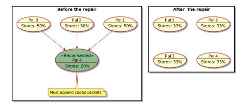
Figure 4.13: Actions that the reconnected peer must perform during the repair session when it must append coded packets.
