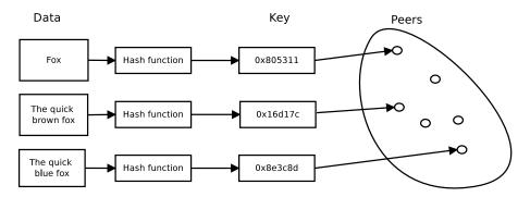
Figure 2.1: Distributed hash tables. Small variations in the input of a hash function results in big variations of the output
