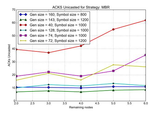
Figure 5.11: Total number of ack messages unicasted in the different repair sessions using MBR codes.
