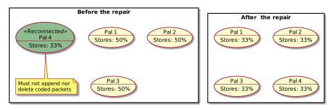
FIGURE 4.15: Actions that the reconnected peer must perform during the repair session when it must not delete nor append coded packets.
