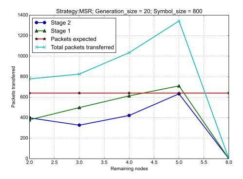
FIGURE 5.2: Total number of packets transferred in the repair sessions for different generation sizes and symbol sizes using MSR codes.
