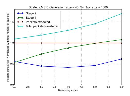
Figure 5.6: Total number of packets transferred (normalized) in the repair sessions MSR codes.
