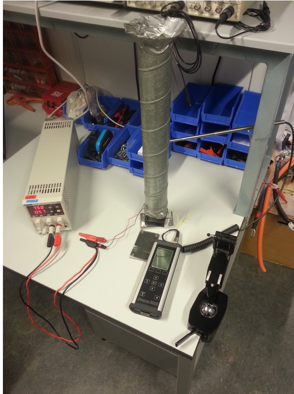
Figure .0.1: DC fan flow measurement setup.
