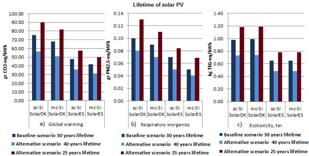
**Figure 6.6:** (Left) **a)** Global warming results for 30 (baseline scenario), 40 (alternative scenario) and 25 (alternative scenario) years lifetime of solar PV system, (Middle) **b)** Respiratory inorganics results for 30, 40 and 25 years lifetime of solar PV system, (Right) **c)** Ecotoxicity terrestrial results for 30, 40 and 25 years lifetime of solar PV system for Solar<sub>DK</sub> and Solar<sub>ES</sub> scenarios.
