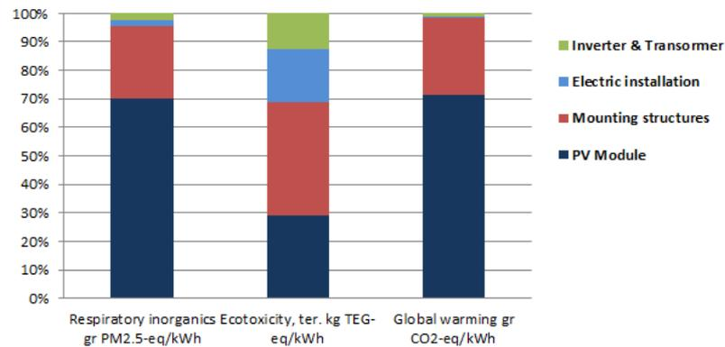
Figure 5.8: Main impact categories for manufacturing stage of solar PV system in Denmark, Solar<sub>DK</sub> scenario.
