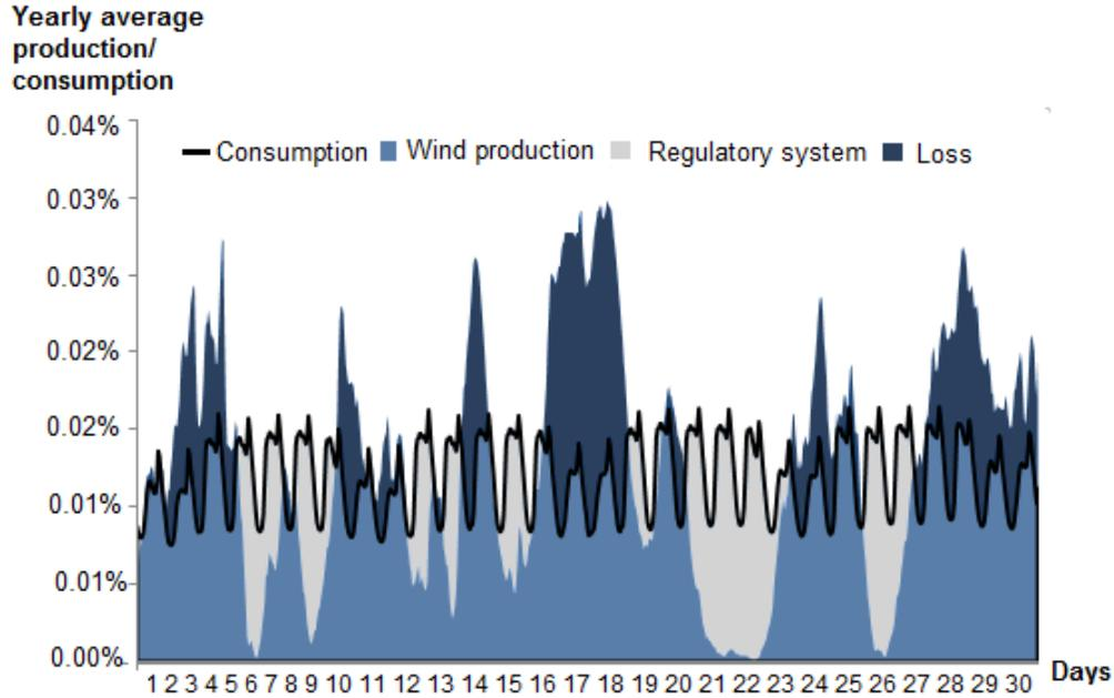
**Figure 3.3:** Calculations of need for regulatory system in wind production for one month in Denmark, based on data from [11]. Regulatory system refers to the wind production that is lower than the consumption, Loss refers to the wind production that is higher than the consumption.
