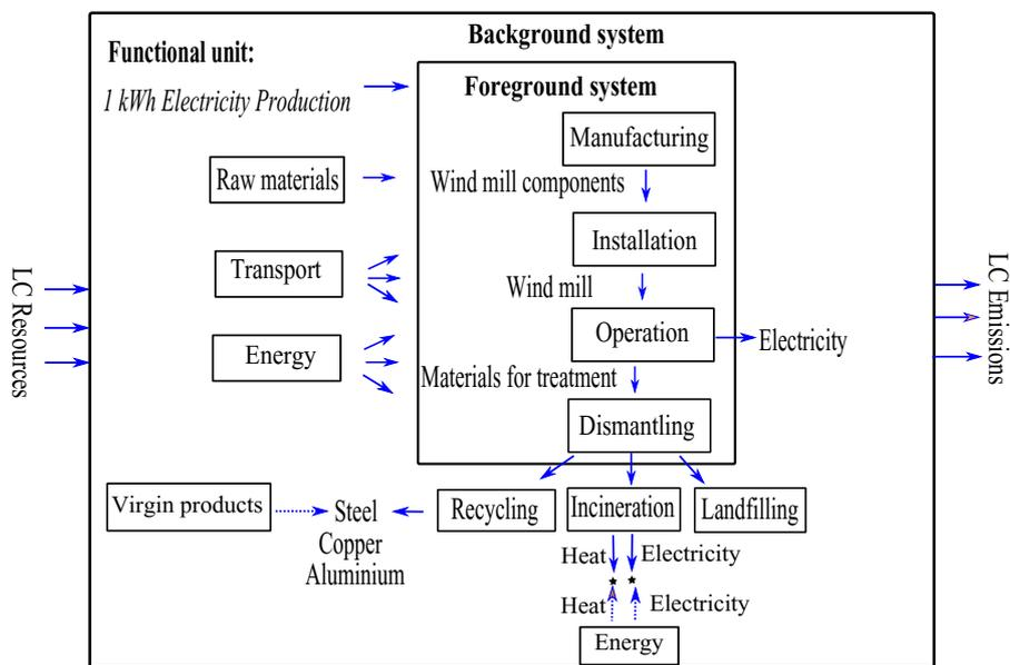
**Figure 3.4:** System boundaries for wind power plant, Wind<sub>DK</sub> and Wind<sub>ES</sub> scenarios.
