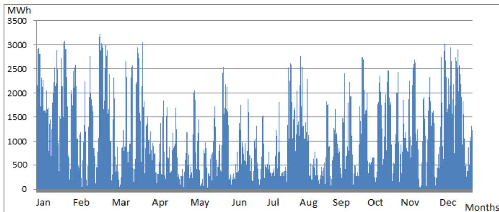
**Figure 3.1:** Hourly wind production per month for one year (2014) in Denmark, based on data from [11].
