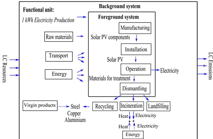
**Figure 3.5:** System boundaries of solar PV power plant,  $Solar_{DK}$  and  $Solar_{ES}$  scenarios.
