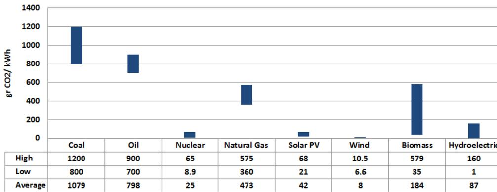
**Figure 1.1:** Life cycle GHG emissions intensity of electricity generation technologies based on: [51], [15], [45], [9], [50], [37], [6], [1], [38], [29], [27], [47], [19], [52].
