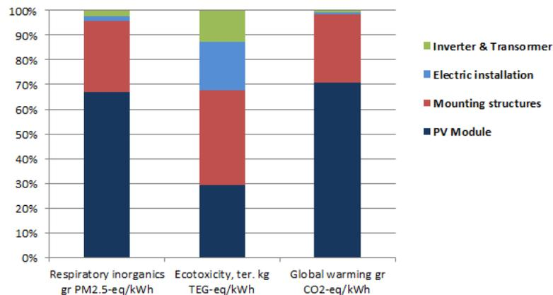
Figure 5.9: Main impact categories for manufacturing stage of solar PV system in Spain, Solar<sub>ES</sub> scenario.
