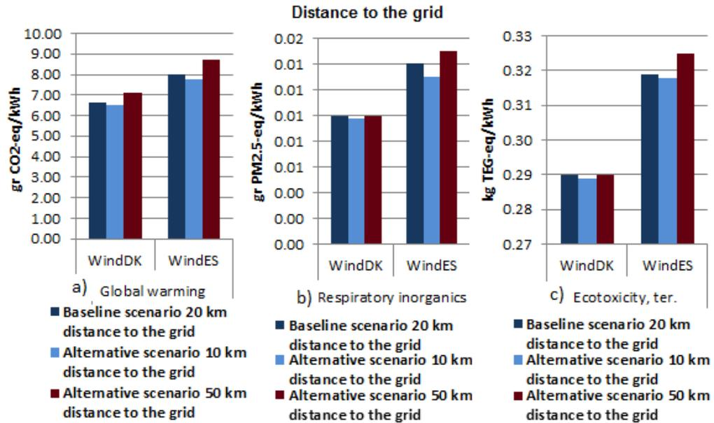
**Figure 6.2:** (Left) a) Global warming results for 20 km (baseline scenario), 10 km (alternative scenario) and 50 km (alternative scenario) distance to the grid, (Middle) b) Respiratory inorganics results for 20 km, 10 km and 50 km distance to the grid, (Right) c) Ecotoxicity terrestrial results for 20 km, 10 km and 50 km distance to the grid for Wind<sub>DK</sub> and Wind<sub>ES</sub> scenarios.
