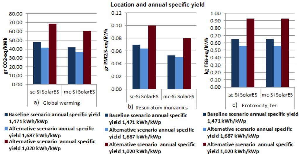
**Figure 6.9:** (Left) a) Global warming results for annual specific yield 1,471 kWh/kWp (baseline scenario), 1,687 kWh/kWp (alternative scenario) and 1,020 kWh/kWp (alternative scenario), (Middle) b) Respiratory inorganics results for annual specific yield 1,471 kWh/kWp, 1,687 kWh/kWp and 1,020 kWh/kWp, (Right) c) Ecotoxicity terrestrial results for annual specific yield 1,471 kWh/kWp, 1,687 kWh/kWp and 1,020 kWh/kWp based on [42] for Solar<sub>ES</sub> scenarios.
