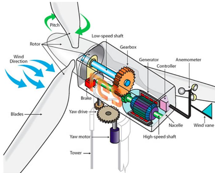
**Figure 4.1:** Main components of a wind turbine [35].
