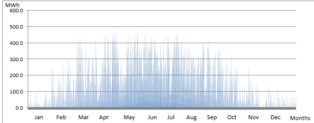
**Figure 3.2:** Hourly solar PV production per month for one year (2013) in Denmark, based on data from [11].
