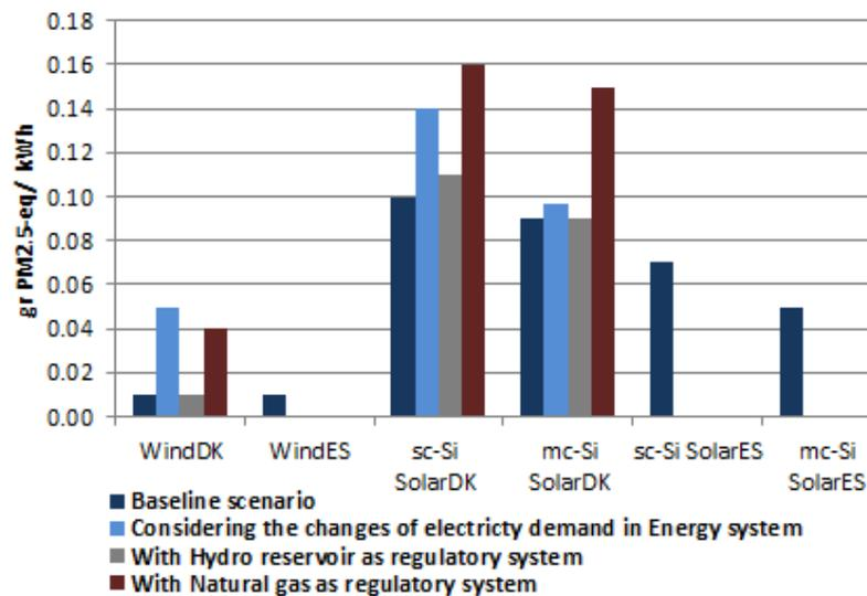
**Figure 5.2:** Respiratory inorganic for 30 MW wind farm (Wind<sub>DK</sub> and Wind<sub>ES</sub> scenarios) and 3 MW solar PV system (Solar<sub>DK</sub> and Solar<sub>ES</sub> scenarios) in Denmark and Spain. It is also presented the scenarios with the inclusion of the changes of electricity demand in energy system and the regulatory systems for Denmark. The results are presented per kWh electricity generation.
