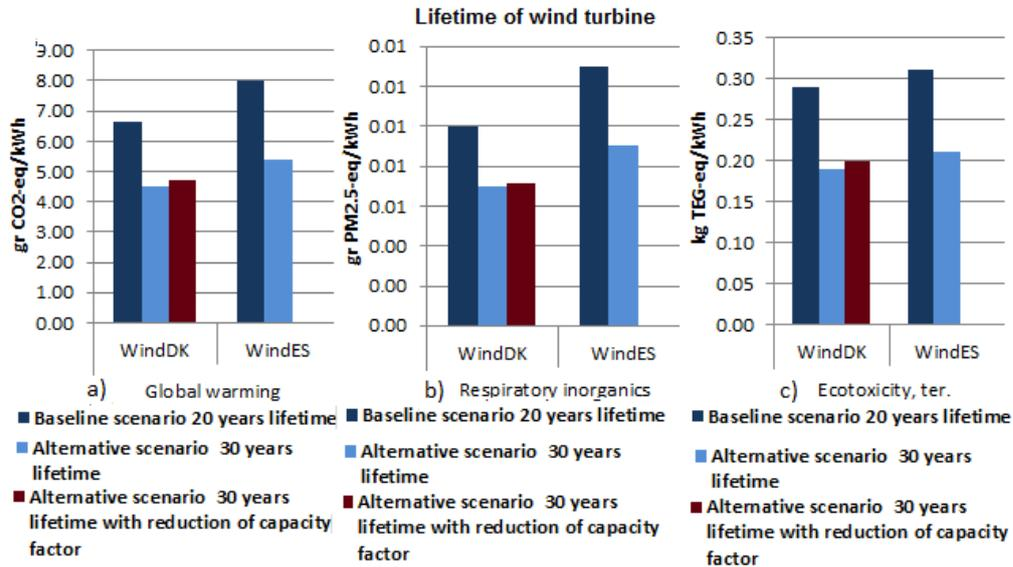
**Figure 6.1:** (Left) a) Global warming results for 20 (baseline scenario) and 30 (alternative scenario) years lifetime of wind turbine, (Middle) b) Respiratory inorganics results for 20 and 30 years lifetime of wind turbine, (Right) c) Ecotoxicity terrestrial results for 20 and 30 years lifetime of wind turbine for Wind<sub>DK</sub> and Wind<sub>ES</sub> scenarios.
