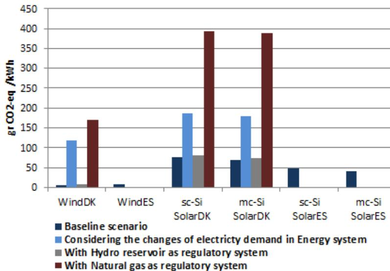
**Figure 5.3:** Global Warming Potential for 30 MW wind farm (Wind<sub>DK</sub> and Wind<sub>ES</sub> scenarios) and 3 MW solar PV system (Solar<sub>DK</sub> and Solar<sub>ES</sub> scenarios) in Denmark and Spain. It is also presented the scenario with the inclusion of the changes of electricity demand in energy system the regulatory systems for Denmark for Denmark. The results are presented per kWh electricity generation.
