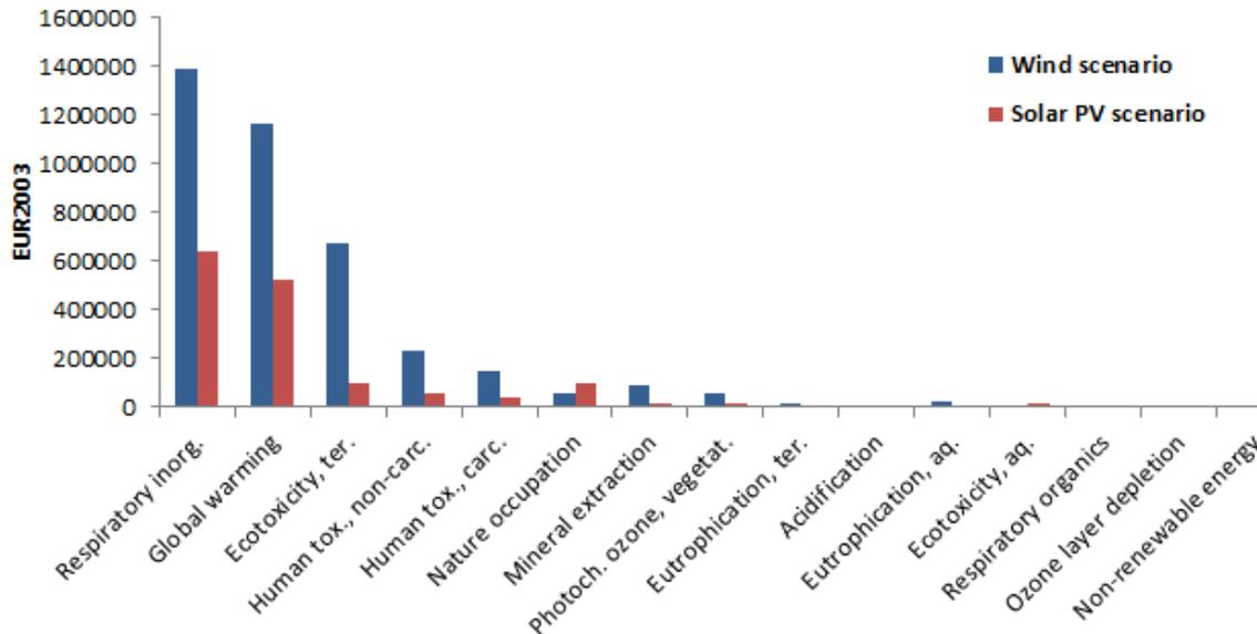
**Figure 5.1:** Results of Weighting comparison of wind and solar PV scenarios. The most significant impact categories start from the left side and end to the most insignificant.
