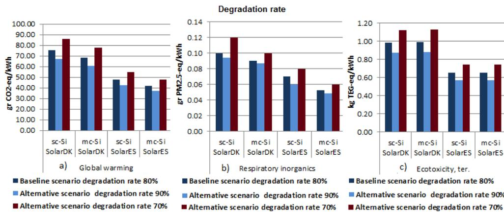
**Figure 6.7:** (Left) **a)** Global warming results for 80% (baseline scenario), 90% (alternative scenario) and 70% (alternative scenario) degradation rate of solar PV system, (Middle) **b)** Respiratory inorganics results for 80%, 90% and 70% degradation rate of solar PV system, (Right) **c)** Ecotoxicity terrestrial results for 80%, 90% and 70% degradation rate of solar PV system for Solar<sub>DK</sub> and Solar<sub>ES</sub> scenarios.
