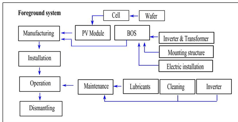
**Figure 3.7:** Foreground system of solar PV for 30 years lifetime,  $Solar_{DK}$  and  $Solar_{ES}$  scenarios.
