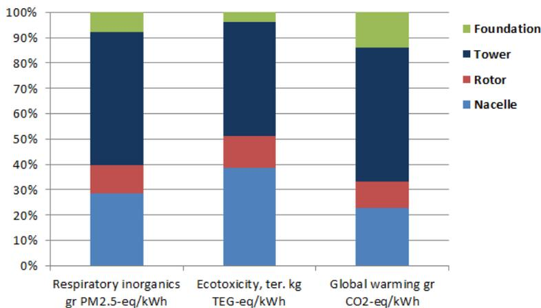
**Figure 5.7:** Main impact categories for manufacturing stage of wind turbine in Spain, Wind<sub>ES</sub> scenario.
