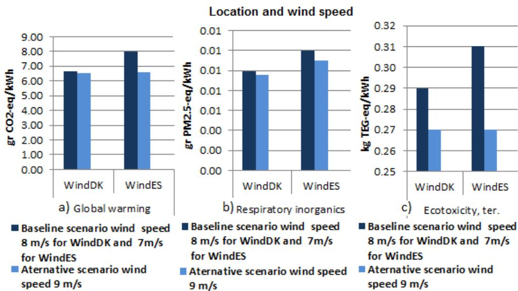
**Figure 6.4:** (Left) **a)** Global warming results for wind speed 8 m/s for Wind<sub>DK</sub> and 7m/s for Wind<sub>ES</sub> (baseline scenario), 9 m/s (alternative scenario), (Middle) **b)**Respiratory inorganics results for wind speed 8 m/s for Wind<sub>DK</sub> and 7m/s for Wind<sub>ES</sub>, 9 m/s, (Right) **c)** Ecotoxicity terrestrial results for wind speed 8 m/s for Wind<sub>DK</sub> and 7m/s for Wind<sub>ES</sub>, 9 m/s for Wind<sub>DK</sub> and Wind<sub>ES</sub> scenarios.
