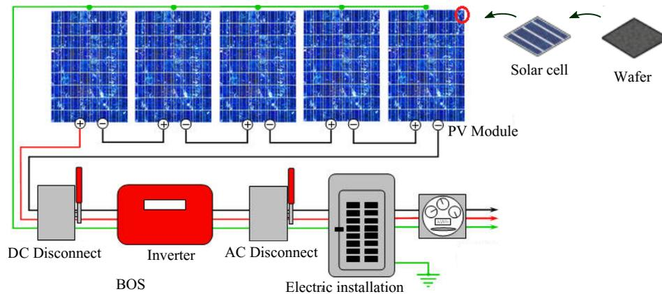
**Figure 4.2:** Main components of a solar PV system based on [3].
