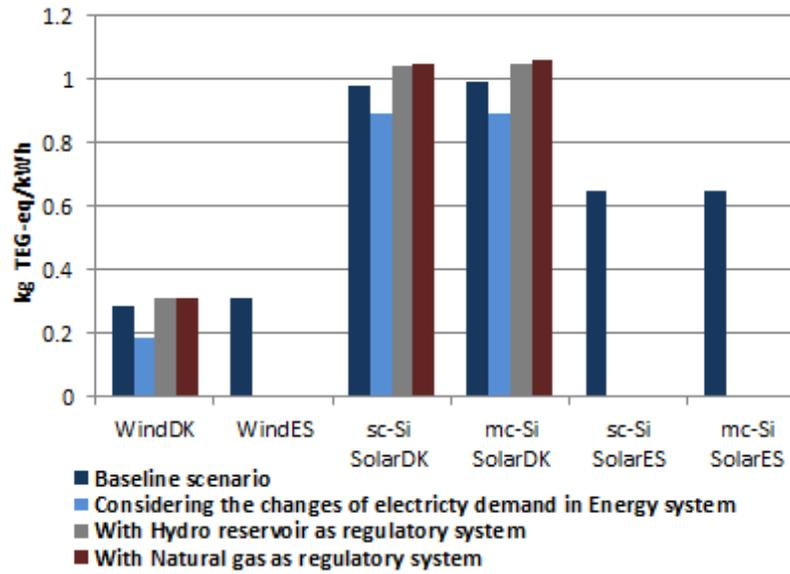
**Figure 5.4:** Ecotoxicity terrestrial for 30 MW wind farm (Wind<sub>DK</sub> and Wind<sub>ES</sub> scenarios) and 3 MW solar PV system (Solar<sub>DK</sub> and Solar<sub>ES</sub> scenarios) in Denmark and Spain. It is also presented the scenario with the inclusion of the changes of electricity demand in energy system the regulatory systems for Denmark for Denmark. The results are presented per kWh electricity generation.
