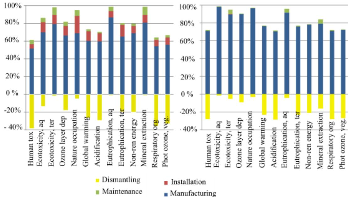
**Figure 5.5:** LCA results for life cycle stages of 30 MW wind farm (left) and 3 MW solar PV system (right).
