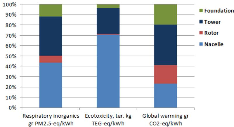
**Figure 5.6:** Main impact categories for manufacturing stage of wind turbine in Denmark, Wind<sub>DK</sub> scenario.
