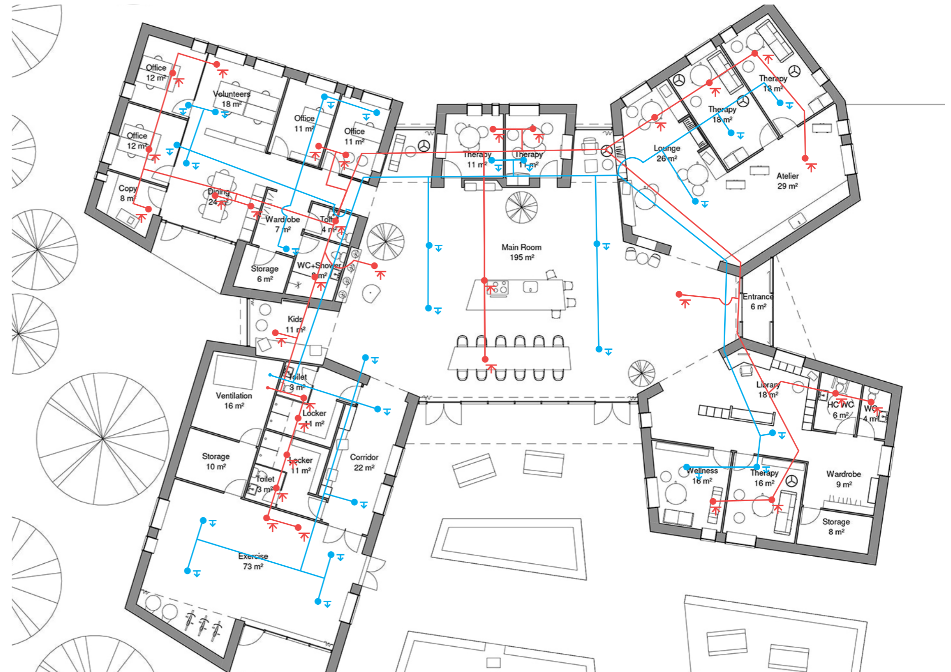
Illustration 222. Ventilation ducts (Plan 1:200)
