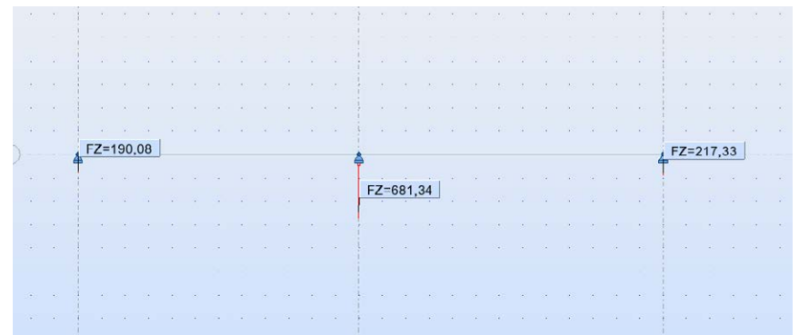
Screenshot from Robot Structural Analysis. Beam with the additional load of the roof.
