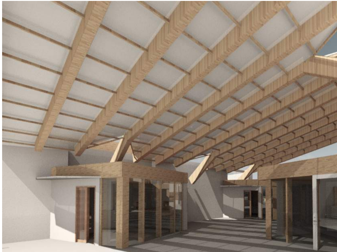
ill. 7.3a :: structure 1 :: three-dimensional beam defining glass element
