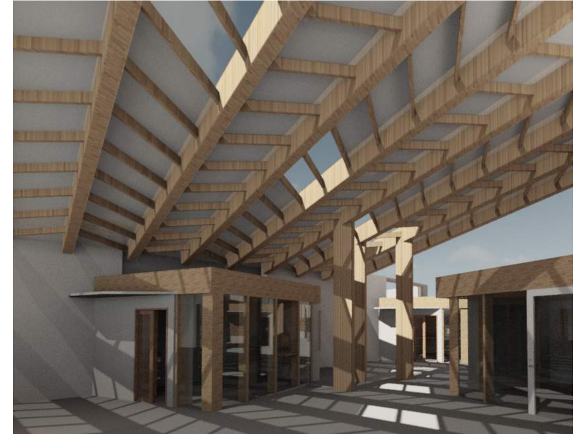
ill. 7.3b :: structure 2 :: the purlins of the structure creating a herringbone pattern which defines glass partitions that simulate the flow on the ground
