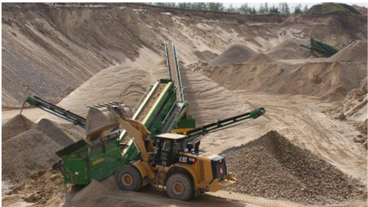
Illustration 4: Sortering (harpning) i grusgrav. [Danmarks Radio, 2015]
