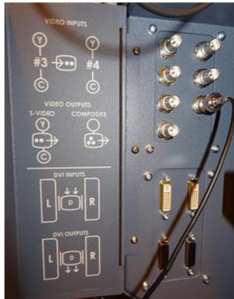
Figure 2.8 Hatch on the surgeon console covers the TilePro inputs and additional outputs.
