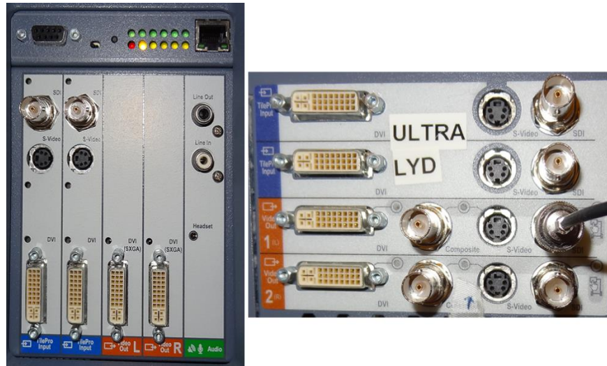
Figure 2.10 Left: Back of the console has TilePro inputs and stereo DVI outputs. Right: VEK with TilePro inputs and adjustable stereo output in different formats.
