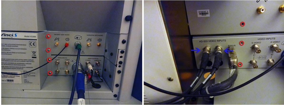
Figure 2.7 Left: Removing the four screws marked with red and three more screws to the left lets you remove the cover. Right: Behind the cover are the video inputs (blue) from the camera controllers.
