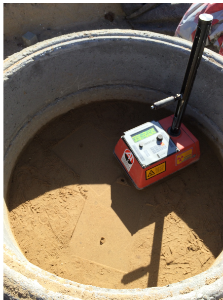
Figur 3.17. CPN isotopsonde i testform.
