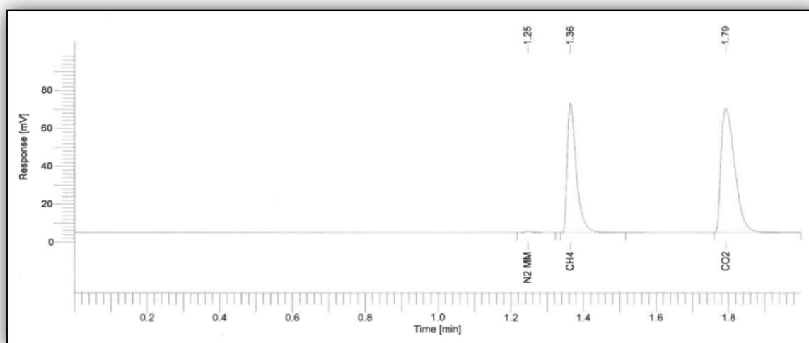
Figure 64 Response peaks from GC measurement for sample BG1.1-J1 (TOC = 11%). Note that the  $\text{CH}_4$  peak is having almost ideal peak-shape, while the non-organic presence of the  $\text{CO}_2$  response infers for broader peak with some disturbances.
