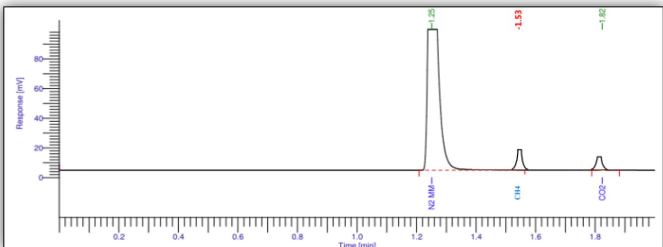
Figure 65 GC response for sample BG1-J1 treated with nitrogen and helium carrier gas. All of the peaks show asymmetrical to fronting tendencies. Quantity of dry gas (CH<sub>4</sub>) is in the vicinity of 3%.
