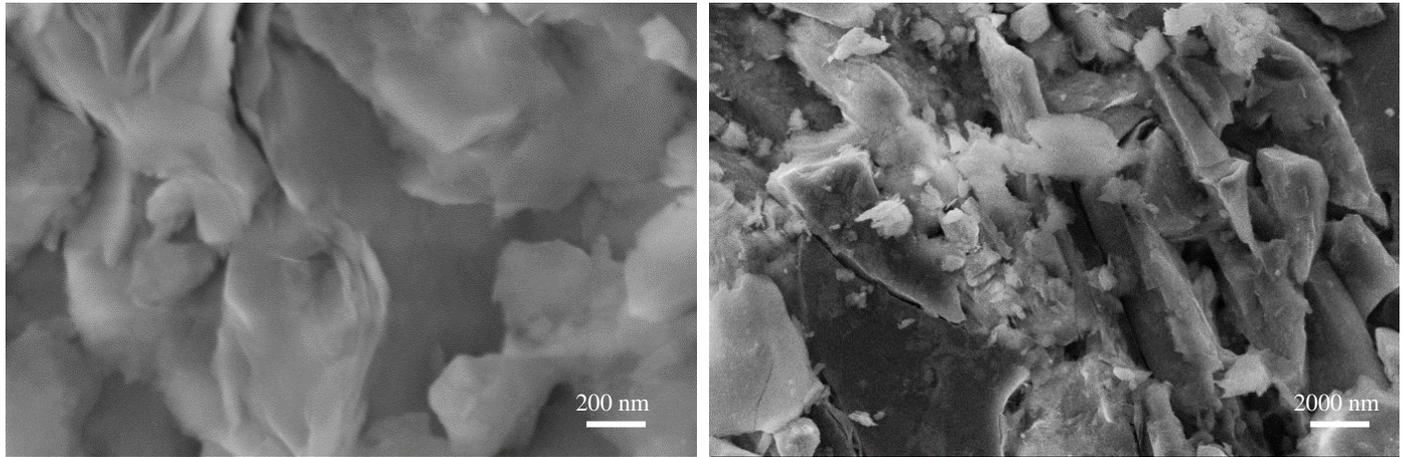
**Figure 20** Nanometer-sized pore throats in the unconventional shale/siltstone reservoirs of N Bulgaria (100 nm) indicating cleavage interpores in vitrinite (right) and intragranular moldic pores in clay crystals (60 nm) (left) (SEM own observation sample BG 1-J1)
