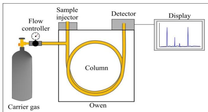
Figure 63 Schematic representation of a typical gas chromatograph's setup (Naturwissenschaften, D. Der. (2013))
