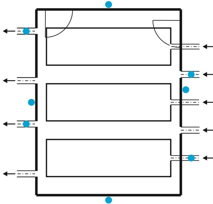
Figure B.1. Position of thermocouples outside test room.
