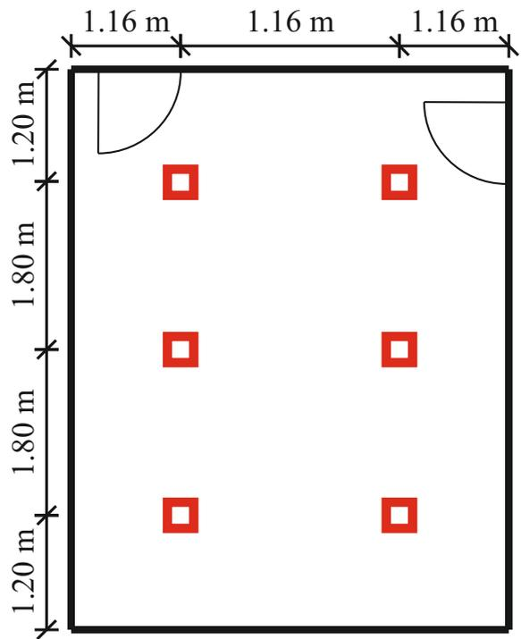
Figure B.4. Heat load distribution 3.
