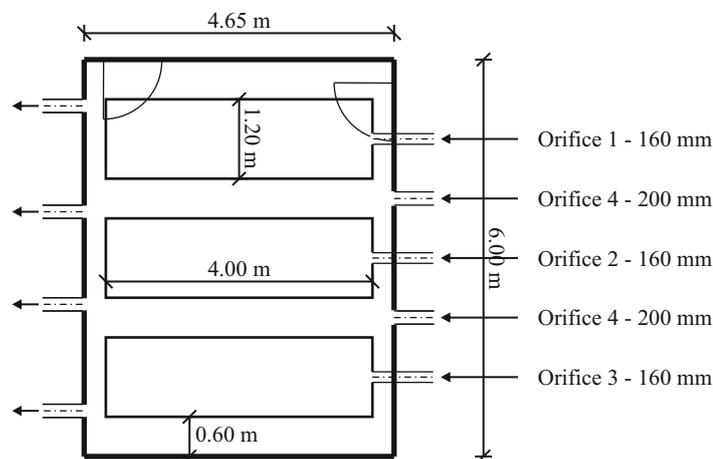
*Figure E.2.* Two different types of orifices used for measuring the supply flow rate.
