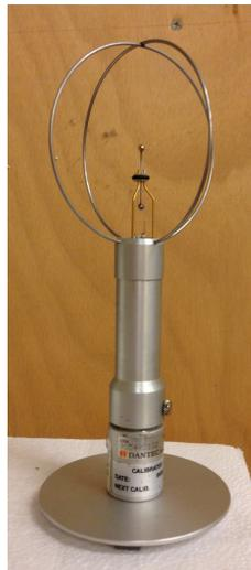
*Figure C.1.* Dantec hot-sphere anemometer.
