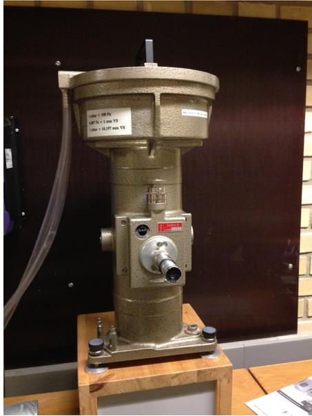
*Figure C.3.* Micro manometer.
