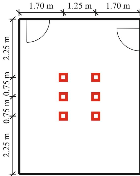
Figure B.2. Heat load distribution 1.
