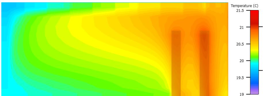
(b) Section, temperature, 64119 cells.
