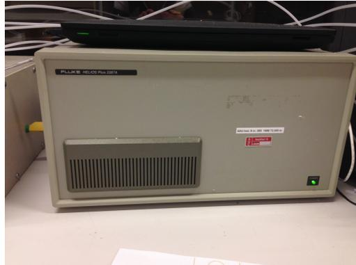
*Figure D.4.* Fluke Helios data logger.
