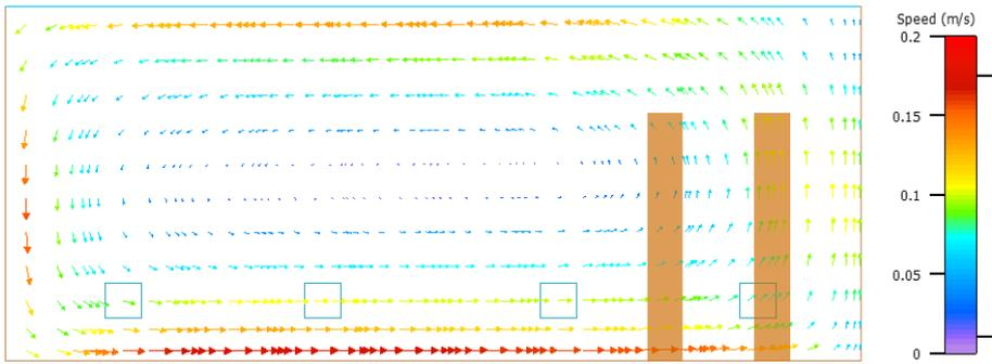
(a) Section, velocity, 35200 cells.
