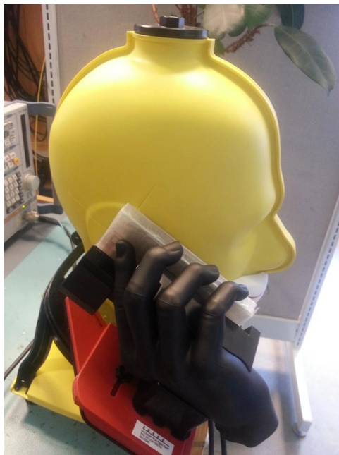
Figure 7.12: Grip of the EUT as per CTIA requirements.
