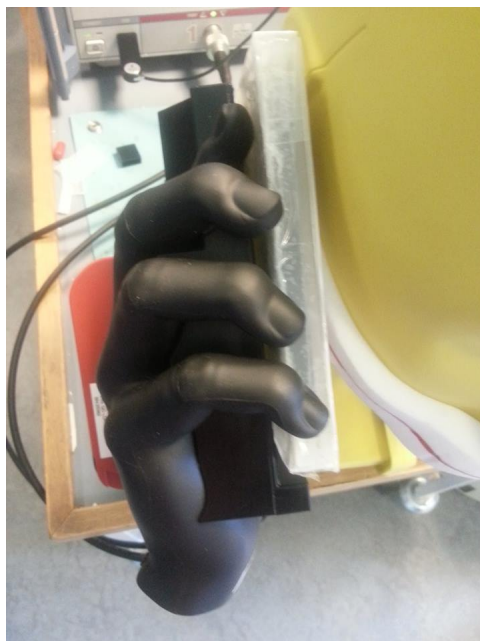
Figure 7.13: Grip of the EUT as per CTIA requirements.
