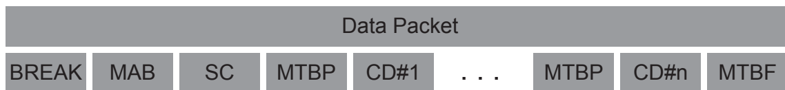
Figure 2.3: Structure of a DMX data packet. It is not mandatory to send all 512 channels so n can be chosen to be 1 < n \leq 512 [4, img. 5]
