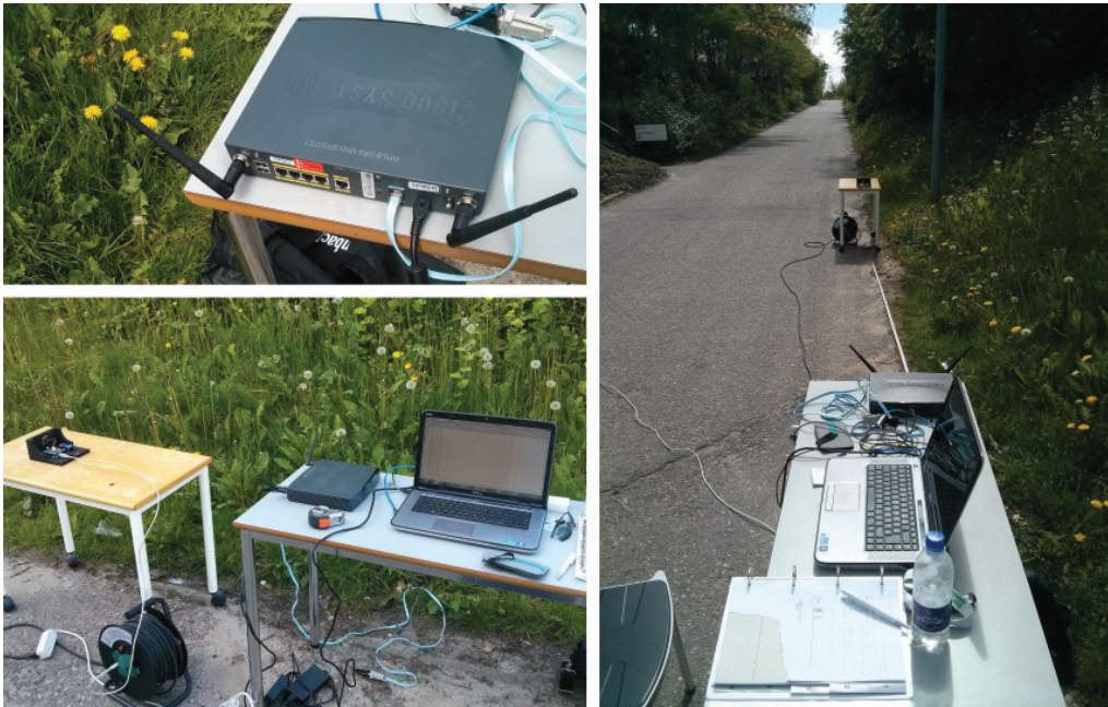
Figure 6.9: Images of the field test. Top: close-up of the antenna positions. Bottom: Measurement of packet loss in 1 m distance. Right: Location of the measurements. The receiver had been placed on different spots on the path, always on the right side to allow traffic to pass by.
