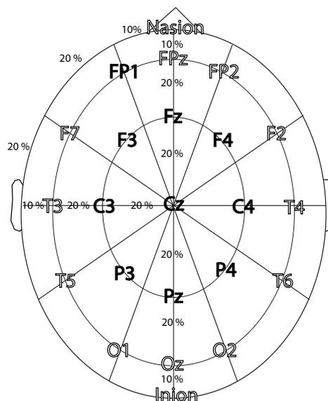
**Figure 6.1:** The location of the recording sites are marked in bold. The electrodes are placed according to the 10 20 EEG system.
