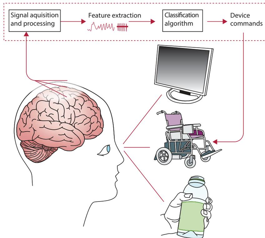
**Figure 2.1:** An illustration of a general BCI showing the three steps signal acquisition and preprocessing, feature extraction, and classification needed to produce device commands to different devices. The figure is adapted from Daly and Wolpaw [2008].
