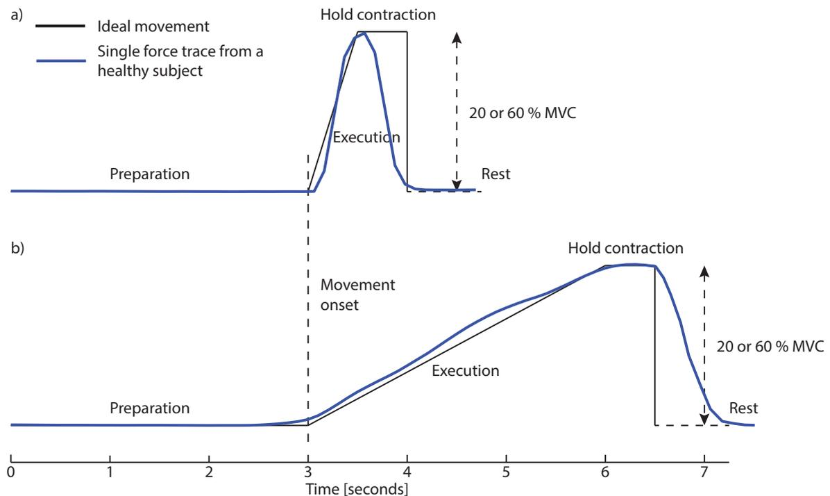
**Figure 7.1:** The two different kinds of movements performed in the experiment. a) a fast movement with a preparation phase of 3 s, an execution phase of 0.5 s, hold phase of 0.5 s, and a rest phase of 3.5 to 4.5 seconds b) a slow movement with a preparation phase of 3 s, a execution phase of 3 s, hold phase of 0.5 s, and a rest phase of 3.5 to 4.5 seconds Both movements are performed at 20% of MVC for the healthy subjects and at both 20 and 60 % MVC for the patients.
