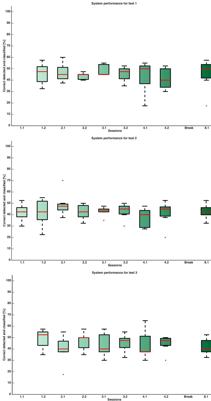
**Figure 11.1:** The boxplots are divided into 25 % and 75 % quartiles showing the median value in a red line and whiskers depicting the extreme datapoints not considering outliers shown by red dots. System performance for the three different tests. Session 1.1 for test one and three are not present since these were not recorded during the first session.
