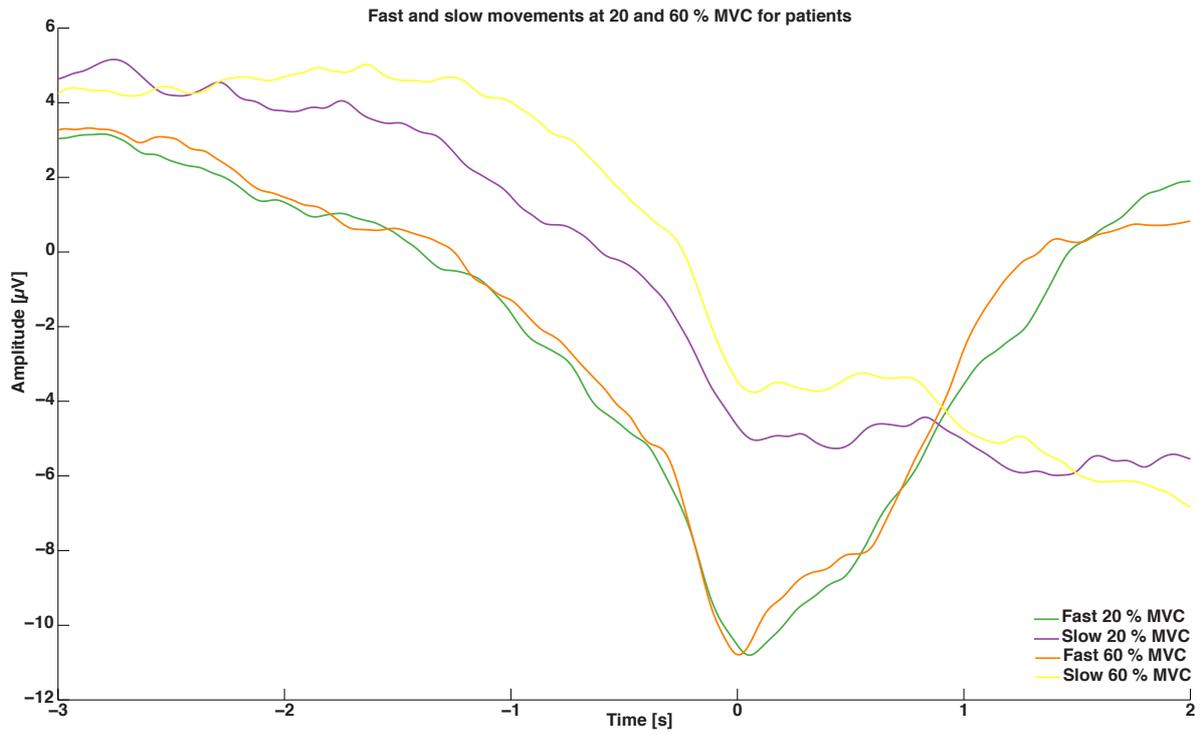
**Figure 12.4:** A grand average of the four different recordings performed for the patients fast and slow movements at 20 or 60 % MVC. The movement onset is at time (0). The figure is based on a total of 1154 MRCP sweeps.
