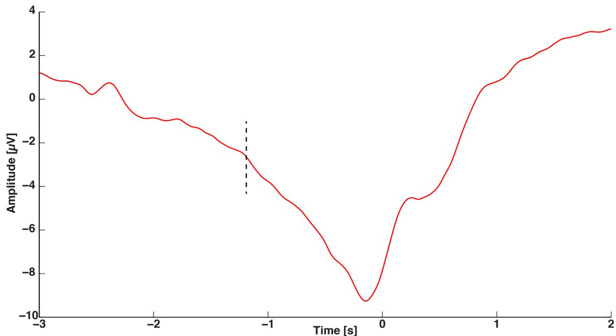
**Figure 3.1:** An example of a MRCP. The movement onset is at 0, the two phases before the peak of maximum negativity is shown by the dotted line and the movement-monitoring potential occurs after the peak of maximum negativity. The movement is an externally cued movement, it was initiated at time(-3) and the cue to move was given at time(0).
