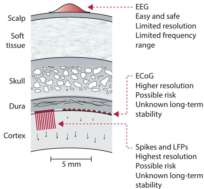
**Figure 2.2:** Location of three different EEG recording electrodes. The figure is from Daly and Wolpaw [2008]
