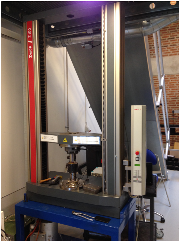
Figure A.6 The M12 transducer mounted in the tensile test machine
