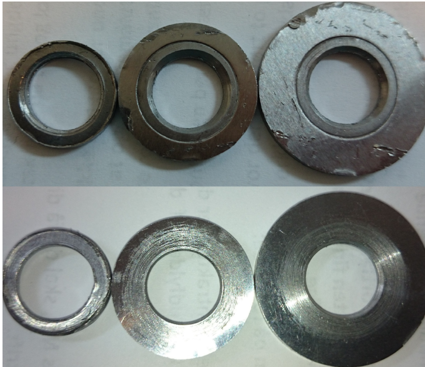
Figure 2.25 Indents and abrasions caused by bolt tightening
