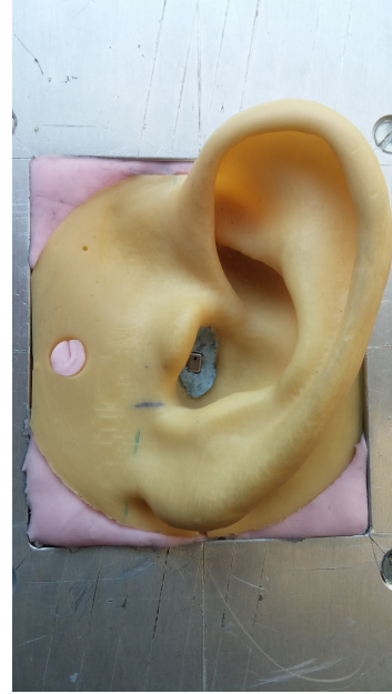
Figure A.6: Artificial ear with the microphone mounted for blocked entrance reference measurement.
