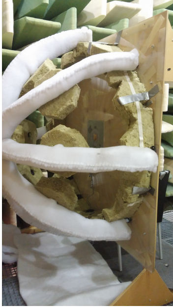
Figure A.5: The spider setup in an anechoic chamber.
