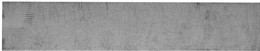
*Figure 5.11.* High contrast photograph of a plate showing surface scratches.
