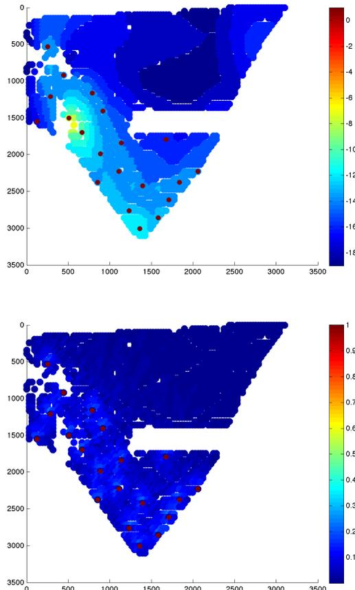
Figure 9.9: Solution with 20 turbines taking the costs of foundations into account. The first plot shows the turbine positions (red dot) in relation with water depth (colors in the background), while the second plot shows the interference between them.
