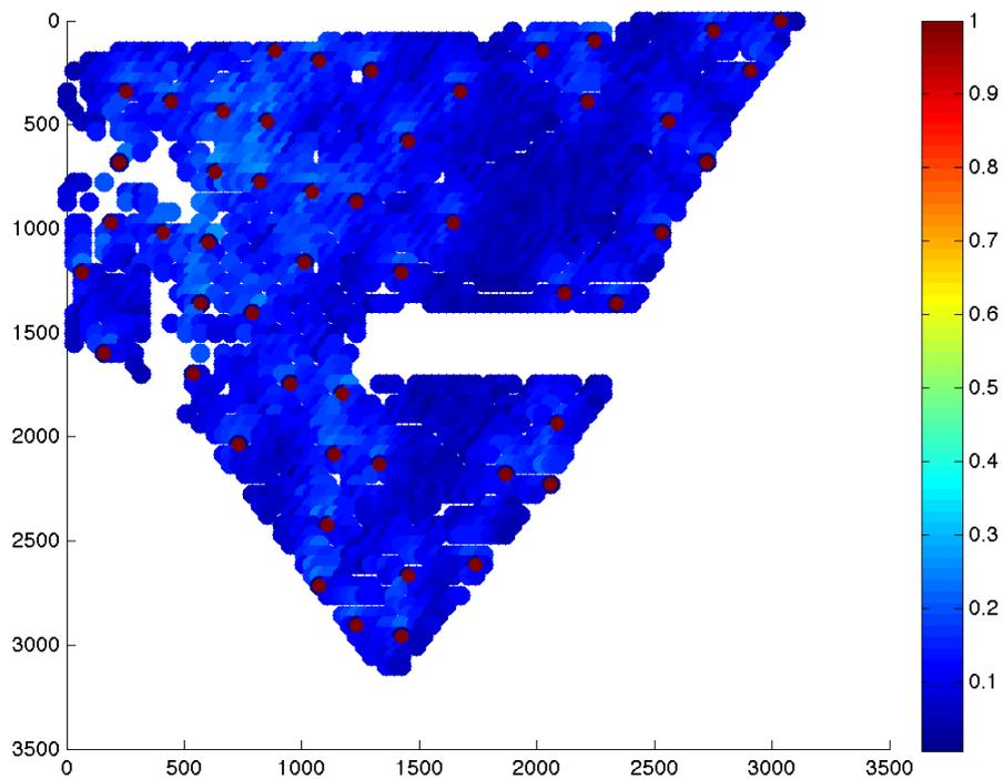
Figure 10.4: Solution with 50 turbines and  $D_{MIN}$  of 10 rotor diameters taking the costs of foundations into account. The plot shows the turbine positions (red dot) in relation with interference (colors in the background).
