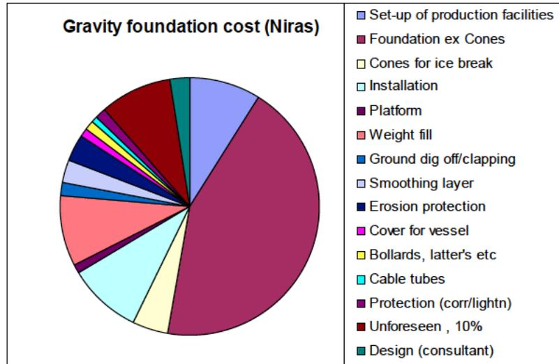
Figure 9.3: An example of how different factors influenced the price of a Gravity foundation on 8m water [21]
