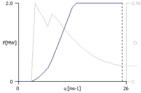
Figure 3.3: Wind Speed vs  $C_t$  (gray line) and Wind Speed vs Power (blu line) [10]
