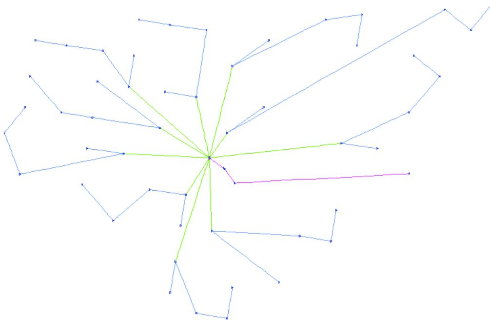
Figure 10.6: Output of our cable optimization tool. The magenta cable represents the export cable (not part of the optimization) that cannot be crossed by the inter-array cables.
