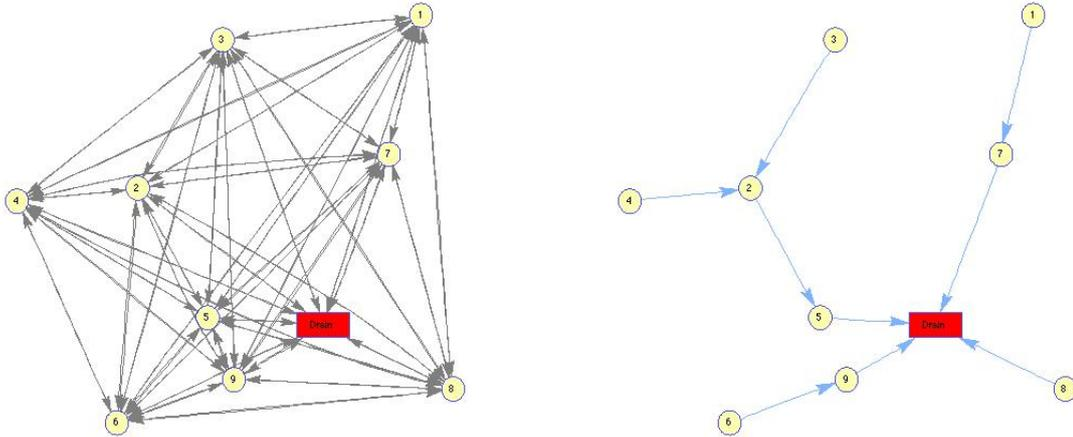
Figure 8.2: Example of cable layout problem for 9 turbines and 1 substation. The model considers all the possible connections between nodes, so the variables of the model will refer to the complete graph in the first plot. Only some arcs will be selected in the final solution tree (second plot).
