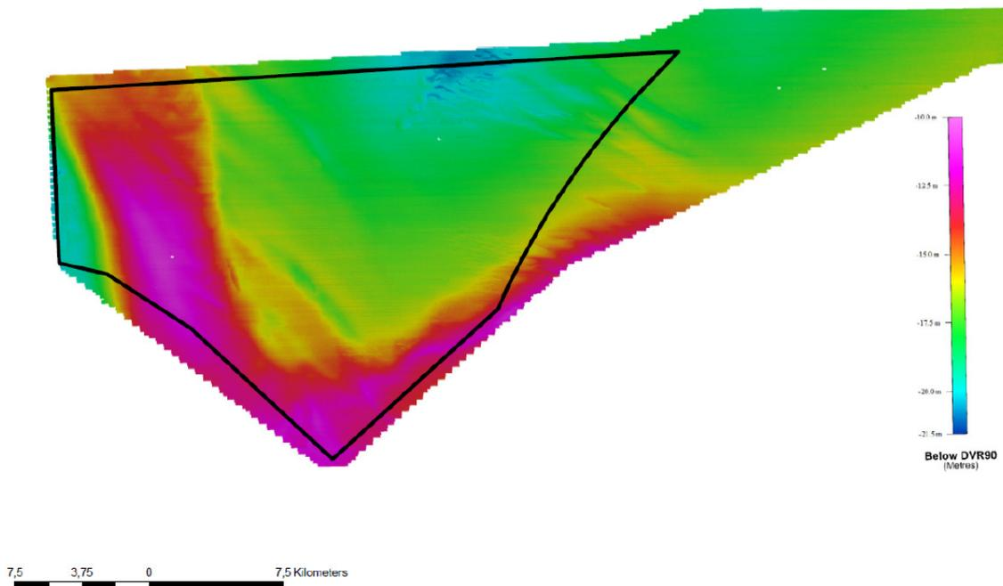
Figure 9.5: Bathymetric map of Horns rev 3 based upon the Geophysical survey in 2012 [22]
