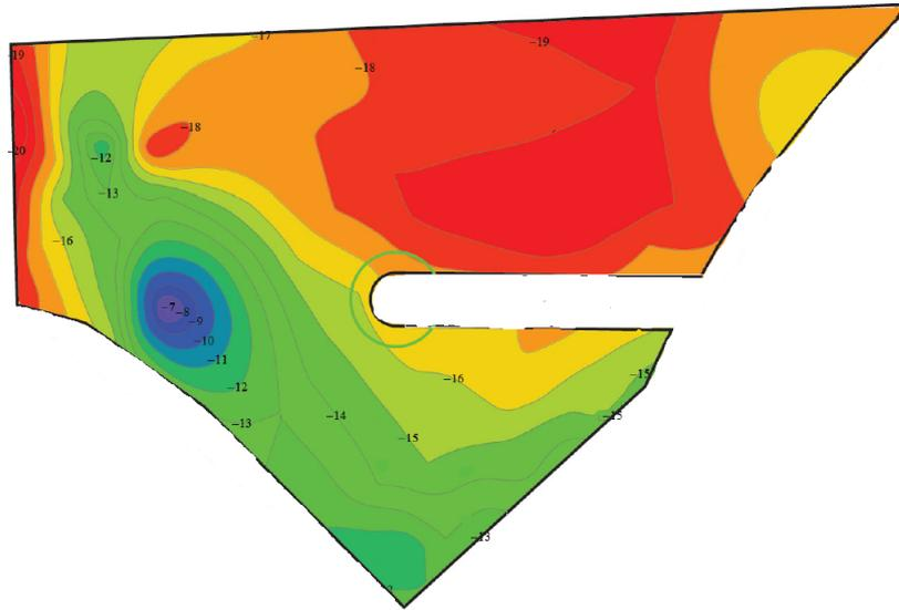
Figure 9.6: Horns Rev 3 available area for the offshore wind park. Colors refer to water depth.
