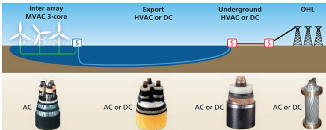
Figure 1.6: Different types of cable connection exist: the inter-array one is used to collect the energy from offshore turbines, while the export cable transfers this energy to the coast and underground and overhead line (OHL) cables make it all work on land. Credit: Nexans
