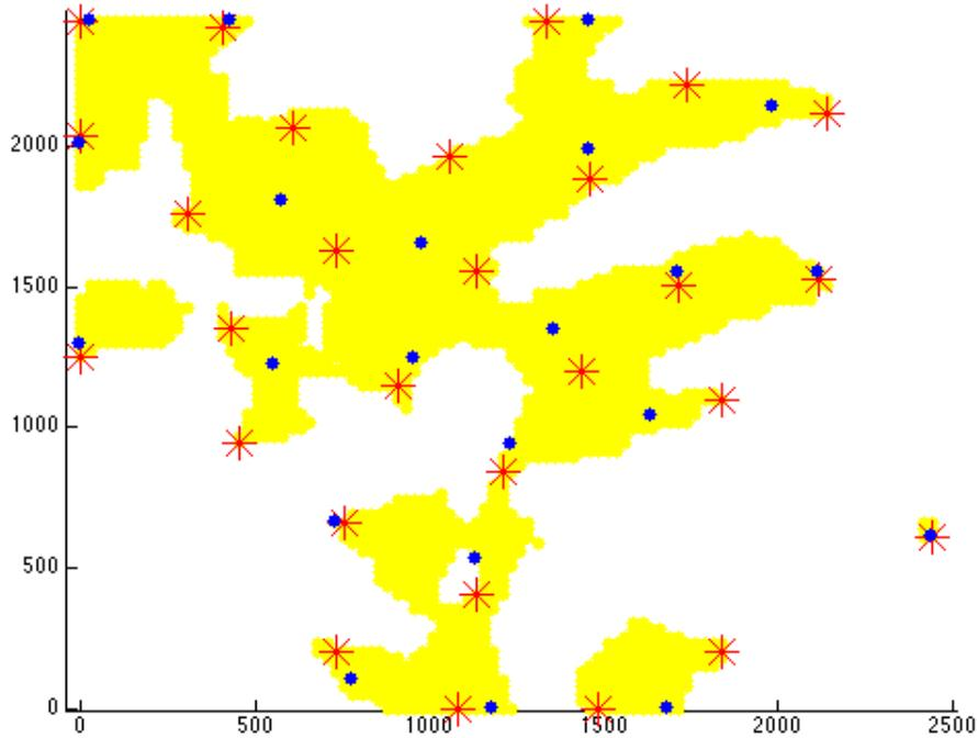
Figure 7.2: Optimized layouts in case of unlimited maximum number of turbines. The yellow area represents the feasible area, the blue dots represent the layout found by *WindPRO's Optimize*, while the red stars are the layouts computed by our tool. *WindPRO's Optimize* is able to locate only 22 turbines vs 28 of our tool.
