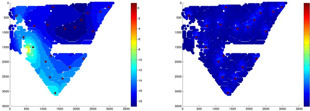
Figure 9.8: Solution with 20 turbines not taking the costs of foundations into account. The first plot shows the turbine positions (red dot) in relation with water depth (colors in the background), while the second plot shows the interference between them.
