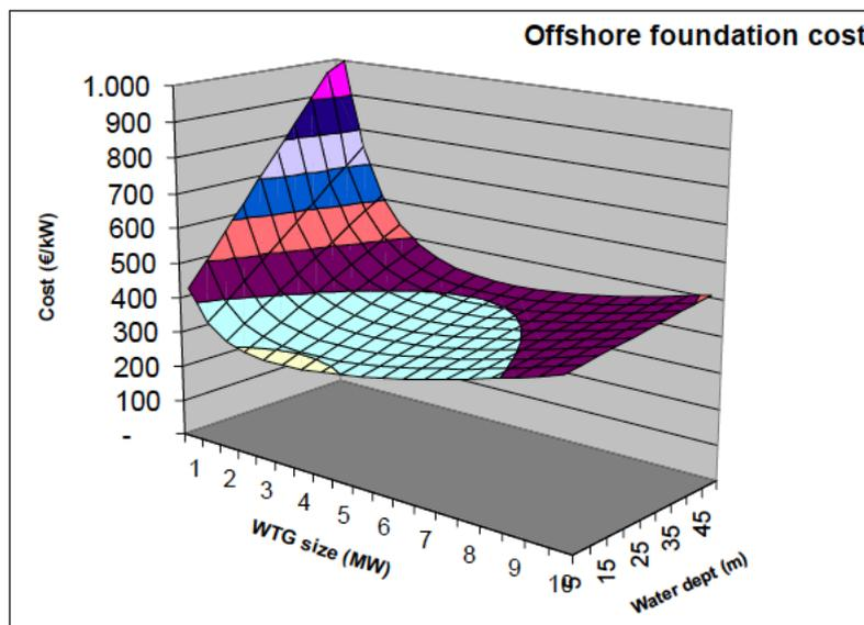
Figure 9.2: Foundation cost depending on water depth and type of turbine [21]
