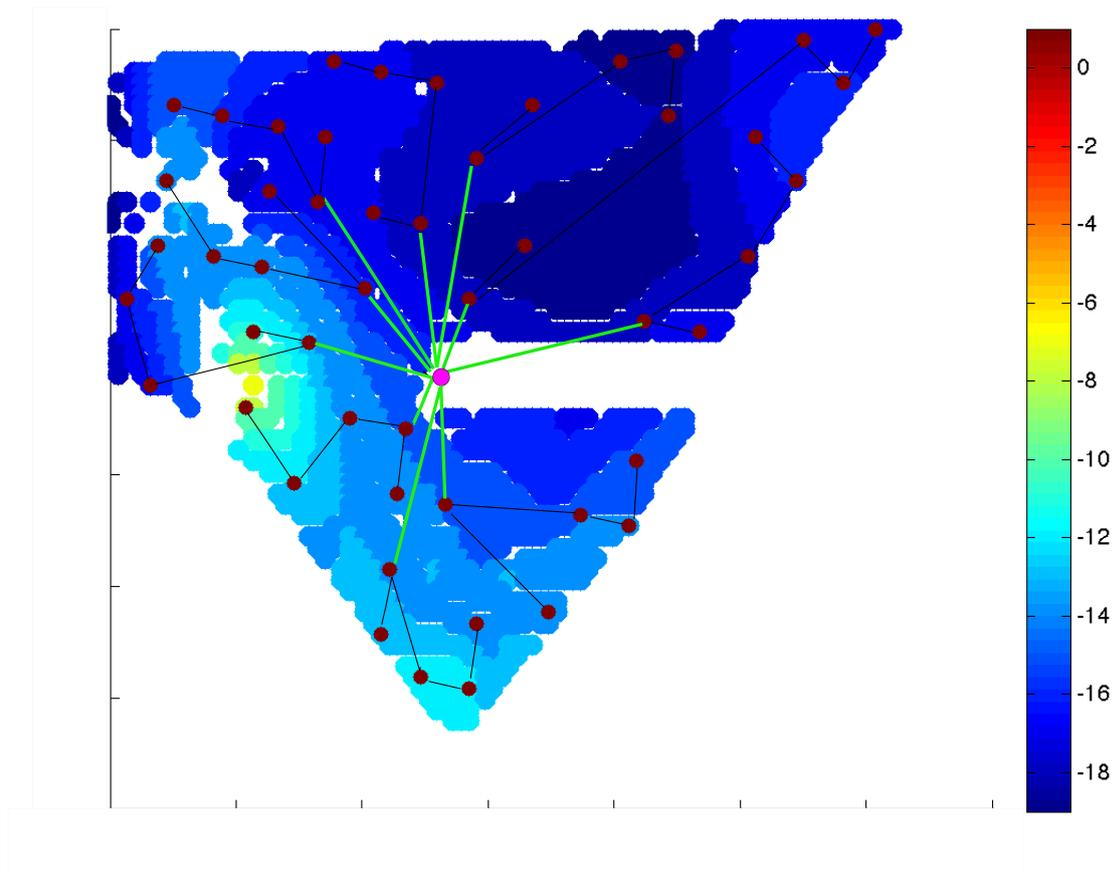
Figure 10.7: Final output of our two tools together: the turbines positions are optimized according to wind resources and foundation costs, while cable connection is optimized according to cable costs, cable capacity and type of substation (number of connection). Cable crosses are not allowed and the export corridor cannot be crossed by cables as well.
