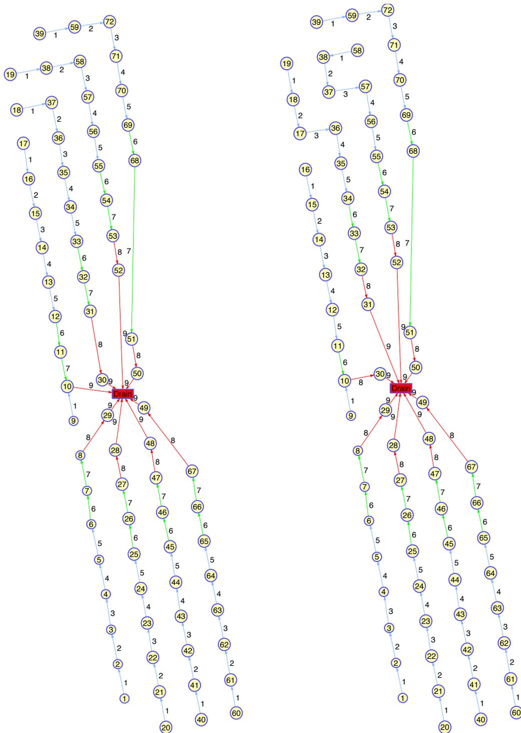
(a) Our layout with installation costs (39 640 235 €) (b) Our layout found with only one type of cable and re-evaluated (39 683 551 €)
