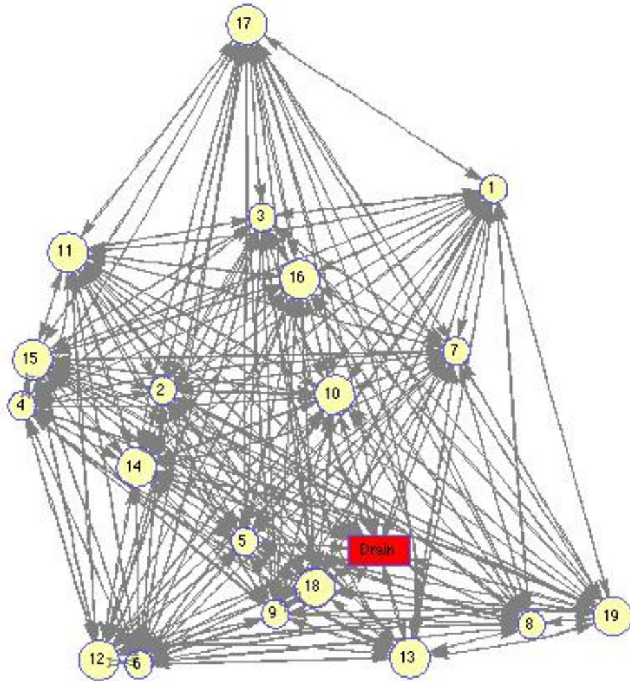
Figure 8.4: The graph with all the possible connections that the optimizer is using for a toy example of 19 turbines and 1 substation. The number of crossings that should be explicitly forbidden is huge.
