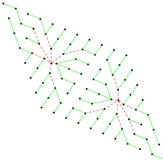
Figure 8.1: Example of a cable grid problem in an offshore site with two substations. [18]
