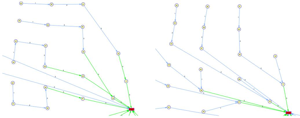
Figure 8.11: Part of the optimized layout of data set 1. The first plot refers to the layout found manually and the second plot is our optimized layout. The blue cables are the less expensive. Part of the solution is not displayed due to confidentiality issues.
