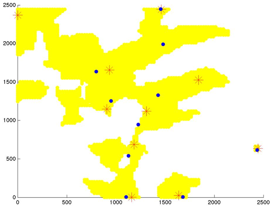
Figure 7.3: Compared layouts in case of maximum number of turbines equal to 5 and 10. The yellow area represents the feasible region, the blue dots represent the layout found by *WindPRO's Optimize*, while the red stars are the layouts computed by our tool.
