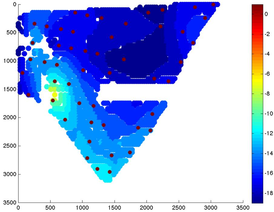
Figure 10.3: Solution with 50 turbines and  $D_{MIN}$  of 10 rotor diameters taking the costs of foundations into account. The plot shows the turbine positions (red dot) in relation with water depth (colors in the background).
