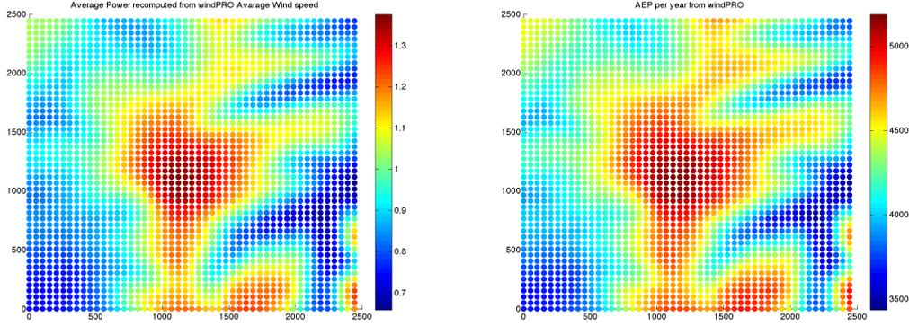
Figure 7.1: Power distribution within the site: left plot is the average power production in MW we computed from the average wind speed given by *WindPRO*, the right one is the annual energy production in MWh/y computed by *WindPRO*.
