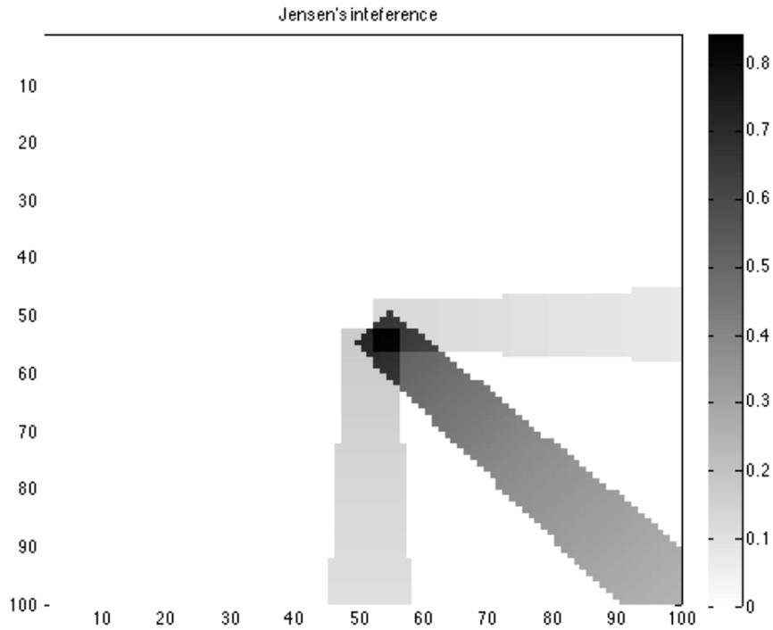
Figure 3.8: An example of  $I_{i,j}$  computed as the average interference between three possible wind scenarios: wind = 7.0 m/s from north with probability 0.3, wind = 8.0 m/s from north-west with probability 0.6, wind = 9.0 m/s from west with probability 0.1 ; pixel = 10x10m;
