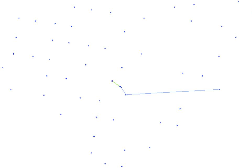
Figure 10.5: Input for the cable optimization. The disconnected turbines are the real turbines found by our layout optimization tool (the ones in Figure 10.3) that we want to connect with an optimal cable routing. A fixed path between fake turbines is added to avoid the tool to pass through the export corridor.
