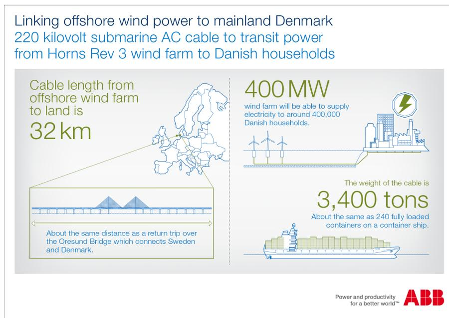
Figure 10.1: Figures related with Horns Rev 3 connection to the coast [ABB infographic Denmark cable link]
