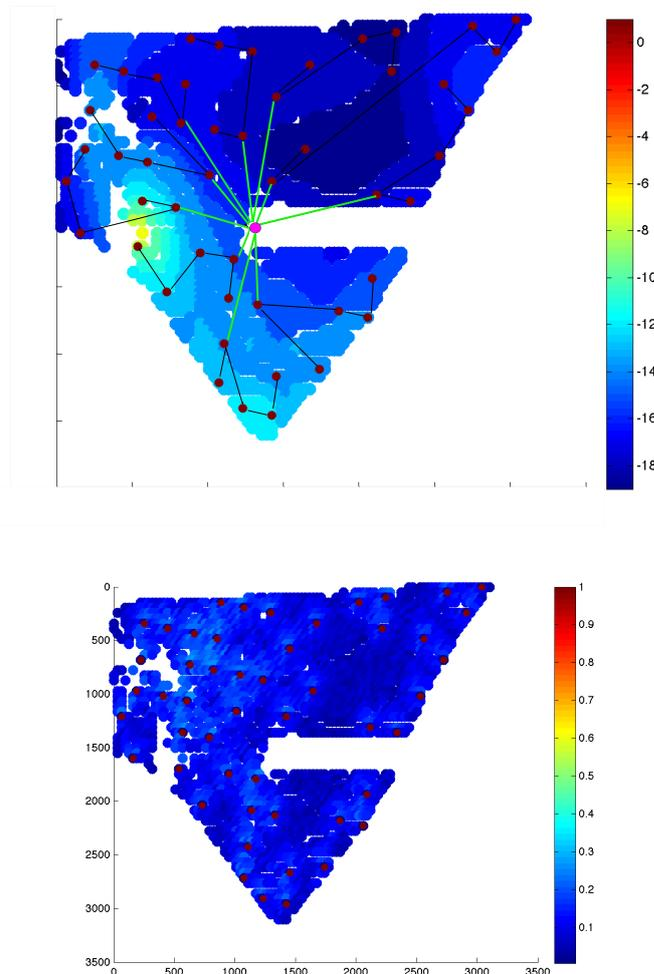
Figure 1.8: Final output of our two tools together for a real-world offshore site: the turbines positions are optimized according to wind resources and foundation costs, while cable connection is optimized according to cable costs, cable capacity and fixed number of connection to the substation. Cable crosses are not allowed and the export corridor cannot be crossed by cables as well. In this optimization the number of turbines to build is fixed (50 turbines).
