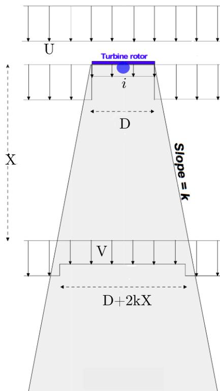
Figure 3.1: Wake effect according to Jensen's model with wind from north to south
