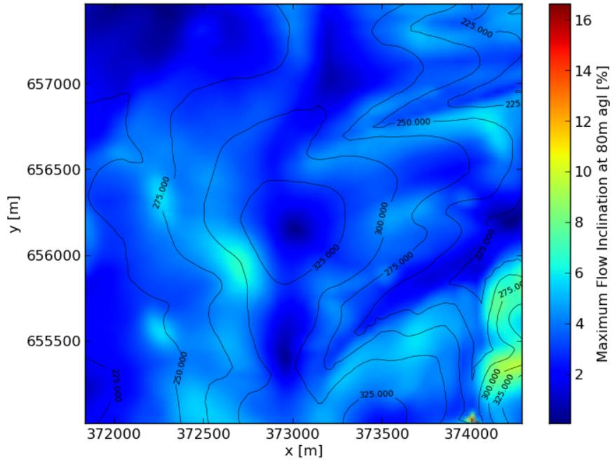
Figure 2.6: Maximum Flow Inclination [m/s] at 80m agl for our test site
