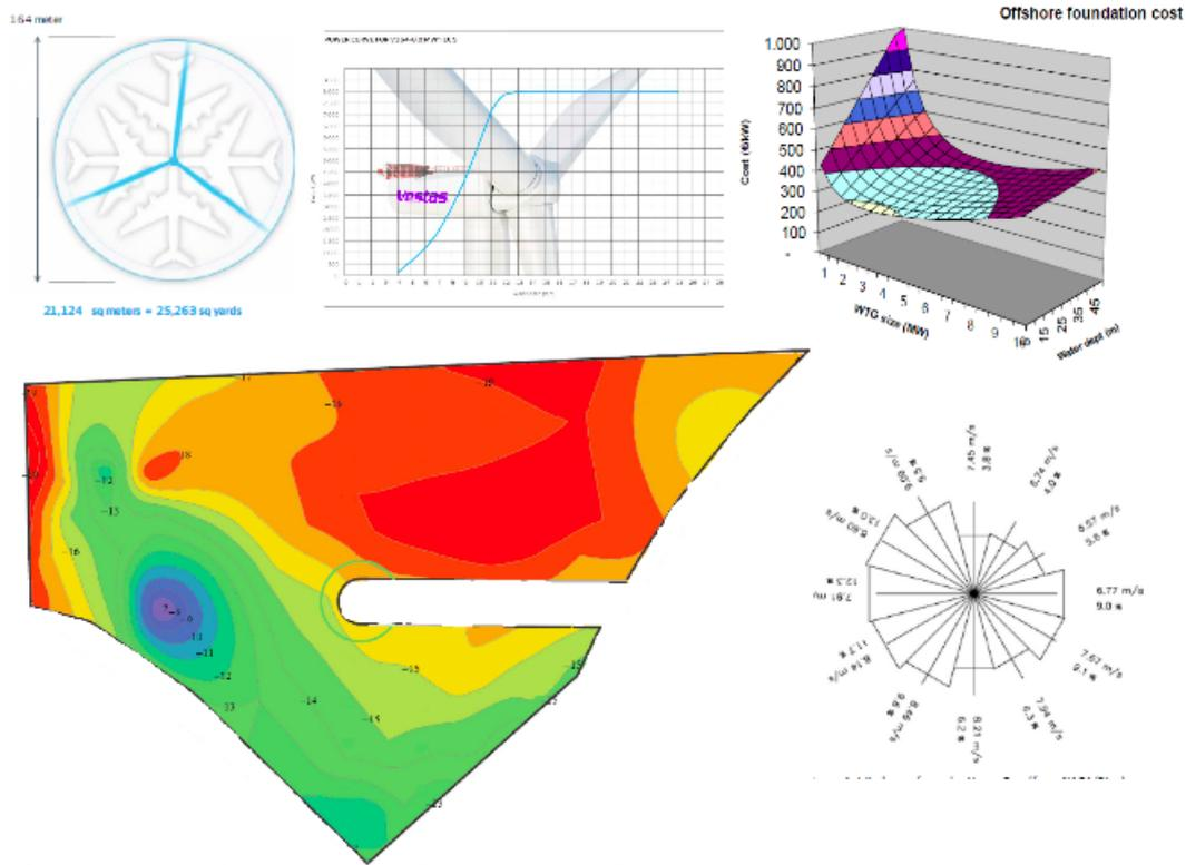
Figure 10.2: Input to the layout optimizer: the characteristic of the turbines V164 (rotor dimension,  $C_p$ ), costs of foundations, the site area with its water depth and wind speed measurements of Horns Rev 1.
