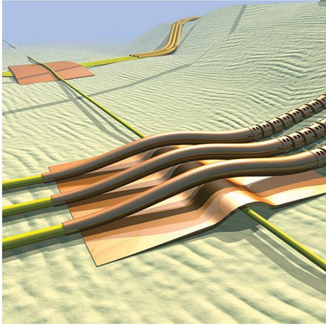
Figure 8.3: Example of cable crossings in an off-shore case
