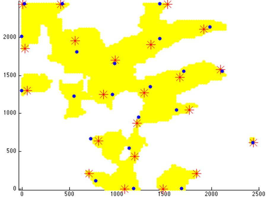
Figure 7.5: Compared layouts in case of maximum number of turbines equal to 22. The yellow area represents the feasible region, the blue dots represent the layout found by *WindPRO's Optimize*, while the red stars are the layouts computed by our tool.
