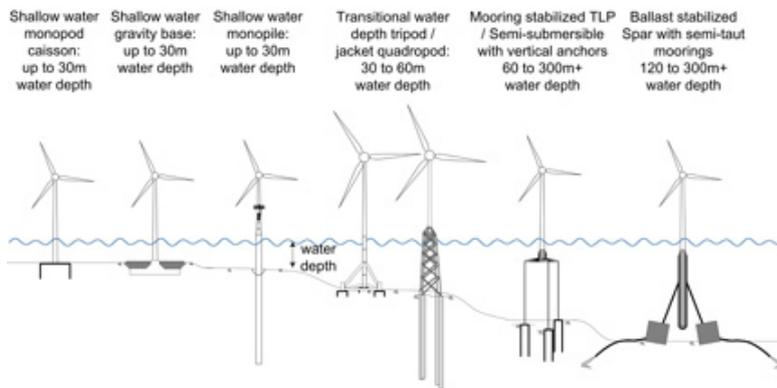
Figure 9.1: Different type of foundations. Figure credit: J. Schneider after NREL.
