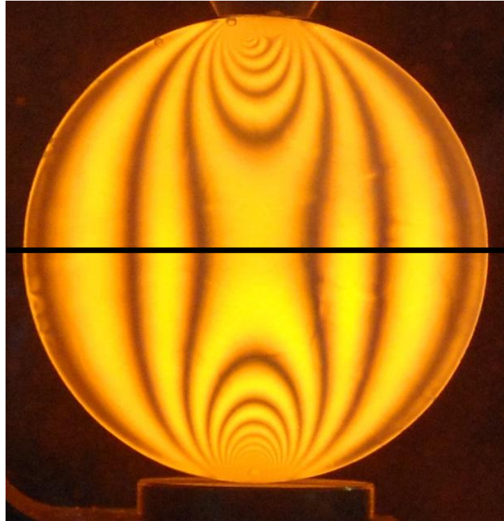
Figure C.3 Fringes in the disc, when a load of 1000 N is applied. The black line mark the horizontal centreline at which the fringes are evaluated.
