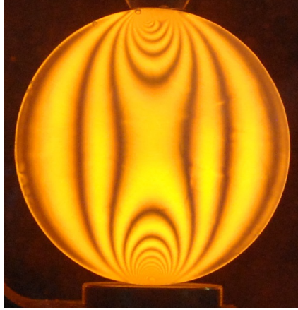
Figure 4.5 Example of fringe pattern in a stressed test specimen.
