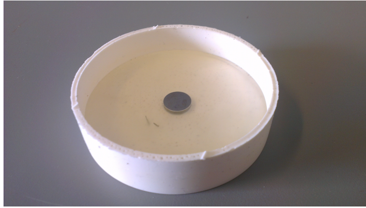
Figure 2.2 Test specimen with steel insert in a silicone mould.
