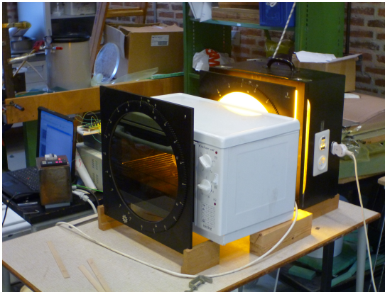
Figure 4.1 Image of the set-up, with an oven between the filters of the polariscope
