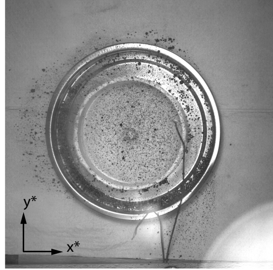
Figure 3.6 Image from right camera of DIC system
