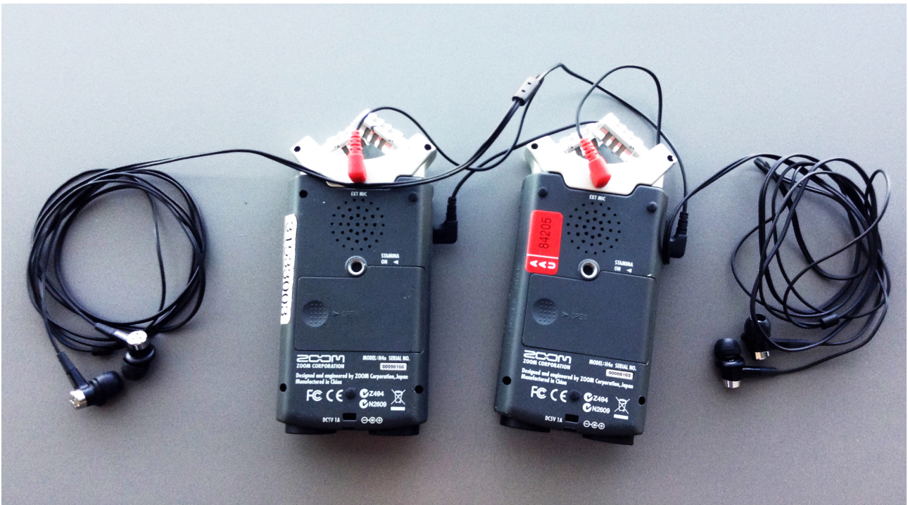
Figure 14: Binaural microphones are cross-connected to Zoom H4n Recorders
