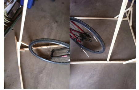
Bicycle clearance when maneuvering a bicycle through pod-car doorway.
