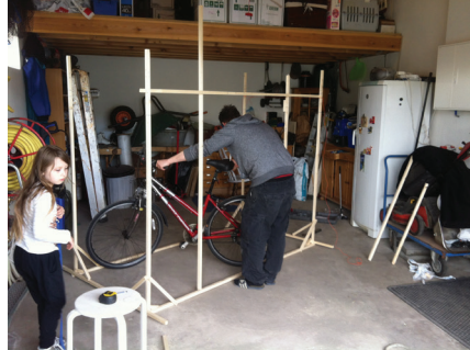
Maneuvering a bicycle into the pod-car and testing needed doorway width.
