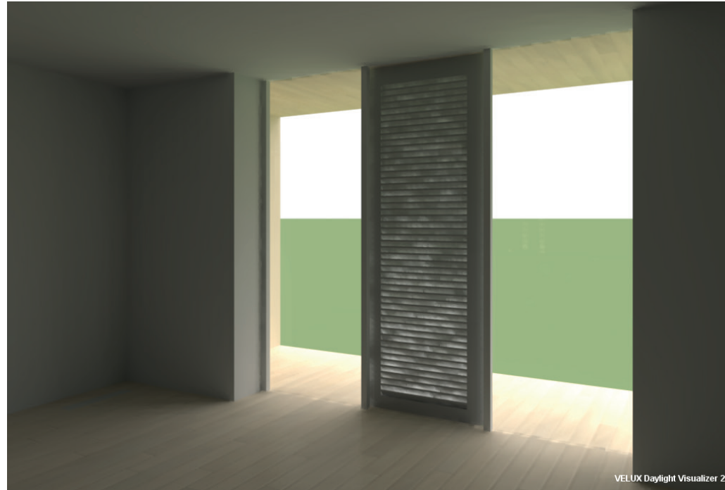
Ill. 104: Final proposal for solarshading
