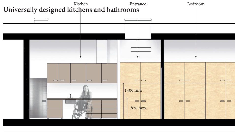
Ill. 147: Section in 1:75 showing kitchens and storage in the apartments
