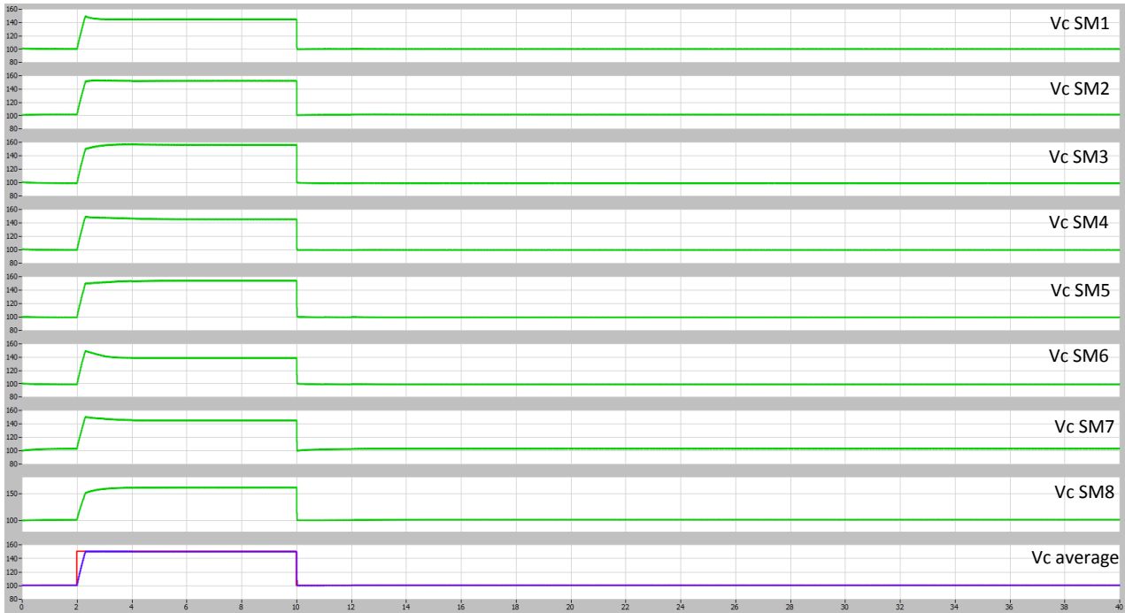
Figure 64. . Simulated capacitor voltage with averaging and balancing control and a step voltage reference.
