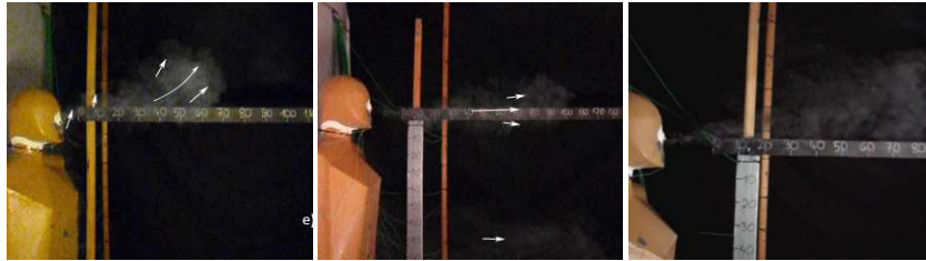
Figure 2.2 Exhalation jet in case of breathing through the mouth for a)no ventilation b)displacement ventilation and c)mixing ventilation [11]
