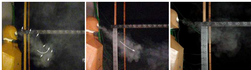
Figure 2.3 Exhalation jet in case of breathing through the nose for a) no ventilation b) displacement ventilation and c)mixing ventilation [11]
