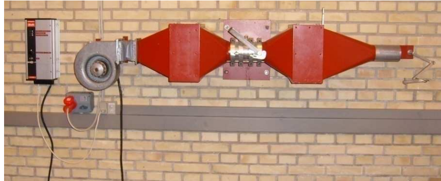
Figure A.2.4. Wind tunnel
