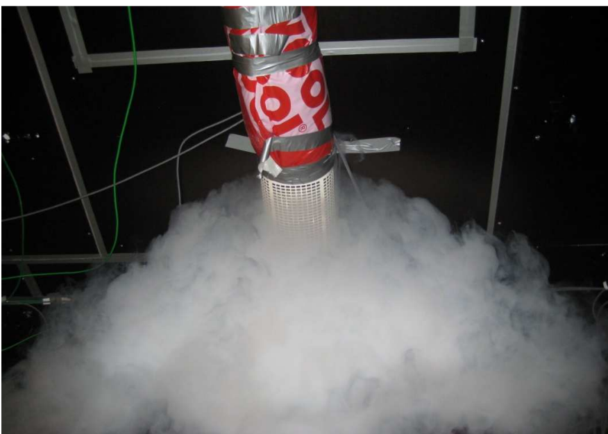
Figure 3.3 A smoke visualization of the air coming out of the diffuser.
