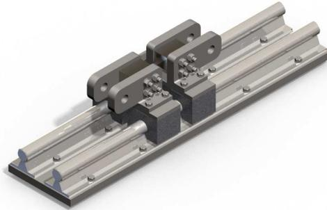
**Figure 3.2:** The slide through which the load and test-cylinder is connected.
