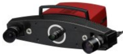
Figur B.4: Atos 3D hvidlysscanner [GOM, 2009]
