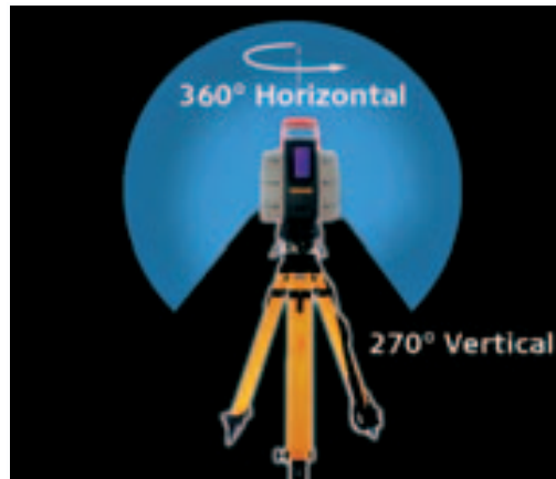
Figur B.5: Synsfeltet for en Leica Scan Station 2 laserscanner [Leica, 2009]
