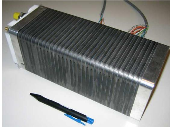
Figure 1.7: Picture of a HTPEM fuel cell
