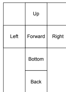
Figure C.3: Vertical cross cube map with annotations of the directions. The forward square is an image of the scene when the camera is directed along the negative z-direction, etc.
