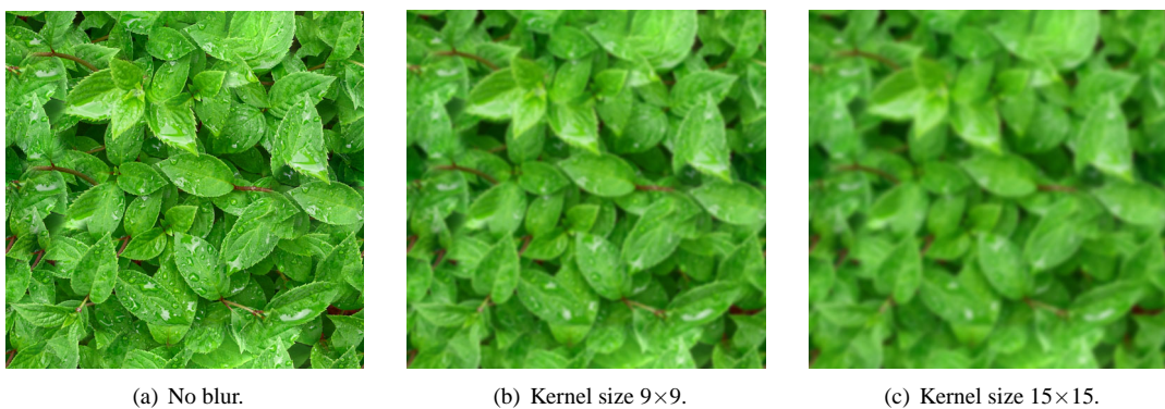
Figure 4.10: The effect of changing the kernel size on the used texture.
