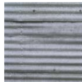
CORRUGATED STEEL: Proposed as the light roof construction over the buffer zone as a reflective material for solar radiation.
