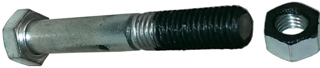
Figure 2. Shows a bolt and nut that is lubricated with Molykote 1000.
