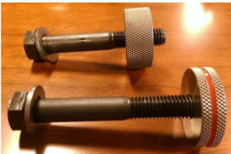
Figure 17. Shows two bolts being tested for thread tolerances with a go/no go test.
