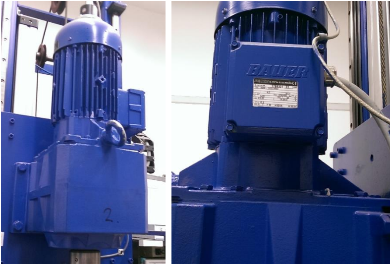
Figure 13. Bauer BG50 4kW helical geared motor.1. seen from the front. 2. Seen from the side.
