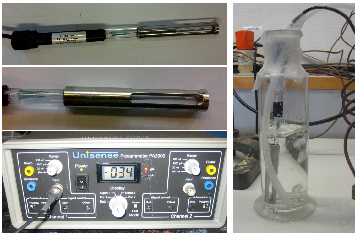
Figure 36: Pictures of the Unisense hydrogen sensor with the protection cap, the used pico ampere meter, and the set-up for calibrating the sensor in hydrogen saturated salt water.
