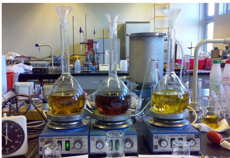
Figure 50: The experimental set-up in the investigation of chemical bleaching of RNO. To the left: Solution 2, in the middle: Solution 1, to the right: Blank (test 14).
