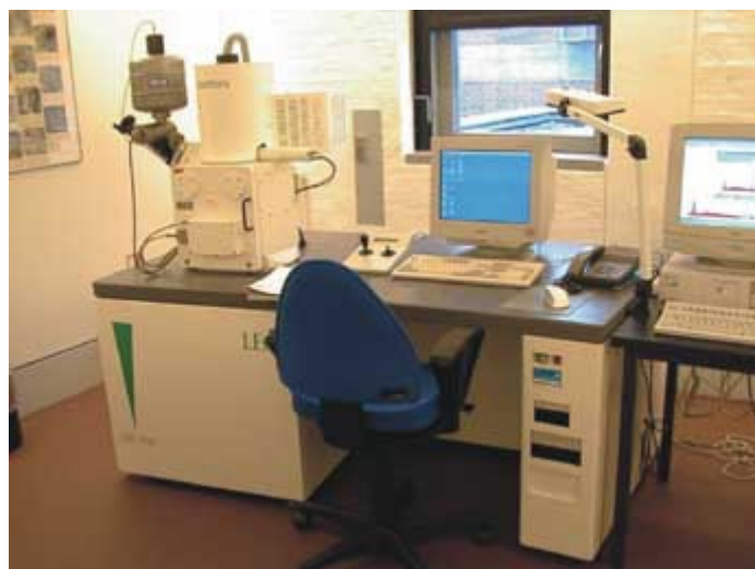
Figure 60: The used scanning electron Microscope at Aalborg University.
