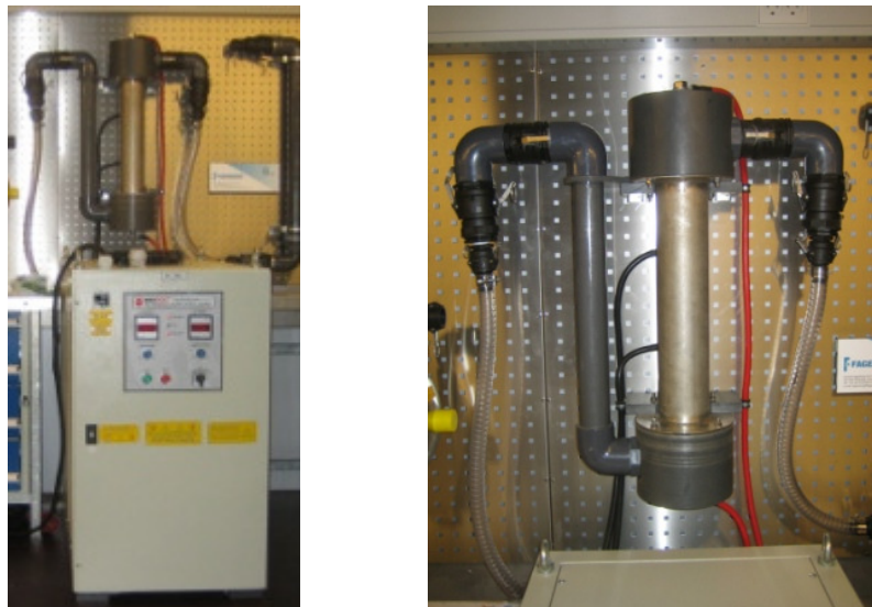
Figure 12: The electrochemical water treatment system consisting of reactor and power unit.
