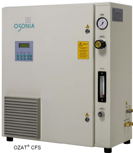
Figure 10: OZAT CFS-2G ozone generator from Ozonia and the installation in the test trailer.
