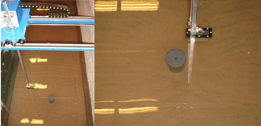
[Figure A.3](#) Illustration of the EP, profiling a back filled scour hole
