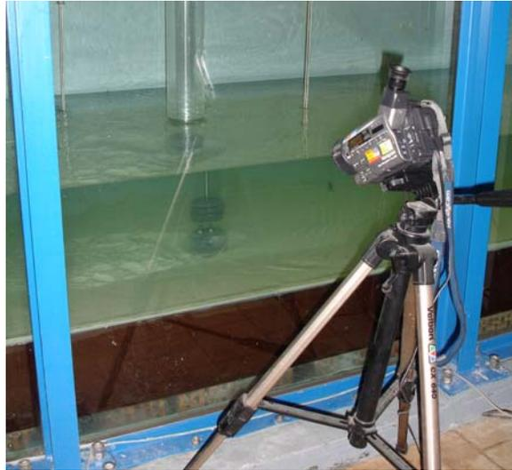
[Figure A.5](#) Video recording of the Clear water scour test
