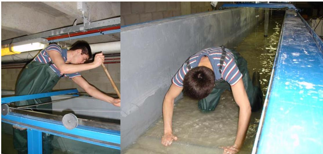
[Figure A.4](#) Working on the re-establishment of the bed, between tests
