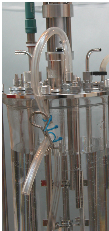
Figure 7.5: Original sampling valve mounted on the recurrent loop – Picture courtesy of Ph.D. Student Carina J. LOMBORG
