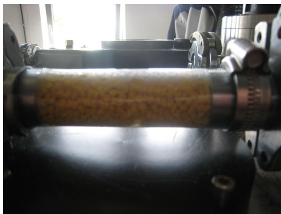
Figure 15.2: Clogging concentration: 15% of dry matter.
