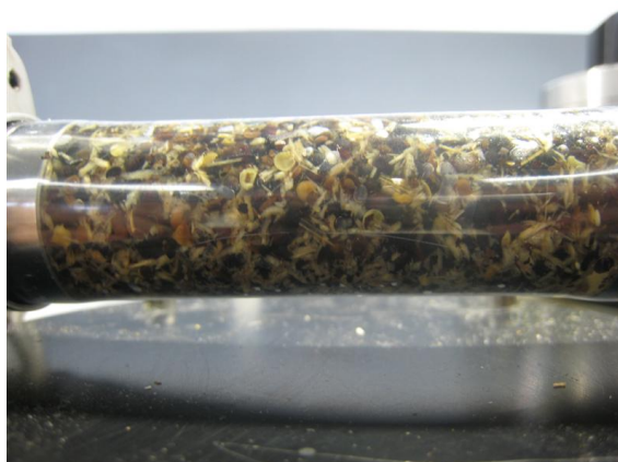
Figure 15.5: Clogging concentration: 7.5% of dry matter.
