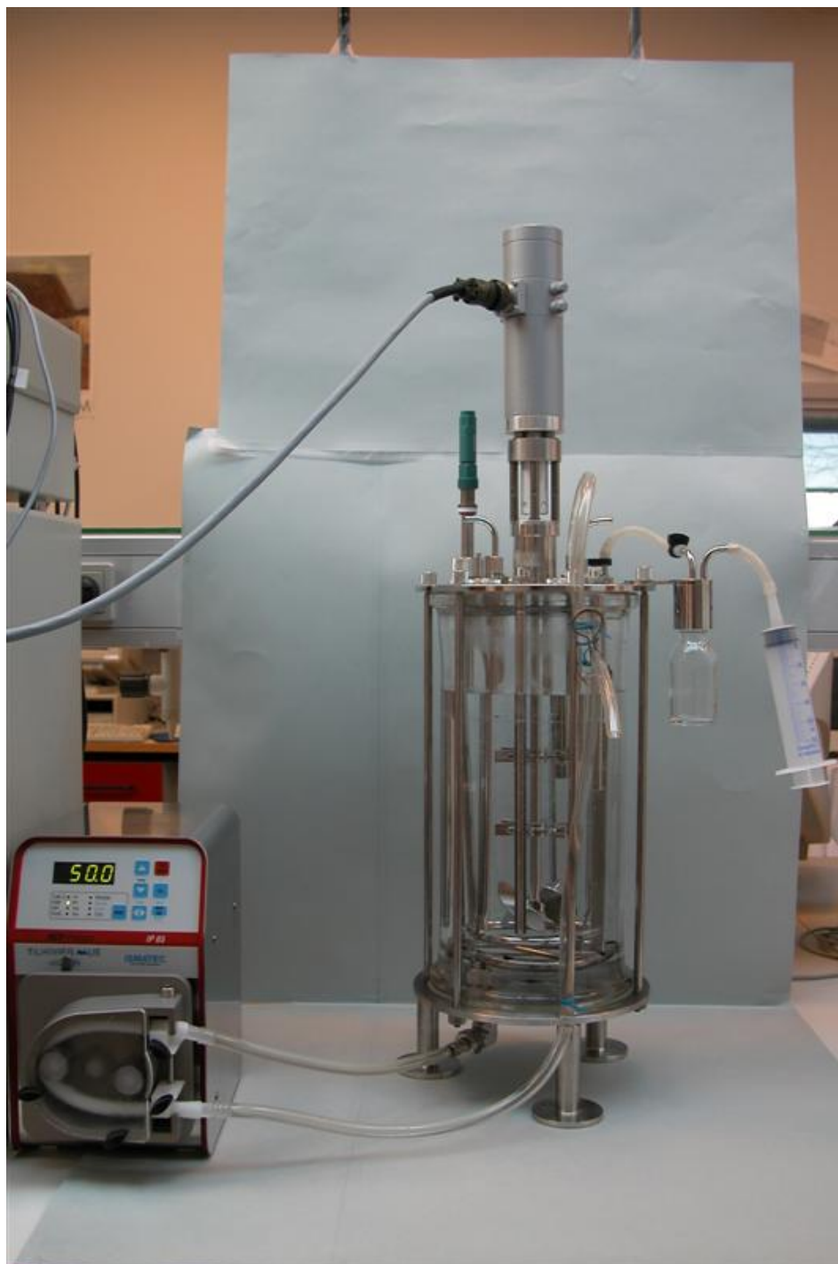
Figure 7.1: Laboratory scale reactor equipped with the original adaptation of the ACABS' sampling loop and the Applikon® standard sampling device – Picture courtesy of Ph.D. Student Carina J. LOMBORG
