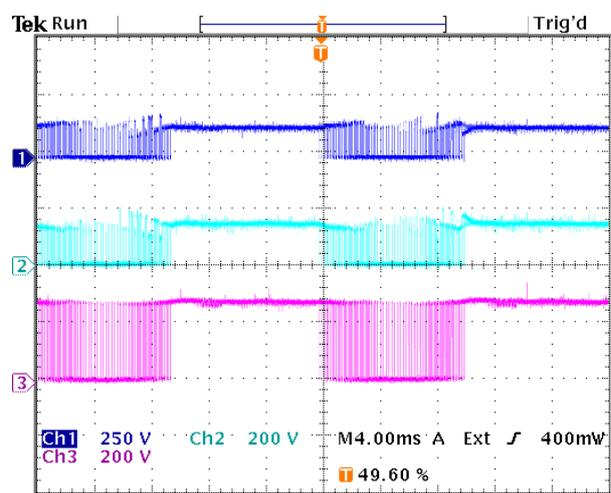
Figure 9.10: Voltage sharing of switch pair  $S_{b4}$ . Dark blue =  $v_{S_{b41}}$ , light blue =  $v_{S_{b42}}$ , purple =  $v_{S_{b4}}$ .
