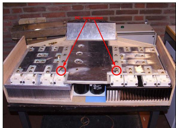
**Figure 8.9:** Layer three: Negative supply plate DC-.
