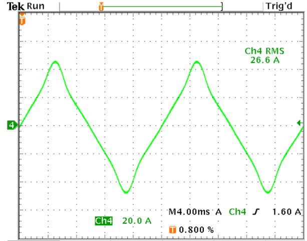
**Figure 7.6:** Measured current for one inductor. Notice the saturation at the top of the sinusoidal curve, causing the current to rise.
