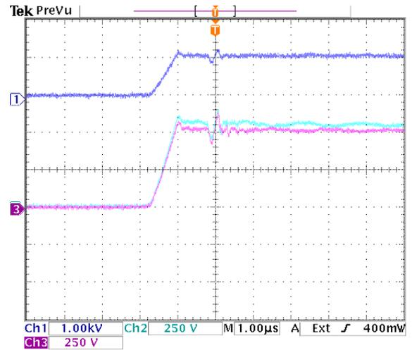
**Figure 9.40:** Zoom of turn off transition of diode pair  $D_{a2}$ . Dark blue =  $v_{Da2}$ , light blue =  $v_{Da21}$ , purple =  $v_{Da22}$ .
