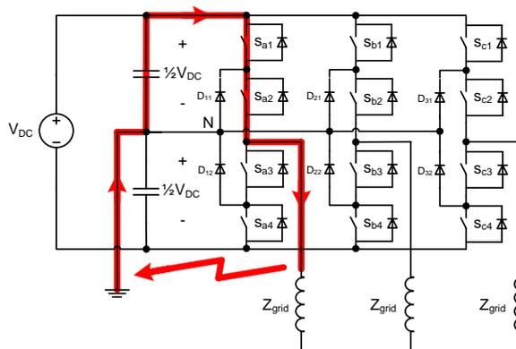
**Figure B.5:** Fast fault with phase to ground short circuit. Characterized by fast current rise, but only involving half of the DC link voltage.
