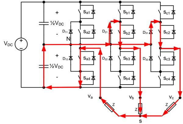
**Figure 2.16:** Current flow for state  $(0, +, +)$ . Notice that the current is leaving the neutral point, hence discharging the bottom capacitor.
