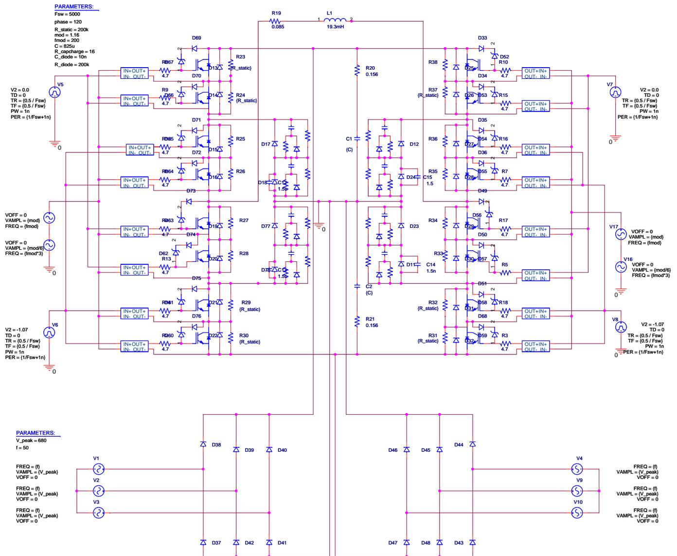
**Figure 8.1:** OrCad simulation of three-level inverter. Voltage imbalance for IGBTs obtained by adding a delay to one of the IGBT's in each pair like in section 4.2.9. Parameter deviation for diodes is implemented by parallel capacitors like in section 4.2.2. The reason for the extra diode across each IGBT is, that the anti parallel diode is not included in the Pspice model of the IGBT.
