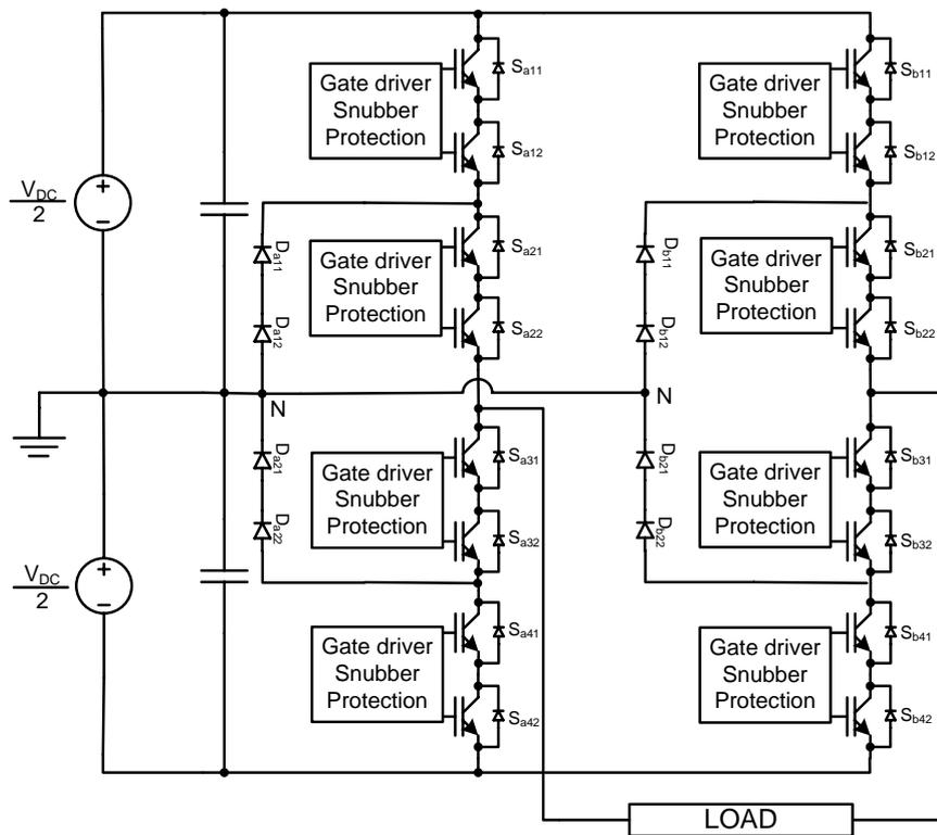
**Figure 7.1:** *Realized three-level inverter setup.*
