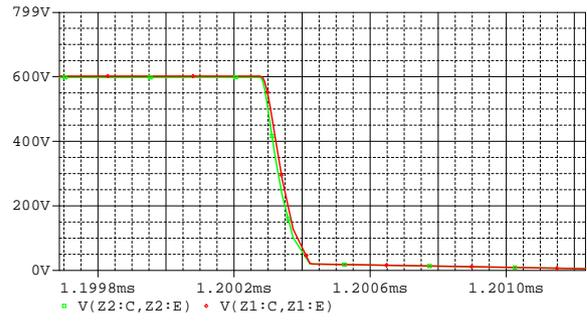
**Figure 3.7:** Turn on transition with added collector emitter capacitance. See schematic in figure 3.2.
