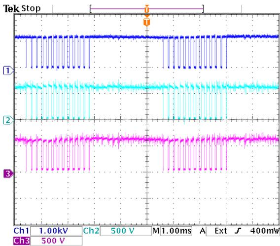
**Figure 9.35:** Voltage sharing of switch pair  $S_{a4}$ . Dark blue =  $v_{S_{a4}}$ , light blue =  $v_{S_{a41}}$ , purple =  $v_{S_{a42}}$ .
