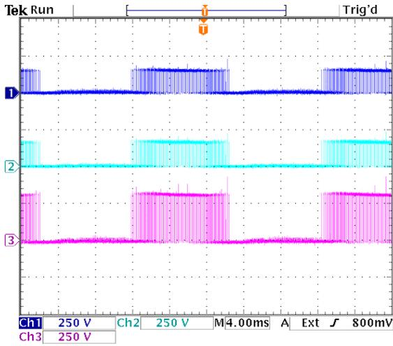
**Figure 9.11:** Voltage sharing of diode pair  $D_{a1}$ . Dark blue =  $v_{Da11}$ , light blue =  $v_{Da12}$ , purple =  $v_{Da1}$ .
