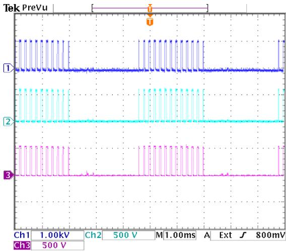
**Figure 9.37:** Voltage sharing of diode pair  $D_{a1}$ . Dark blue =  $v_{Da1}$ , light blue =  $v_{Da11}$ , purple =  $v_{Da12}$ .
