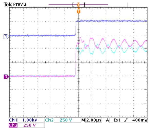
Figure 9.44: Zoom of turn off transition of switch pair  $S_{a2}$ . Dark blue =  $v_{S_{b2}}$ , light blue =  $v_{S_{b21}}$ , purple =  $v_{S_{b22}}$ .
