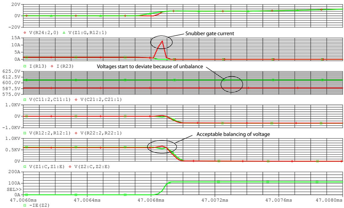
**Figure 4.45:** Zoom in of on transition simulation of the non ideal active gate control. (1)  $v_{ge1}$  and  $v_{ge2}$ , (2)  $i_{R13}$  and  $i_{R23}$ , (3)  $v_{C12}$  and  $v_{C22}$ , (4)  $v_{R11}$  and  $v_{R21}$ , (5)  $v_{ce,Z1}$  and  $v_{ce,Z2}$  and (6)  $i_{c,Z1}$ .
