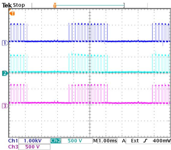
Figure 9.51: Voltage sharing of diode pair  $D_{b2}$ . Dark blue =  $v_{D_{b2}}$ , light blue =  $v_{D_{b21}}$ , purple =  $v_{D_{b22}}$ .
