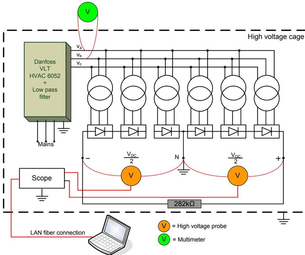
Figure D.16: Schematic view of medium voltage DC supply test setup.
