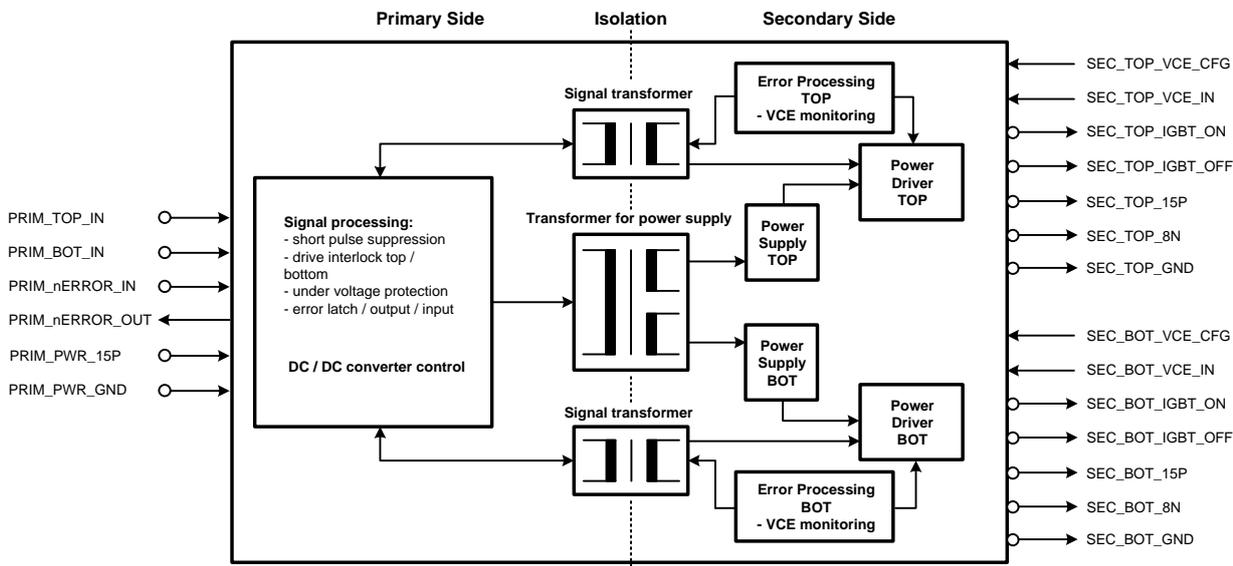
Figure 7.20: Schematic of the Semikron Skyper 32 gate driver [Semikron, 2007a].
