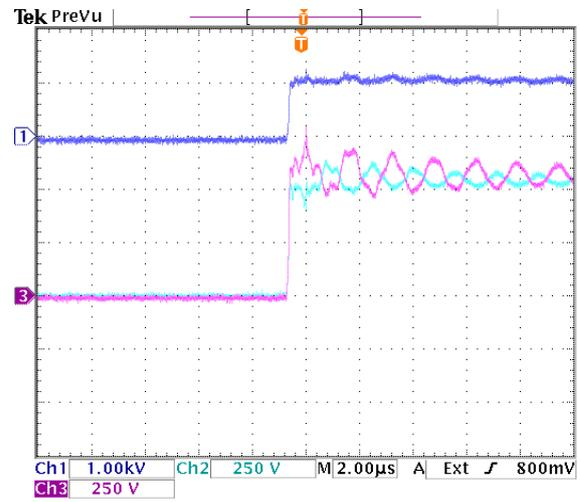
Figure 9.42: Zoom of turn off transition of switch pair  $S_{a2}$ . Dark blue =  $v_{S_{b1}}$ , light blue =  $v_{S_{b11}}$ , purple =  $v_{S_{b12}}$ .
