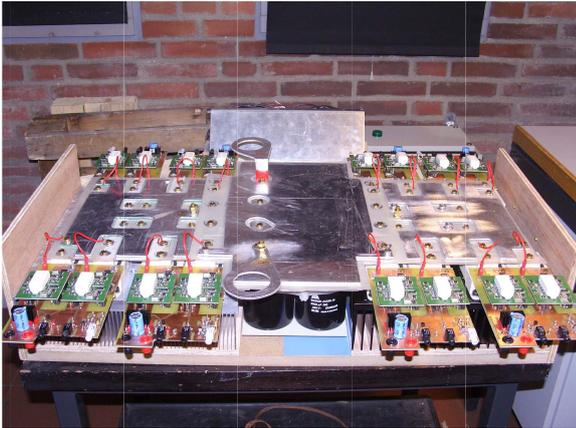
**Figure 8.10:** Layer four: Gate drivers and supply/safety terminals for grounding capacitors.
