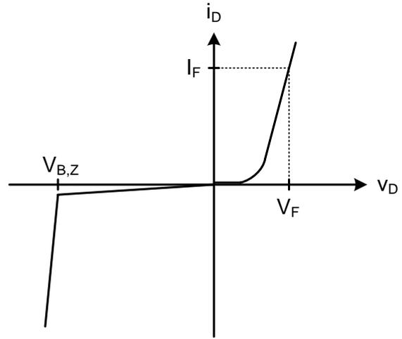
**Figure 4.48:**  $i/v$  curve for a zener diode.
