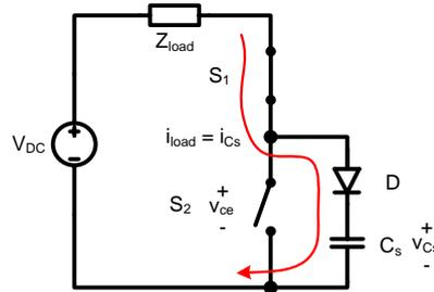
**Figure 4.12:** Current path when lower switch is off.
