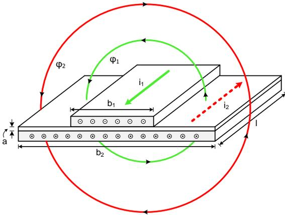
**Figure C.5:** One flat wire with non identical return path.
