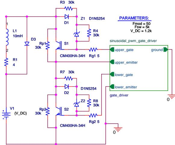
Figure 4.49: Zener clamped snubber simulation schematic. The zener break down voltage is defined to  $v_{B,Z} = 700V$ .
