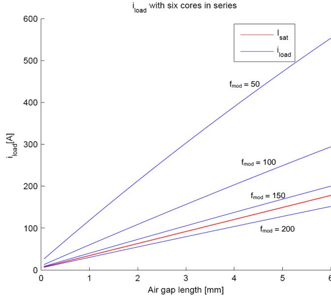
**Figure 7.9:**  $i_{load}$  and  $I_{sat}$  plotted as function of  $l_{gap}$  for  $f_{mod} = 50, 100, 150, 200Hz$  and  $v_{ab} = 2.4kV$ .
