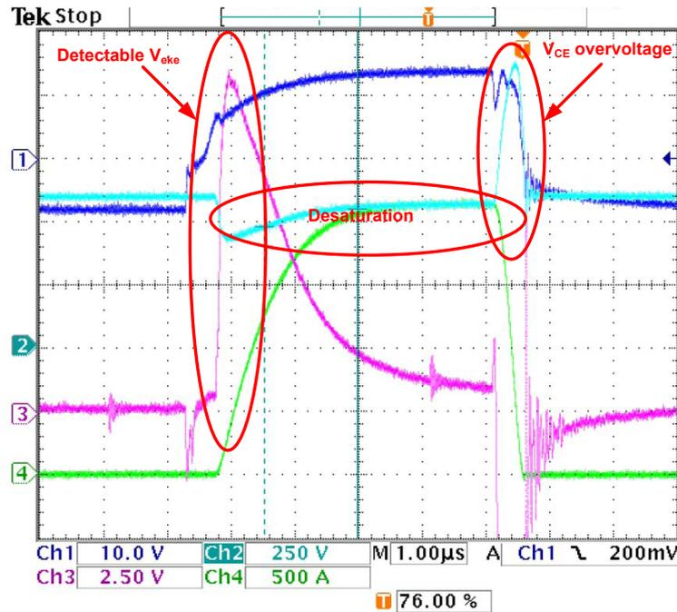
**Figure 5.12:** Short circuit test for  $V_{in} = 600V$ . Dark blue =  $v_{ge}$ , light blue =  $v_{ce}$ , purple =  $v_{eke}$ , green =  $i_c$ . Notice that the offset for  $v_{ce}$  has changed. Also notice that the desaturation occurs immediately.
