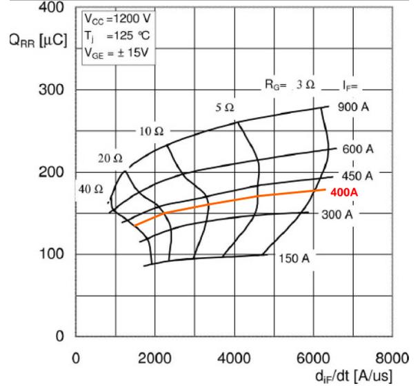
**Figure A.8:** Reverse recovery charge for the reverse diode as function of forward current and gate resistance for the SKM600GA176D [Semikron, 2006].
