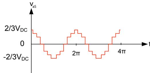
**Figure 2.5:**  $v_{as}$  voltage waveform.
