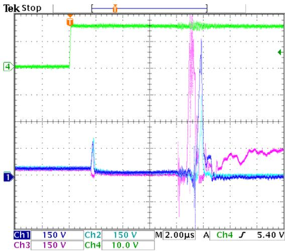
**Figure 9.57:** Short circuit test 1. Dark blue =  $v_{ce,Sa21}$ , light blue =  $v_{ce,Sa22}$ , purple =  $v_{ce,Sb31}$ , green = gate trigger signal.
