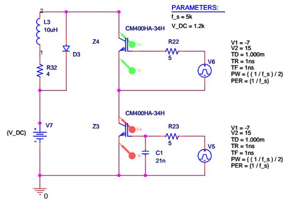
**Figure 3.3:** Schematic with added gate emitter capacitance shown as  $C_1 = 3.3nF$ . Results are shown in figures 3.8 and 3.9.
