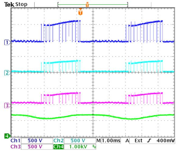
**Figure 9.25:** Voltage sharing of diode pair  $D_{a2}$ . Dark blue =  $v_{D_{a2}}$ , light blue =  $v_{D_{a21}}$ , purple =  $v_{D_{a22}}$ , green = DC link voltage.
