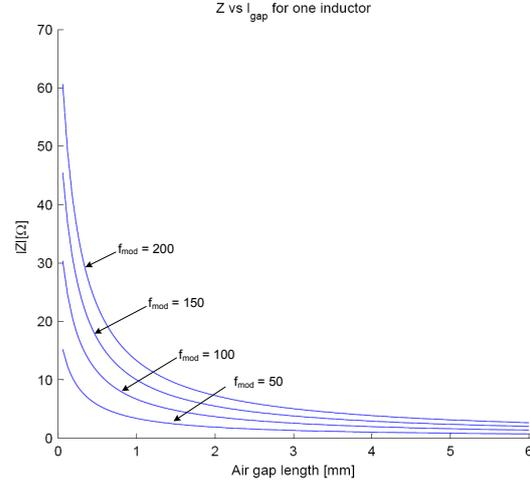
**Figure 7.8:** Impedance  $|Z|$  for one inductor as function of  $l_{gap}$  plotted for  $f_{mod} = 50, 100, 150, 200Hz$ . The largest frequency gives the largest impedance.
