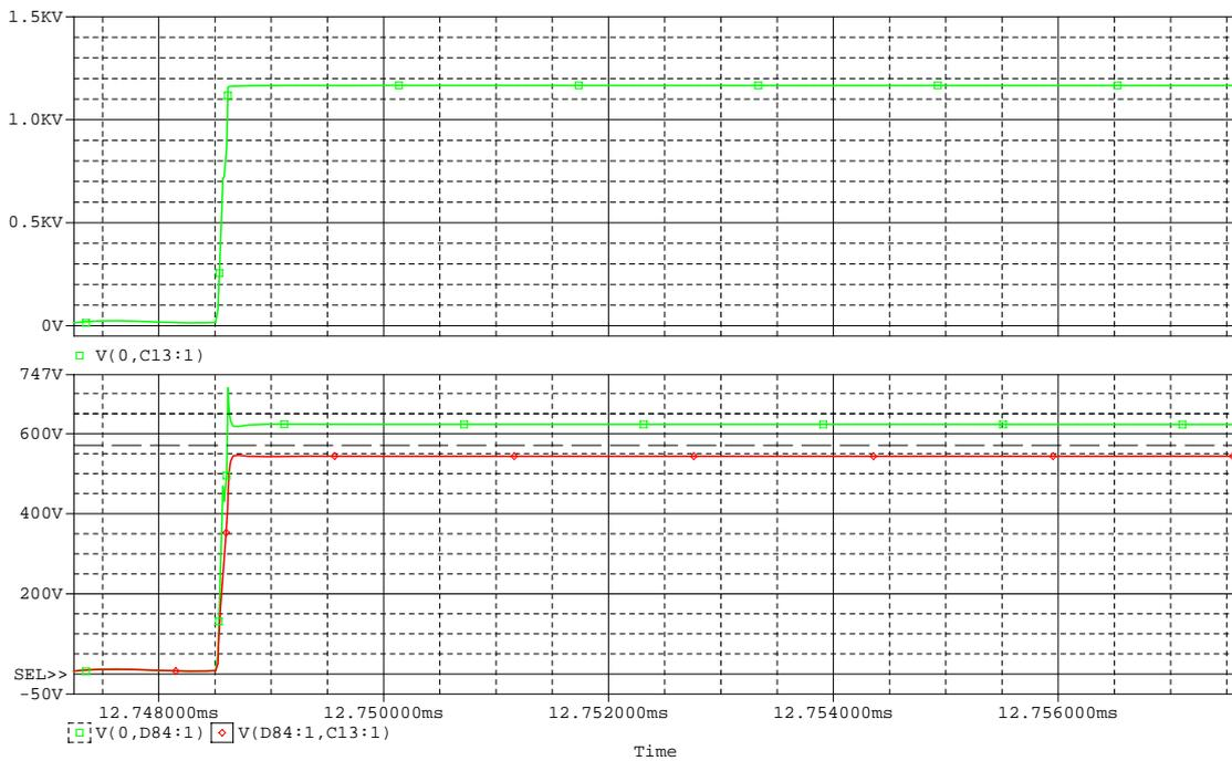
**Figure 8.5:** Voltage sharing for two diodes, together with the voltage across a diode pair. Top: Resulting waveform for diode  $D_{a31} + D_{a32}$ . Bottom;  $D_{a31}$  (green), and  $D_{a32}$  (red) with an added parallel capacitor of  $1.5nF$ .
