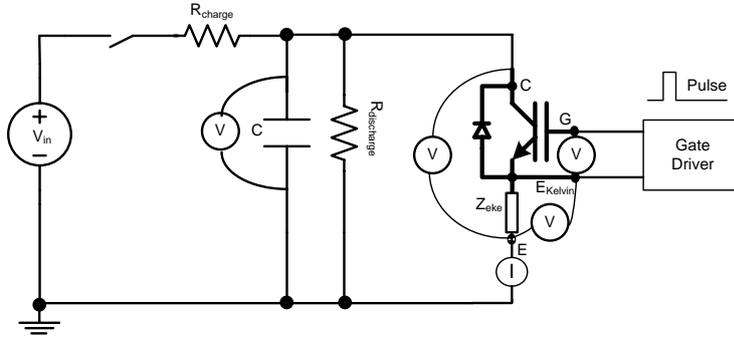
Figure D.2: Test setup for short circuit test.
