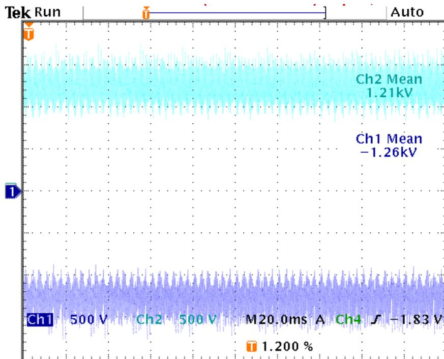
Figure D.22: DC link voltage for  $V_{ab} = 296V$ .
