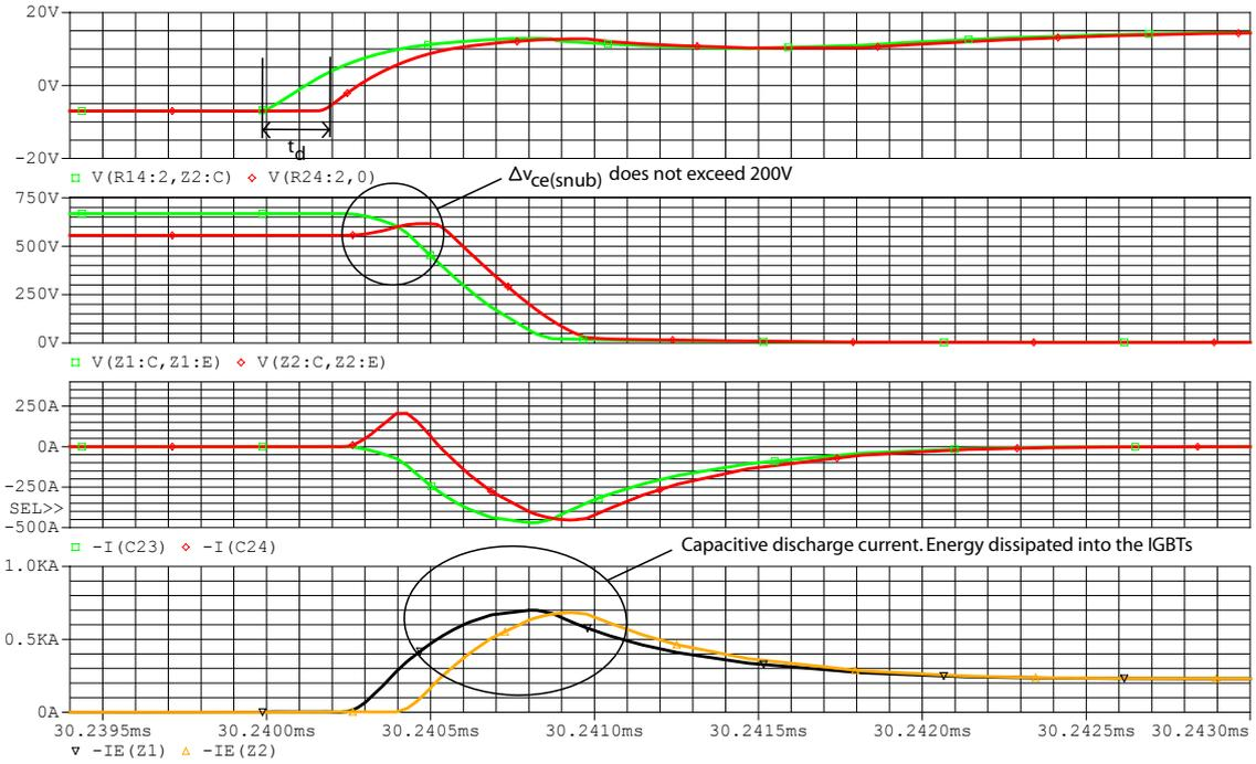
**Figure 4.17:** Simulation of on transition of passive snubber for series connected IGBTs. (1)  $v_{ge1}$  and  $v_{ge2}$ , (2)  $v_{ce,Z1}$  and  $v_{ce,Z2}$ , (3)  $i_{Cs1}$  and  $i_{Cs2}$  and (4)  $i_{c,Z1}$  and  $i_{c,Z2}$ .
