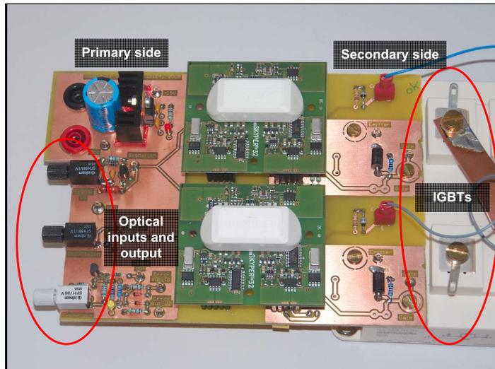
Figure 7.24: Photography of the gate driver board mounted on two IGBTs.
