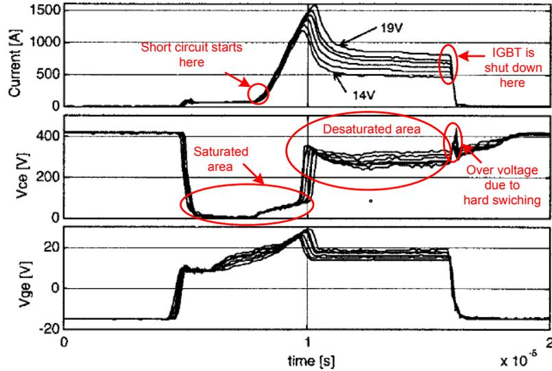
**Figure 5.6:** Short circuit characteristic of a Toshiba MG100Q2YS40 IGBT rated 1.2kV/100A [Vinod john, April 1999].
