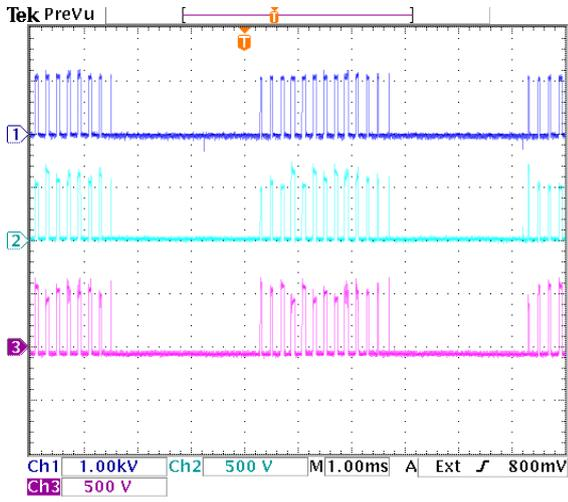
Figure 9.45: Voltage sharing of switch pair  $S_{b3}$ . Dark blue =  $v_{S_{b3}}$ , light blue =  $v_{S_{b31}}$ , purple =  $v_{S_{b32}}$ .
