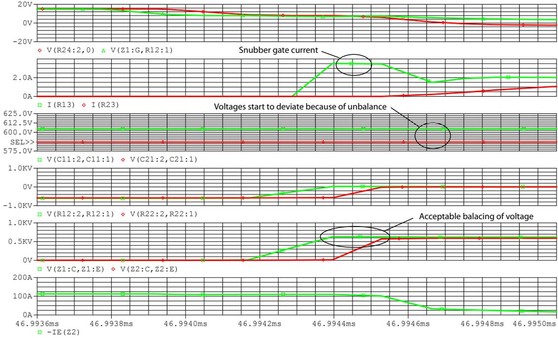
**Figure 4.46:** Zoom in of off transition simulation of the non ideal active gate control. (1)  $v_{ge1}$  and  $v_{ge2}$ , (2)  $i_{R13}$  and  $i_{R23}$ , (3)  $v_{C12}$  and  $v_{C22}$ , (4)  $v_{R11}$  and  $v_{R21}$ , (5)  $v_{ce,Z1}$  and  $v_{ce,Z2}$  and (6)  $i_{c,Z1}$ .
