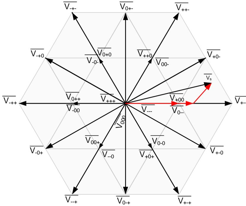
Figure 2.14: SVM states in the three-level inverter.
