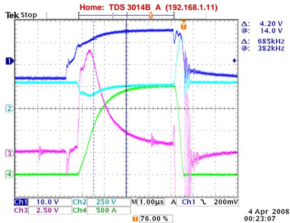
**Figure D.5:** Short circuit test for  $V_{in} = 300V$ . Dark blue =  $v_{ge}$ , light blue =  $v_{ce}$ , purple =  $v_{eke}$ , green =  $i_C$ .
