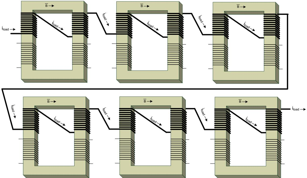
Figure 7.3: Realized load inductor layout.
