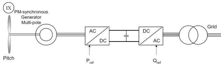
**Figure 1.2:** *Electrical system in a turbine with permanent magnet generator [Blaabjerg, 2006].*
