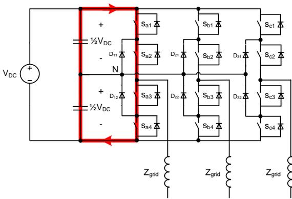
**Figure 5.3:** Fast fault with shoot through in one phase leg. Characterized by very fast current rise.
