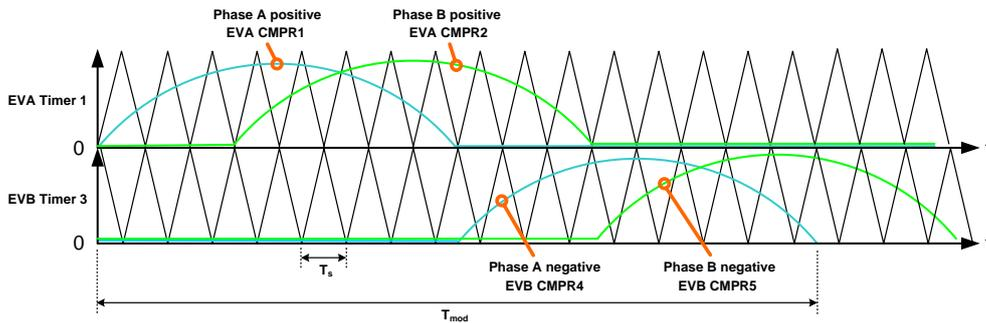
**Figure 7.15:** Modified PWM scheme for the three level inverter with only positive wave form values. Blue: Phase A and green: Phase B. Notice, that the third harmonic waveform is not included in the figure.
