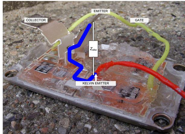
**Figure 5.10:** Picture of the Semikron IGBT internal.  $Z_{ek_e}$  is shown by the blue line.
