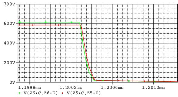
**Figure 3.11:** Turn on transition with added gate resistance. See schematic in figure 3.4.
