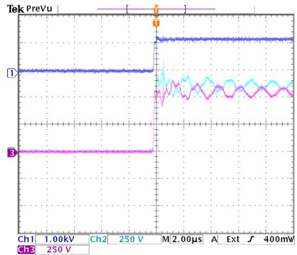
**Figure 9.36:** Zoom of turn off transition of switch pair  $S_{a4}$ . Dark blue =  $v_{S_{a4}}$ , light blue =  $v_{S_{a41}}$ , purple =  $v_{S_{a42}}$ .
