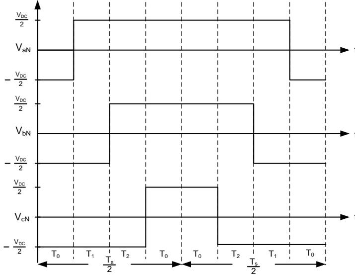
**Figure 2.11:** Phase voltage representation of equation (2.58).
