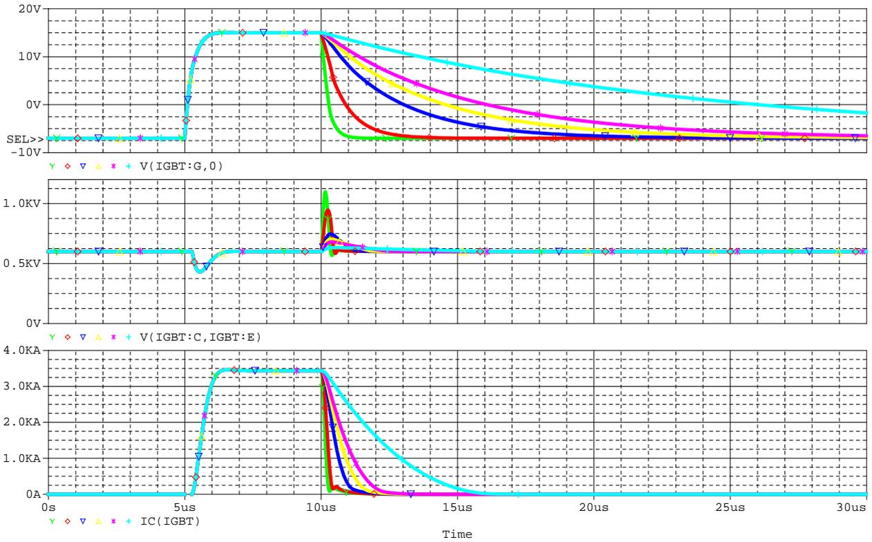
**Figure 5.16:** Simulation results of soft shutdown protection.  $R_{SS}=4.7(Y)$ ,  $15(\diamond)$ ,  $50(\nabla)$ ,  $75(\Delta)$ ,  $100(*)$ ,  $263(+)[\Omega]$  used for parameter sweep analysis. From the top:  $v_{ge}$ ,  $v_{ce}$  and  $i_c$ .
