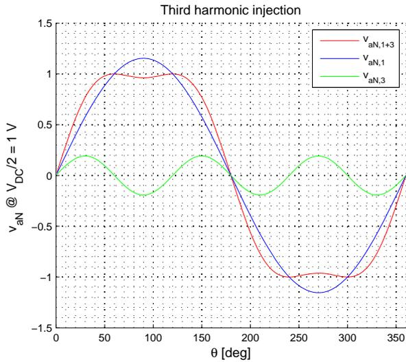
**Figure 2.8:** First harmonic, third harmonic and resulting waveform for  $Ma_1 = 1.16$ .
