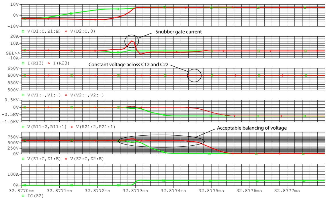
**Figure 4.40:** Zoom in of simulation of an on transition by the ideal active gate control (constant voltage across  $C_{11}$  and  $C_{21}$ ). (1)  $v_{ge1}$  and  $v_{ge2}$ , (2)  $i_{R13}$  and  $i_{R23}$ , (3)  $v_{C12}$  and  $v_{C22}$ , (4)  $v_{R11}$  and  $v_{R21}$ , (5)  $v_{ce,Z1}$  and  $v_{ce,Z2}$  and (6)  $i_{c,Z1}$ .
