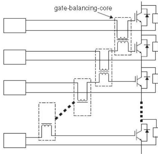
**Figure 4.4:** Gate balancing core method [N.Y.A. Shamma & Chamud, February 2006].
