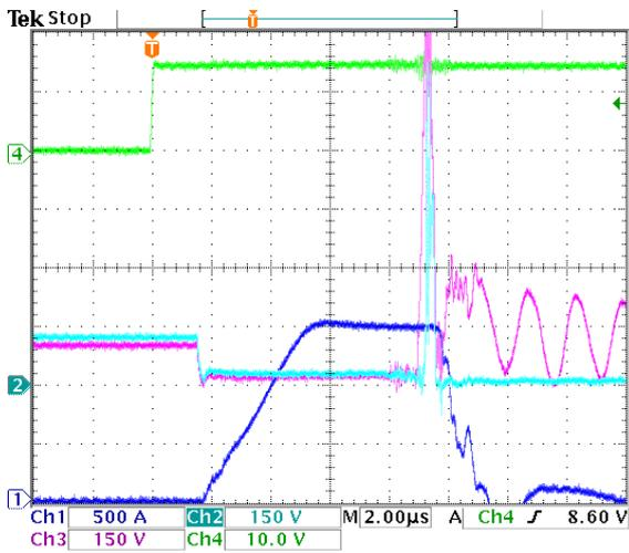
**Figure 9.55:** Short circuit test 1. Dark blue =  $i_{load}$ , light blue =  $v_{ce,Sa11}$ , purple =  $v_{ce,Sa12}$ , green = gate trigger signal.
