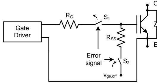
Figure 5.13: Soft shut down implementation schematic.
