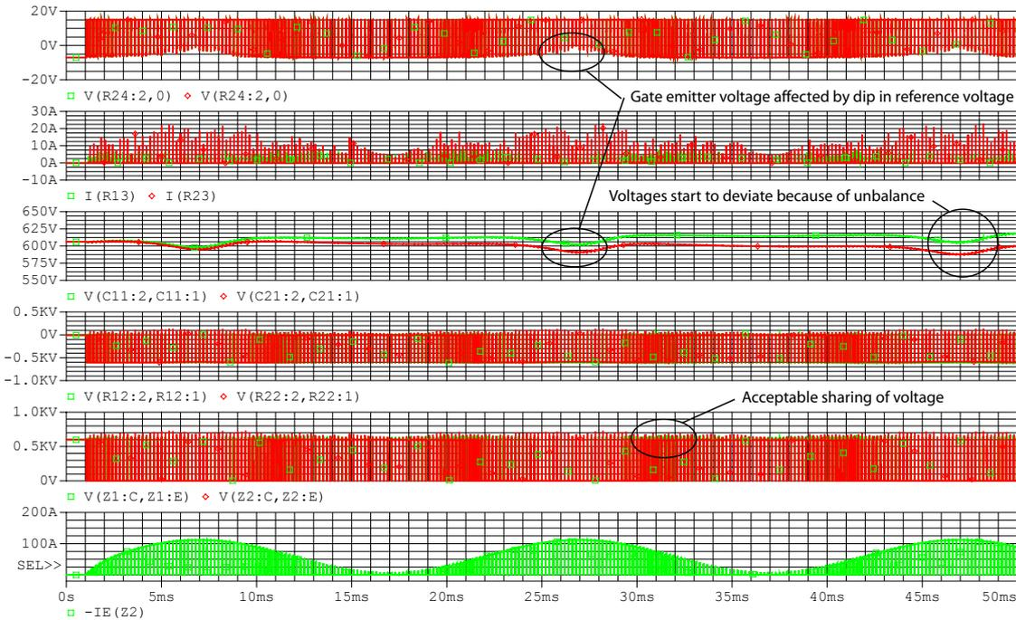
**Figure 4.44:** Simulation of the non ideal active gate control. (1)  $v_{ge1}$  and  $v_{ge2}$ , (2)  $i_{R13}$  and  $i_{R23}$ , (3)  $v_{C12}$  and  $v_{C22}$ , (4)  $v_{R11}$  and  $v_{R21}$ , (5)  $v_{ce,Z1}$  and  $v_{ce,Z2}$  and (6)  $i_{c,Z1}$ .
