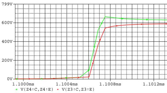
**Figure 3.8:** Turn off transition with added gate emitter capacitance. See schematic in figure 3.3.
