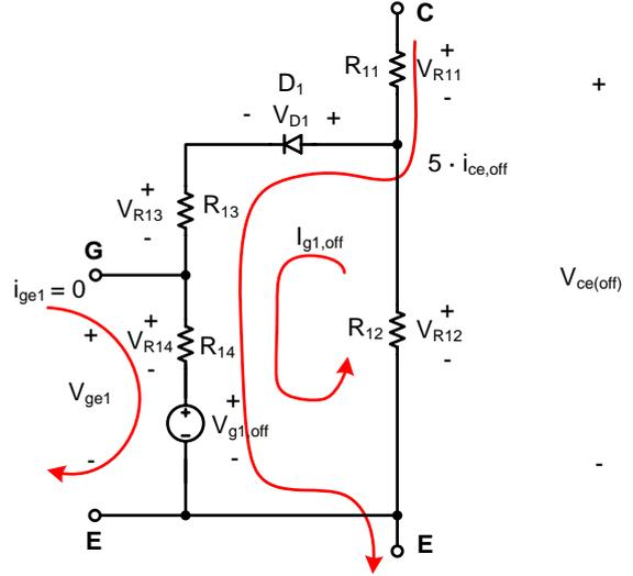
**Figure 4.35:** Schematic of current paths with gate driver in off state.
