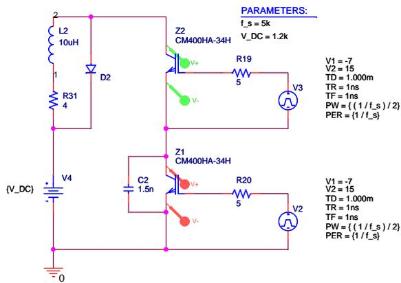
**Figure 3.2:** Schematic with added collector emitter capacitance shown as  $C_2 = 2.7nF$ . Results are shown in figures 3.6 and 3.7.
