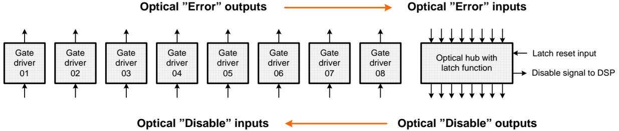
**Figure 7.31:** Block diagram of the optical hub used for fast fault protection. The detection of the fast fault is performed by the gate drivers.
