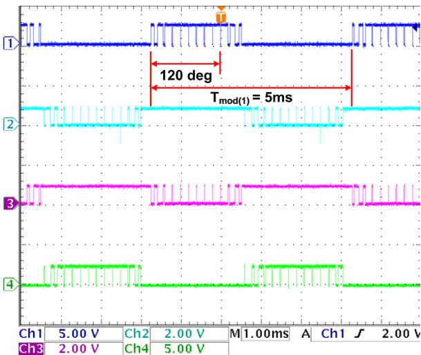
**Figure 7.16:** Measured PWM signals for phase A. From the top:  $A_1$  to  $A_4$ .
