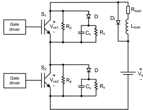
Figure 4.9: Schematic of two passive snubbers.
