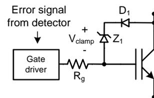
**Figure 5.17:** Schematic of break down protection by voltage clamping. The error signal is received from the error detector.
