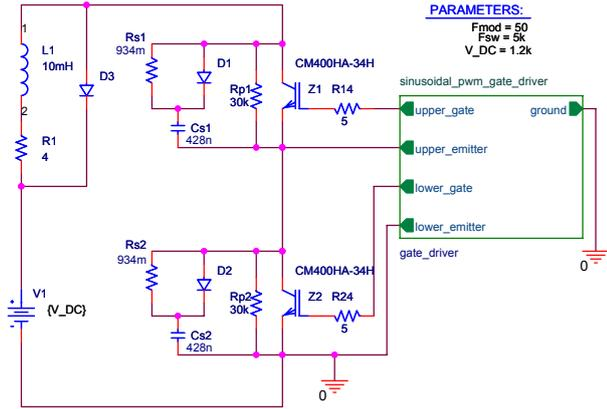
Figure 4.13: Simulation schematic for passive snubber.
