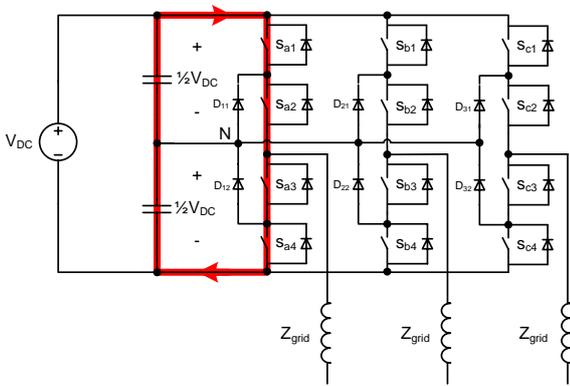
**Figure B.3:** Fast fault with shoot through in one phase leg. Characterized by very fast current rise.
