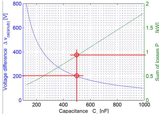
**Figure 4.25:** Plot of acceptable voltage difference  $\Delta v_{ce,snub}$  between two switches in off state, required snubber capacitance  $C_s$  and related losses  $P_{loss}$ . Fixed parameters are  $I_{load} = 300A$  and  $f_{sw} = 5kHz$ .
