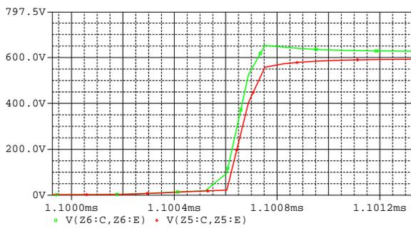
**Figure 3.10:** Turn off transition with added gate resistance. See schematic in figure 3.4.
