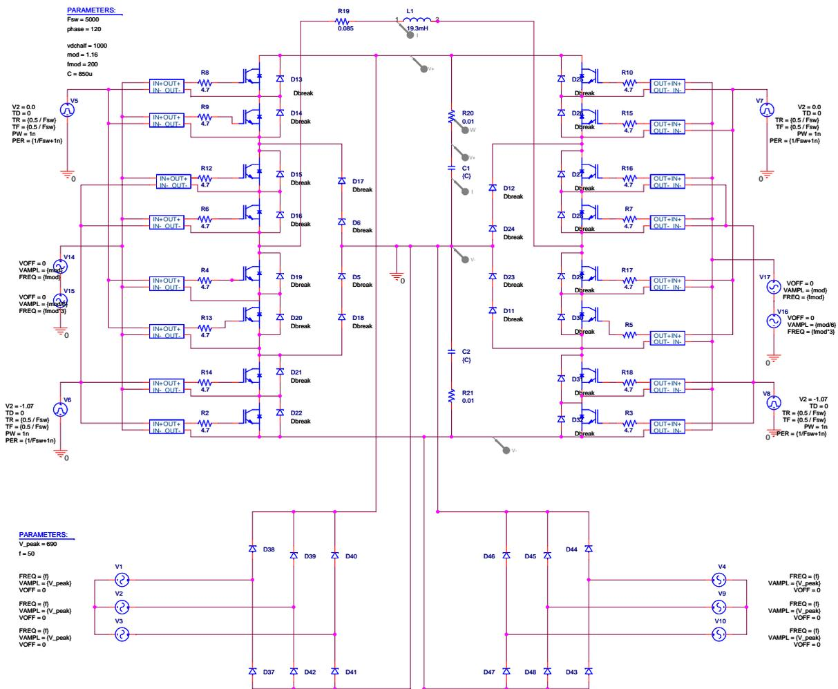
Figure D.25: OrCad simulation schematic for capacitor simulation.
