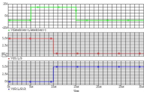
**Figure 5.15:** Control signals for soft shut down simulation. From the top  $v_{ge}$ ,  $v_{error}$  for S1 and  $v_{error}$  for S2.
