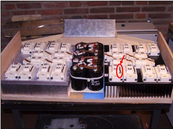
**Figure 8.6:** Bottom layer: Layout of the IGBTs, the heat sinks and the neutral point capacitor bank. The zener clamped snubber / protection can be seen next to each IGBT terminal.
