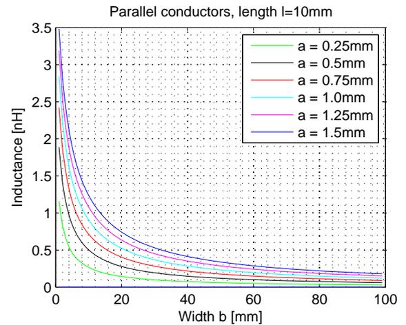
**Figure C.6:** Self inductance for two flat parallel non identical wires according to equation (C.5).
