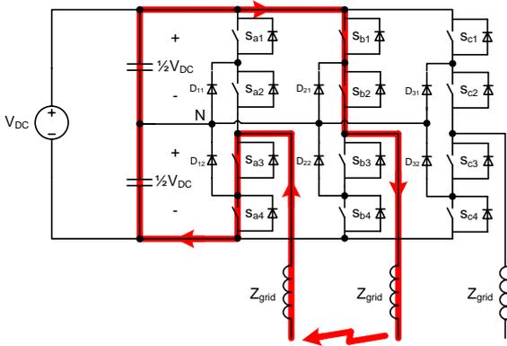
**Figure B.6:** Slow fault with phase to phase short circuit.
