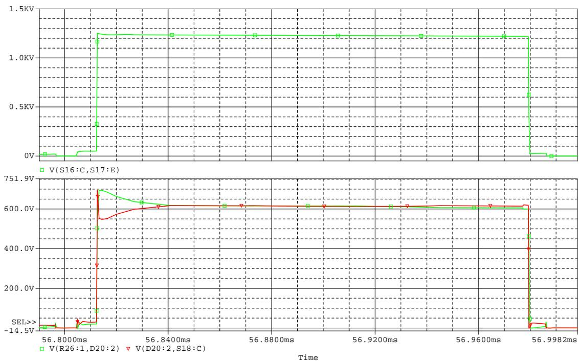
**Figure 8.4:** Voltage sharing for two IGBTs, together with the voltage across a switch pair. Top: Resulting waveform for switch  $S_{a31} + S_{a32}$ . Bottom:  $S_{a31}$  (green), and  $S_{a32}$  with an added gate signal delay of 170ns.
