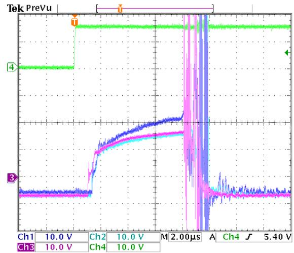
**Figure 9.58:** Gate signals of short circuit test 1. Dark blue =  $v_{ge,Sa21}$ , light blue =  $v_{ge,Sa22}$ , purple =  $v_{ge,Sb31}$ , green = gate trigger signal.
