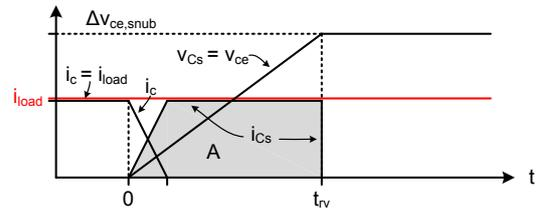
**Figure 4.11:** Voltage and current waveforms for IGBT and snubber in figure 4.9.
