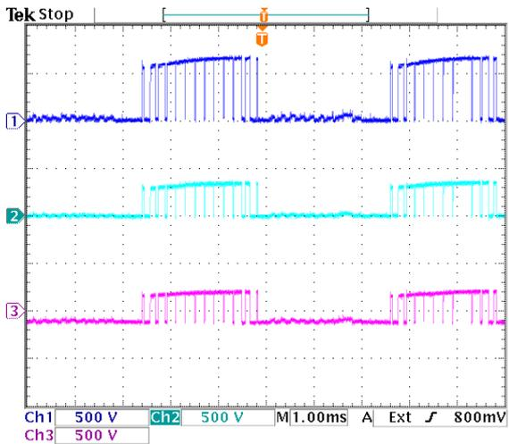
**Figure 9.26:** Voltage sharing of diode pair  $D_{b1}$ . Dark blue =  $v_{D_{b1}}$ , light blue =  $v_{D_{b11}}$ , purple =  $v_{D_{b12}}$ .
