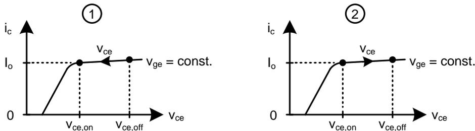
Figure A.5: Transfer curve for the IGBT. (1) in the turn on. (2) in the turn off.
