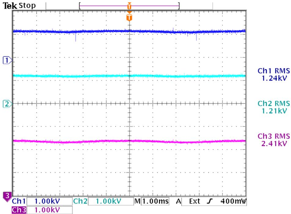
Figure 9.53: DC link voltage. Dark blue = upper  $\frac{V_{DC}}{2}$ , light blue = lower  $\frac{V_{DC}}{2}$ , purple =  $V_{DC}$ .
