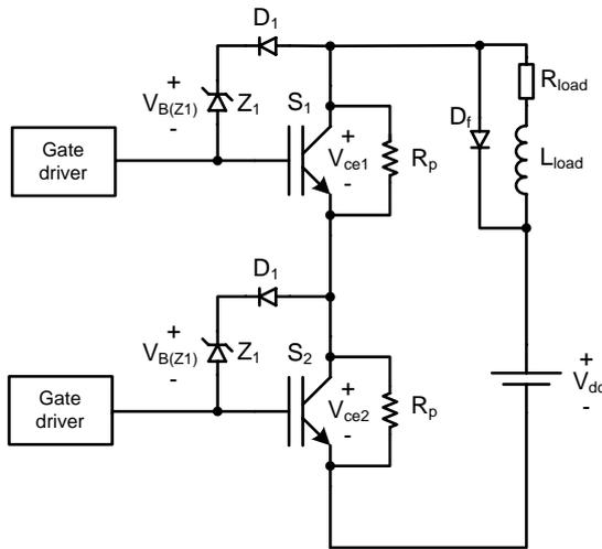
**Figure 4.5:** Voltage clamping by a zener diode between collector and gate.
