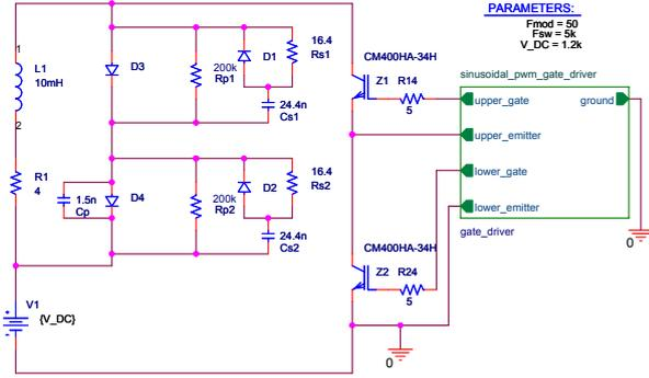
**Figure 4.18:** Simulation schematic for the passive snubber for diodes - here used for two free wheeling diodes.
