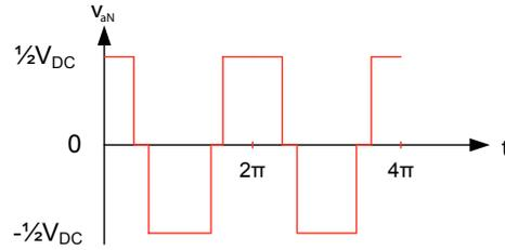
**Figure 2.2:**  $v_{aN}$  voltage waveform.
