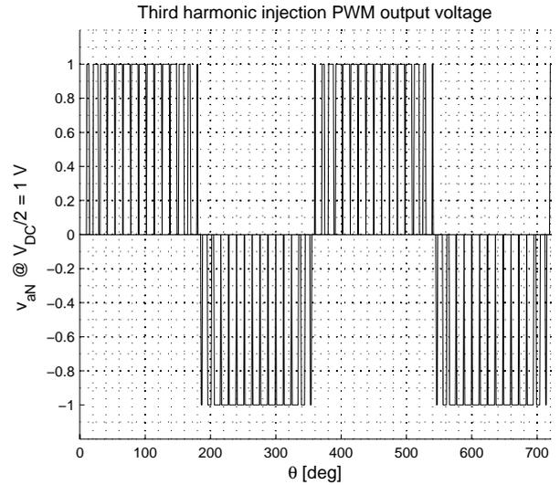
**Figure 2.9:** PWM output voltage for carrier based modulation.
