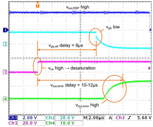
**Figure 7.28:** Zoom of gate driver signals in desaturation situation. Blue:  $v_{out,DSP}$ , magenta:  $v_{ge}$ , purple:  $v_{ce}$  and green:  $v_{out,error}$ .
