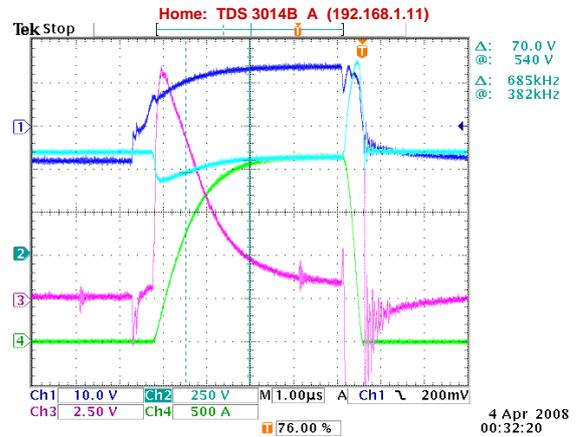
Figure D.8: Short circuit test for  $V_{in} = 600V$ . Dark blue =  $v_{ge}$ , light blue =  $v_{ce}$ , purple =  $v_{eke}$ , green =  $i_C$ . Notice that the offset for  $v_{ce}$  has changed.
