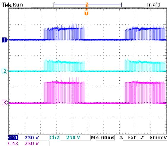
**Figure 9.5:** Voltage sharing of switch pair  $S_{a3}$ . Dark blue =  $v_{Sa31}$ , light blue =  $v_{Sa32}$ , purple =  $v_{Sa3}$ .
