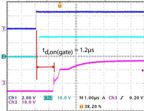
**Figure 7.25:** Measured gate driver signals in turn on transition. Blue:  $v_{out,DSP}$ , magenta:  $v_{in,gate}$  and purple:  $v_{ge}$ .
