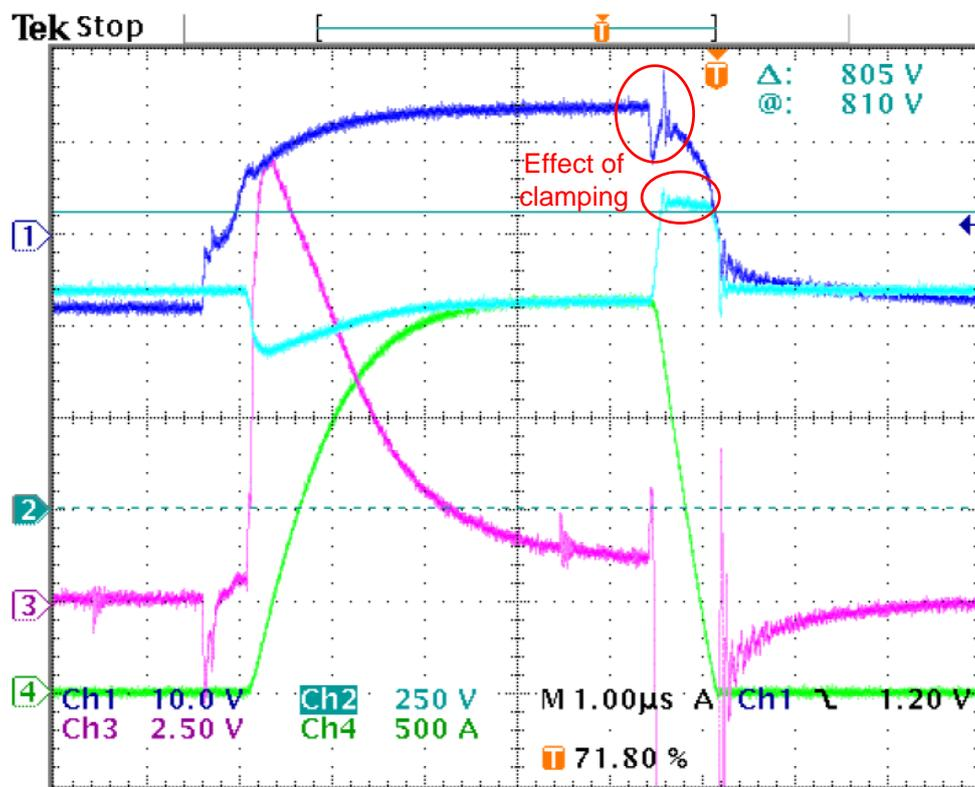
Figure D.13: Short circuit test for  $V_{in} = 600V$  with added clamping protection. Dark blue =  $v_{ge}$ , light blue =  $v_{ce}$ , purple =  $v_{ke}$ , green =  $i_c$ .
