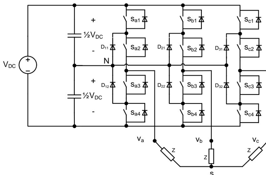
**Figure 2.1:** Three-level three phase inverter schematic with star connected load.
