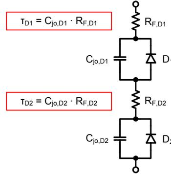
**Figure 4.20:** Circuit model of two diodes in series, each with individual forward resistance  $R_F$  and junction capacitance  $C_{j0}$ .
