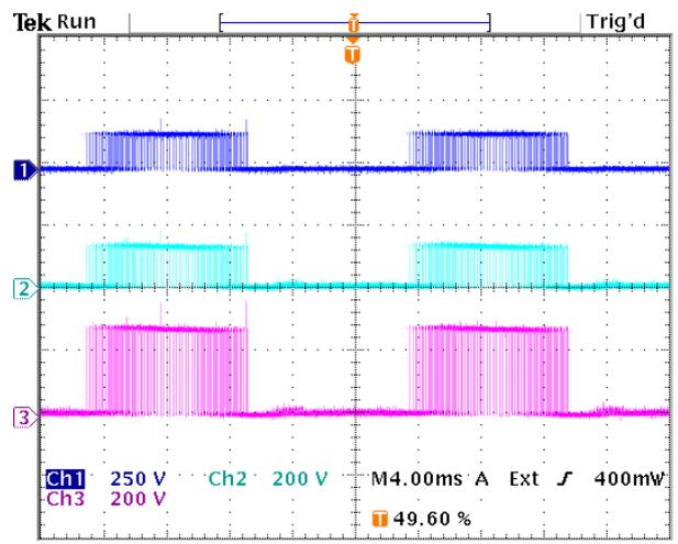
**Figure 9.12:** Voltage sharing of diode pair  $D_{a1}$ . Dark blue =  $v_{Da21}$ , light blue =  $v_{Da22}$ , purple =  $v_{Da2}$ .
