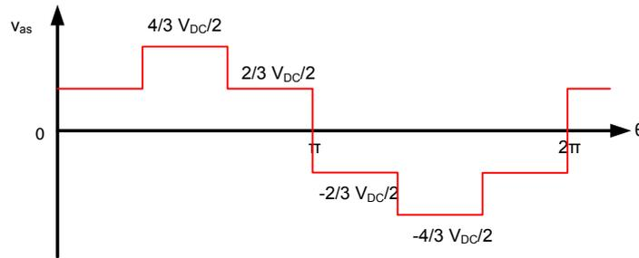
**Figure 2.6:** Phase to star-point voltage  $v_{as}$  levels for two-level inverter. Freely after [Lipo, 2003].
