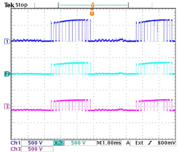
**Figure 9.27:** Voltage sharing of diode pair  $D_{b2}$ . Dark blue =  $v_{D_{b2}}$ , light blue =  $v_{D_{b21}}$ , purple =  $v_{D_{b22}}$ .
