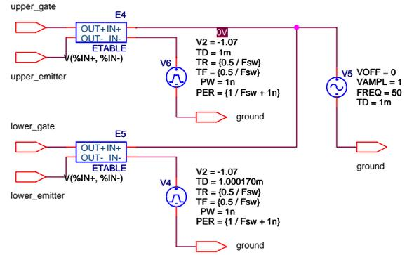
Figure 4.50: Simulation schematic for sinusoidal PWM circuit with  $t_d = 170ns$  and  $f_{mod} = 50Hz$ .
