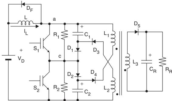
**Figure 4.7:** Voltage clamping by diodes and capacitors [N.Y.A. Shamma & Chamud, February 2006].
