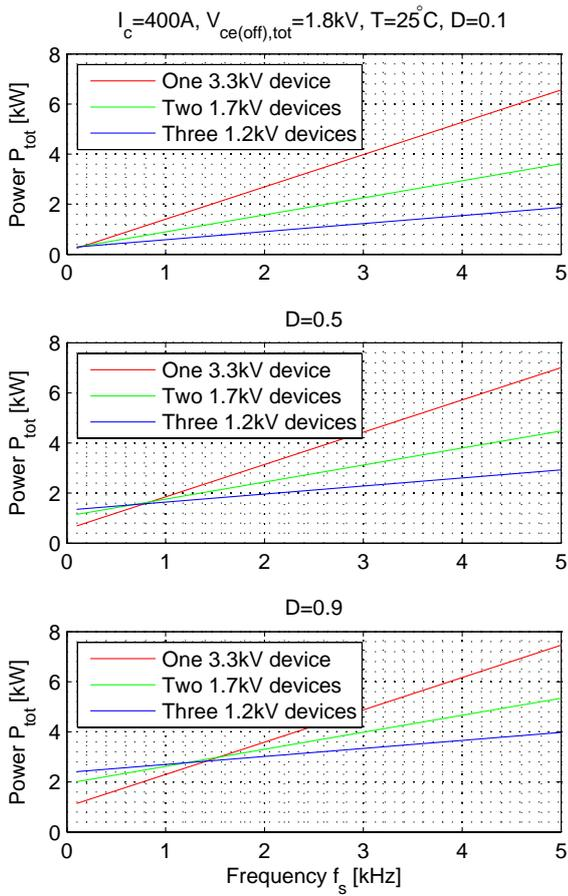
**Figure 3.14:** Total losses at  $T = 25^\circ\text{C}$  with duty cycle  $D = 0.1$ ,  $D = 0.5$  and  $D = 0.9$ .
