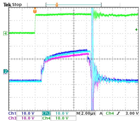
**Figure 9.66:** Gate signals of short circuit test 2. Dark blue =  $v_{ge,Sa32}$ , light blue =  $v_{ge,Sa41}$ , purple =  $v_{ge,Sa42}$ , green = gate trigger signal.
