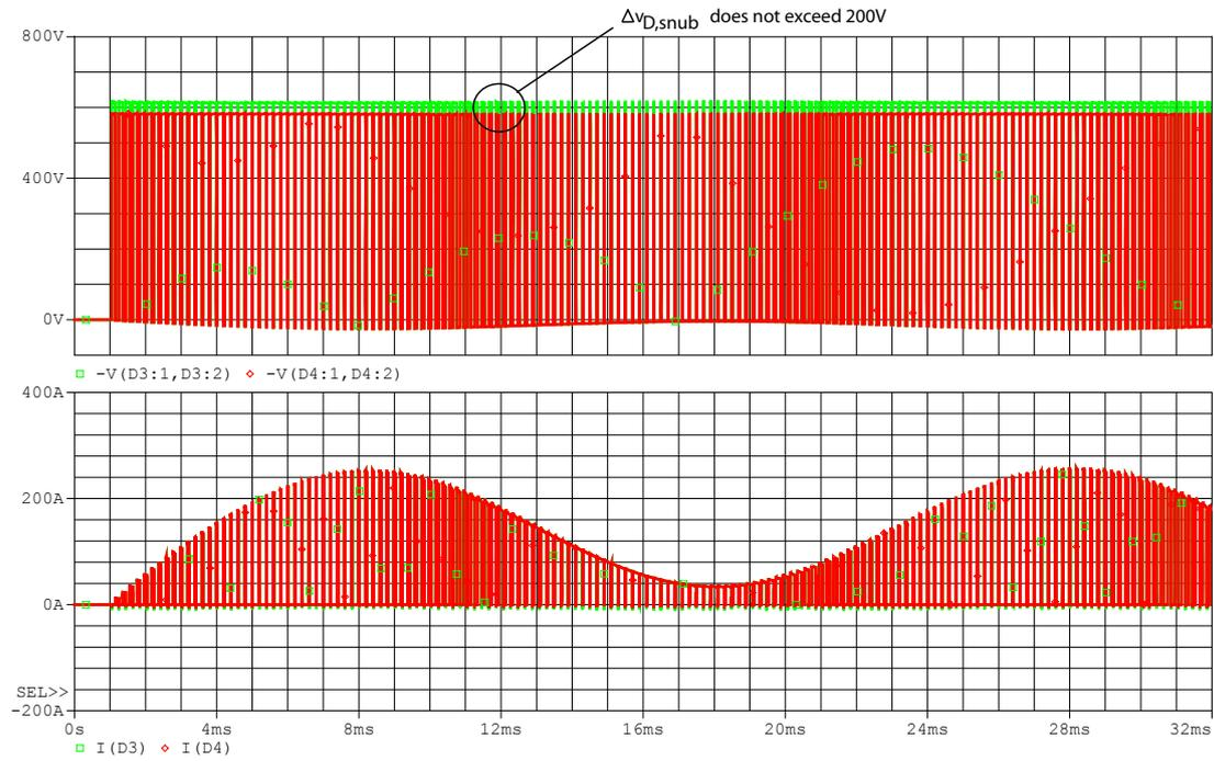
Figure 4.22: Simulation of passive snubber for series connected diodes. (1)  $v_{D3}$  and  $v_{D4}$ , (2)  $i_{D3}$  and  $i_{D4}$ .
