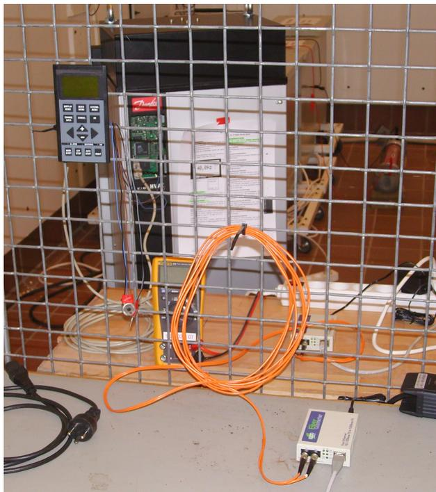
**Figure D.19:** *The Danfoss HVAC 6052 VLT. Notice the display on the cage and the two fiber converters connected via the orange fiber. This equipment is used to control the VLT and the scopes by LAN interface.*
