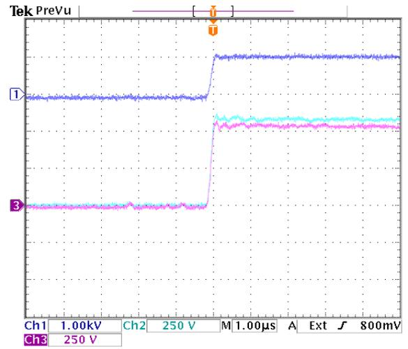
**Figure 9.38:** Zoom of turn off transition of the diode pair  $D_{a1}$ . Dark blue =  $v_{Da1}$ , light blue =  $v_{Da11}$ , purple =  $v_{Da12}$ .
