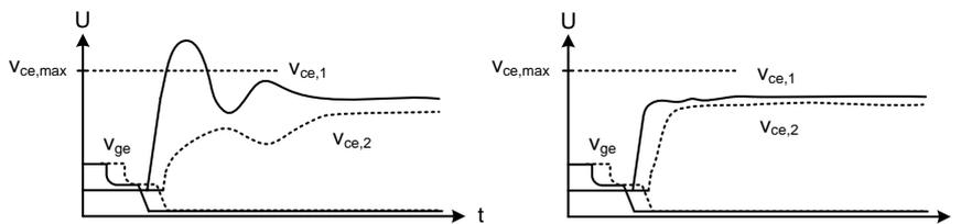
**Figure 3.1:** Switch voltages for two switches with (a) unequal voltage sharing, and (b) equal voltage sharing.
