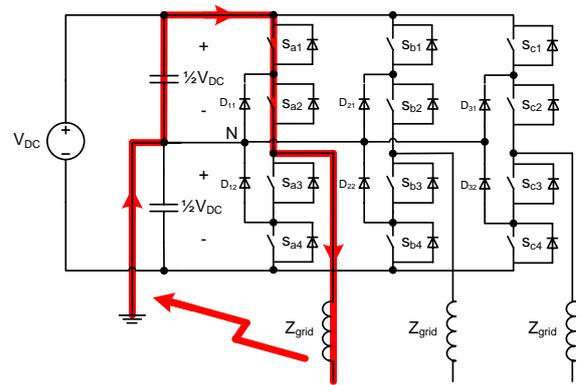
**Figure B.7:** Slow fault with phase to ground short circuit.
