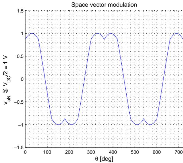
**Figure 2.12:** Space vector output wave form for  $v_{aN}$ .
