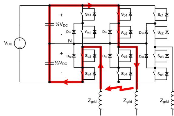
**Figure B.4:** Fast fault with phase to phase short circuit. Characterized by very fast current rise.
