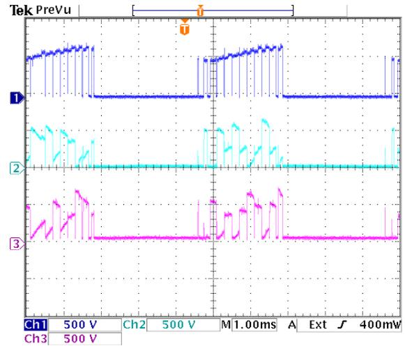
**Figure 9.17:** Voltage sharing of switch pair  $S_{a2}$ . Dark blue =  $v_{S_{a2}}$ , light blue =  $v_{S_{a21}}$ , purple =  $v_{S_{a22}}$ .
