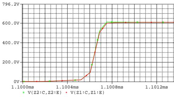
**Figure 3.6:** Turn off transition with added collector emitter capacitance. See schematic in figure 3.2.
