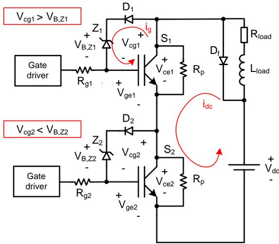
**Figure 4.47:** Zener clamped snubber schematic showing current paths in a turn off transient with  $S_1$  turning off quicker than  $S_2$ .
