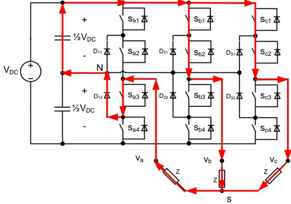
**Figure 2.15:** Current flow for state  $(0, +, +)$ . Notice that the current is entering the neutral point, hence discharging the top capacitor.
