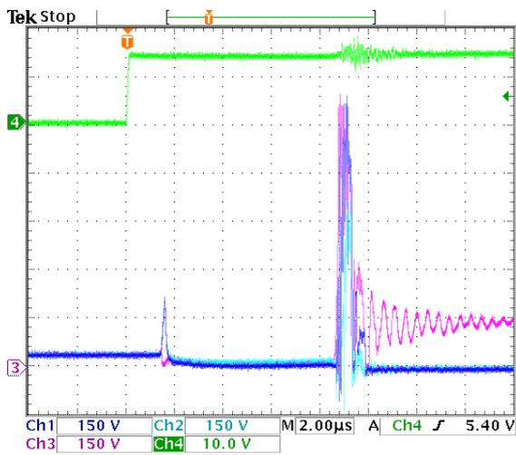
**Figure 9.63:** Short circuit test 2. Dark blue =  $v_{ce,Sb21}$ , light blue =  $v_{ce,Sb22}$ , purple =  $v_{ce,Sa31}$ , green = gate trigger signal.
