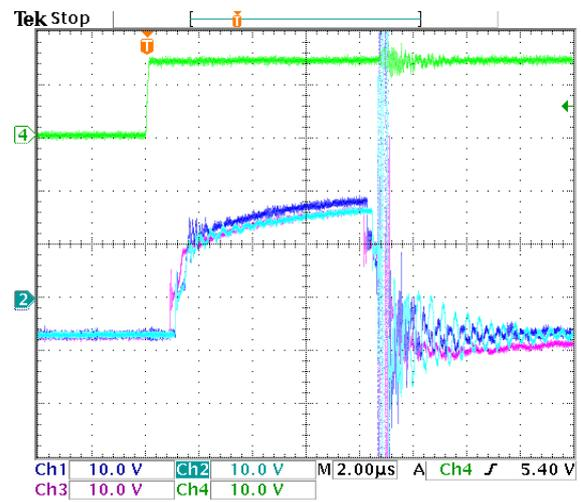
**Figure 9.64:** Gate signals of short circuit test 2. Dark blue =  $v_{ge,Sb21}$ , light blue =  $v_{ge,Sb22}$ , purple =  $v_{ge,Sa31}$ , green = gate trigger signal.
