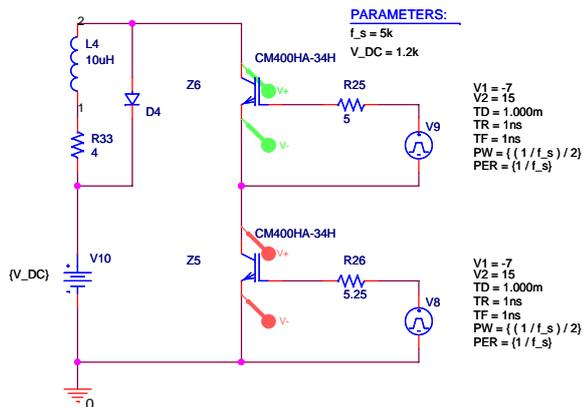
**Figure 3.4:** Schematic with added gate resistance shown as  $R_{26} = 5.25\Omega$ . Results are shown in figures 3.10 and 3.11.
