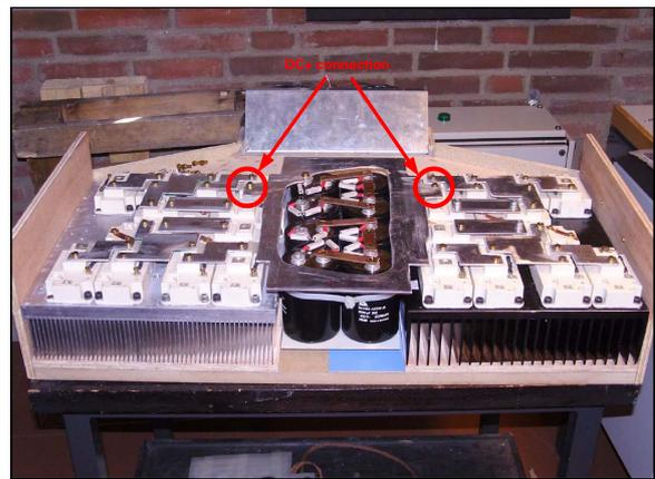
**Figure 8.7:** Layer one: Realized connections between switches and the positive supply plate DC+.
