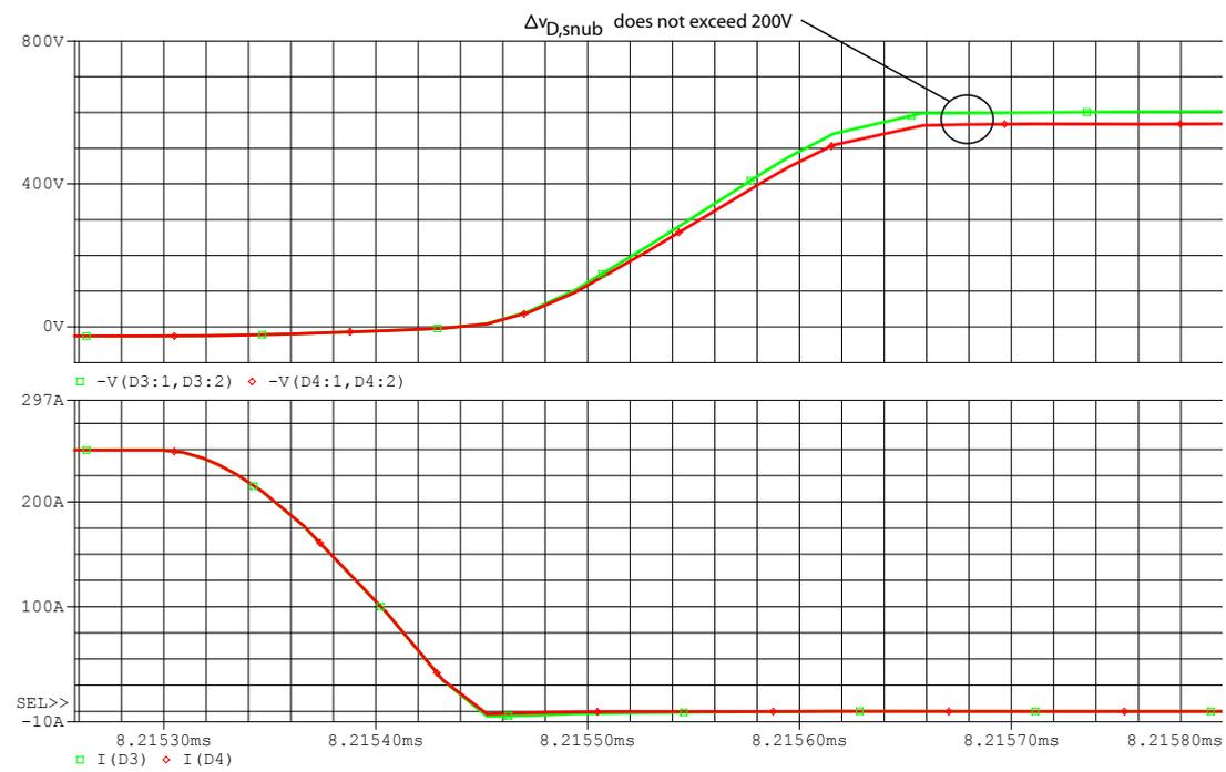
Figure 4.23: Simulation of off transition of passive snubber for series connected diodes. (1)  $v_{D3}$  and  $v_{D4}$ , (2)  $i_{D3}$  and  $i_{D4}$ .
