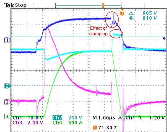
**Figure 5.19:** Short circuit test with added clamping protection for  $V_{in} = 600V$ . Dark blue =  $v_{ge}$ , light blue =  $v_{ce}$ , purple =  $v_{eke}$  and green =  $i_c$ .
