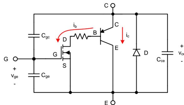
**Figure A.1:** *Equivalent circuit for the IGBT.*
