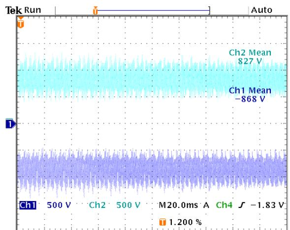
Figure D.21: DC link voltage for  $V_{ab} = 200V$ .
