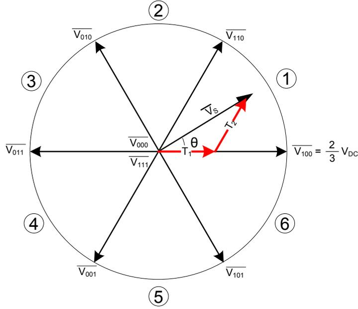
Figure 2.10: SVM states in the two-level inverter.
