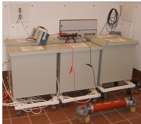
Figure D.18: The six AXA transformers with the diode bridge from figure D.17 on top. In the bottom, the load resistor is seen.
