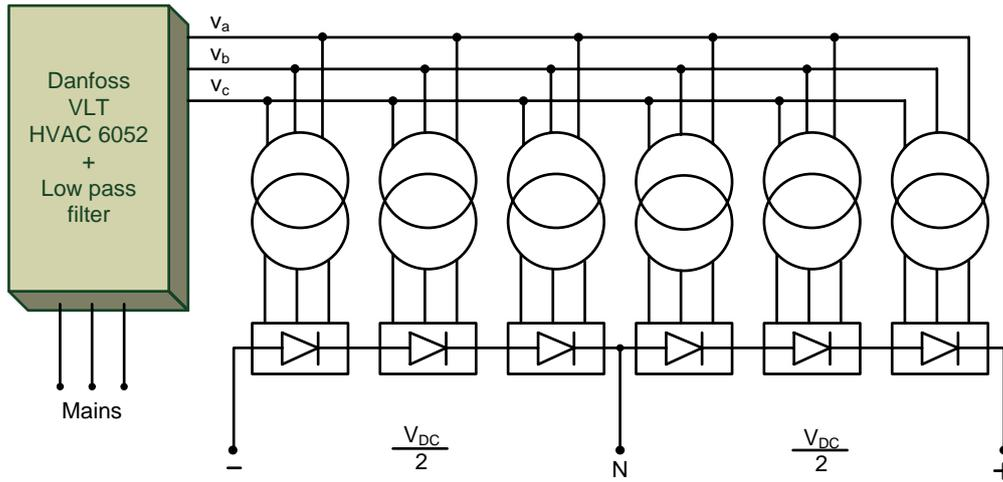
Figure D.14: Medium voltage DC supply.
