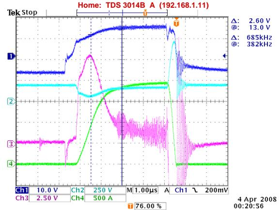
**Figure D.4:** Short circuit test for  $V_{in} = 200V$ . Dark blue =  $v_{ge}$ , light blue =  $v_{ce}$ , purple =  $v_{eke}$ , green =  $i_C$ .
