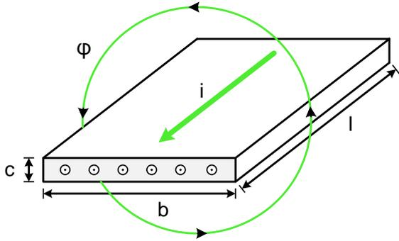
Figure C.1: Layout of a single flat wire with no current return path.
