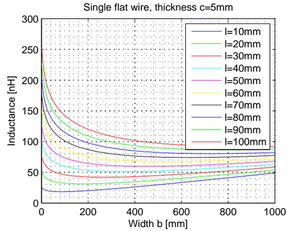
Figure C.2: Self inductance one flat parallel wire according to equation (C.3).
