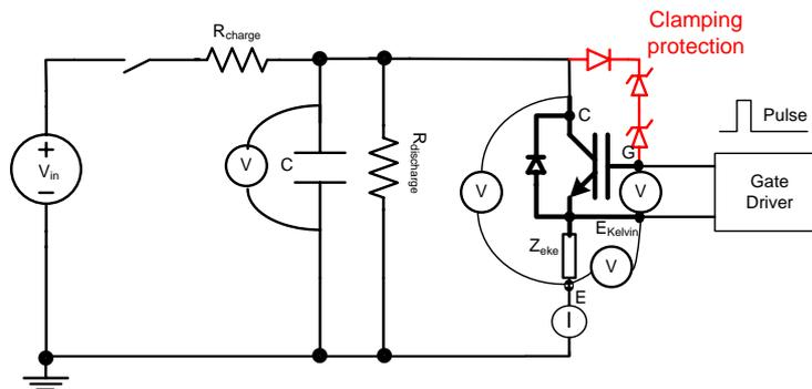
Figure D.11: Test setup for protection by clamping test.
