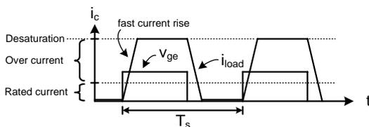
**Figure 5.1:** Desaturation by fast fault with small inductance. Desaturation occurs immediately after short circuit.
