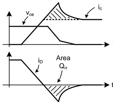
**Figure A.6:** Reverse recovery current through a diode and switch.
