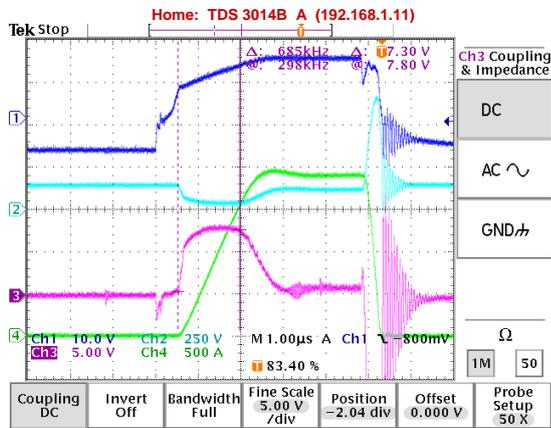
**Figure D.3:** Short circuit test for  $V_{in} = 150V$ . Dark blue =  $v_{ge}$ , light blue =  $v_{ce}$ , purple =  $v_{eke}$ , green =  $i_C$ .
