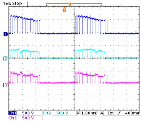
**Figure 9.21:** Voltage sharing of switch pair  $S_{b2}$ . Dark blue =  $v_{S_{b2}}$ , light blue =  $v_{S_{b21}}$ , purple =  $v_{S_{b22}}$ .
