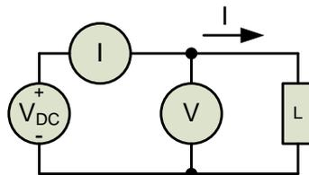
**Figure D.24:** *Resistance measurement test setup.*
