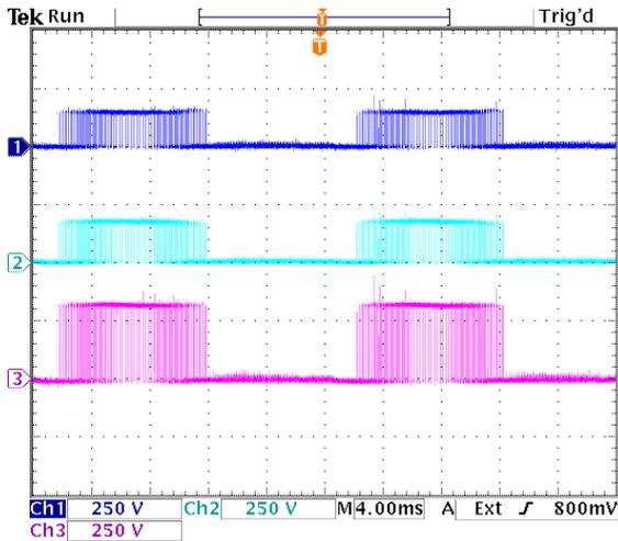
**Figure 9.13:** Voltage sharing of diode pair  $D_{b1}$ . Dark blue =  $v_{Db11}$ , light blue =  $v_{Db12}$ , purple =  $v_{Db1}$ .
