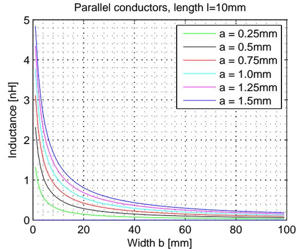
Figure C.4: Self inductance for two flat parallel wires according to equation (C.4).
