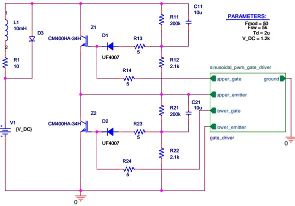
**Figure 4.42:** Simulation schematic for non ideal active gate control snubber.
