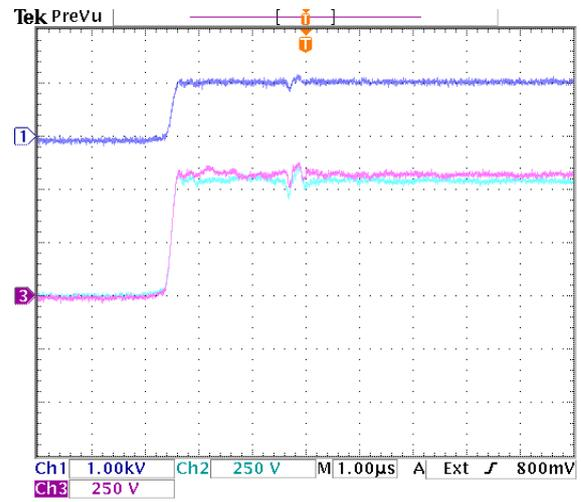
Figure 9.50: Zoom of turn off transition of diode pair  $D_{b1}$ . Dark blue =  $v_{D_{b1}}$ , light blue =  $v_{D_{b11}}$ , purple =  $v_{D_{b12}}$ .
