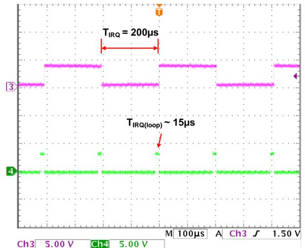
**Figure 7.19:** Measured IRQ parameters. Purple: IRQ period and green: IRQ execution time.
