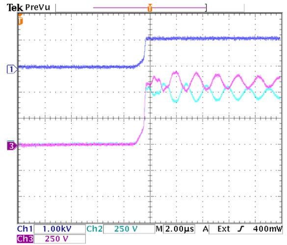
Figure 9.48: Zoom of turn off transition of switch pair  $S_{a4}$ . Dark blue =  $v_{S_{b4}}$ , light blue =  $v_{S_{b41}}$ , purple =  $v_{S_{b42}}$ .
