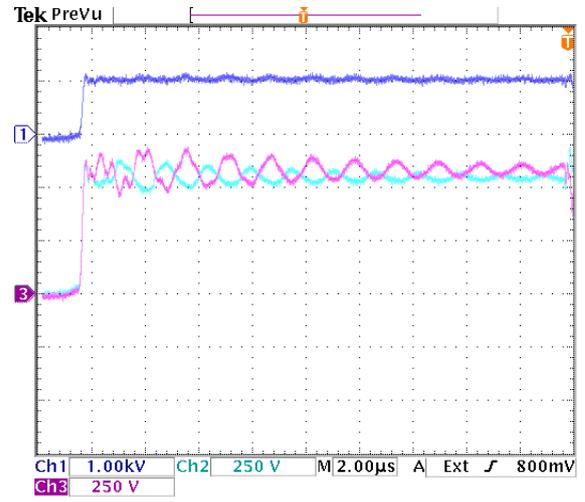
Figure 9.46: Zoom of turn off transition of switch pair  $S_{b3}$ . Dark blue =  $v_{S_{b3}}$ , light blue =  $v_{S_{b31}}$ , purple =  $v_{S_{b32}}$ .
