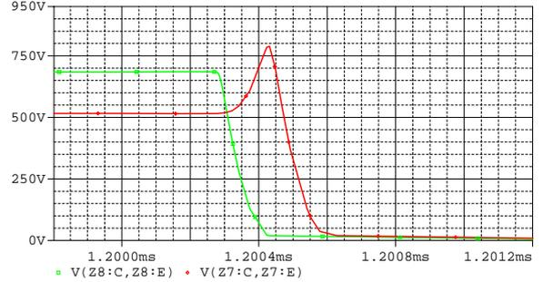
**Figure 3.13:** Turn on transition with added gate signal delay. See schematic in figure 3.5.
