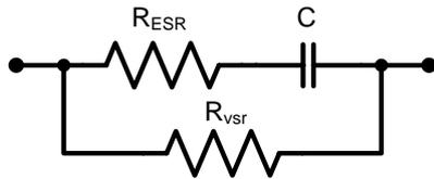
Figure 7.10: Capacitor circuit model.
