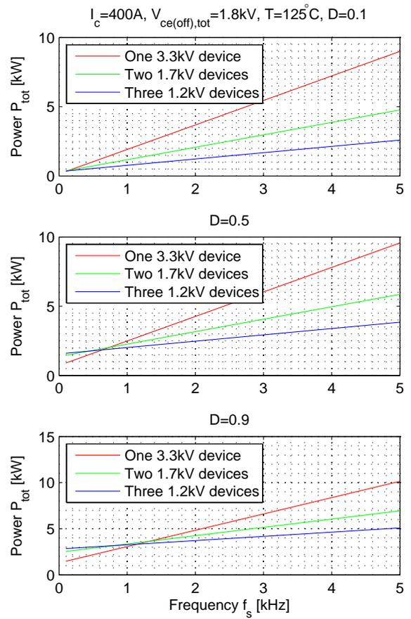
**Figure 3.15:** Total losses at  $T = 125^\circ\text{C}$  with duty cycle  $D = 0.1$ ,  $D = 0.5$  and  $D = 0.9$ .
