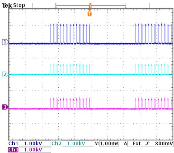
Figure 9.43: Voltage sharing of switch pair  $S_{b2}$ . Dark blue =  $v_{S_{b2}}$ , light blue =  $v_{S_{b21}}$ , purple =  $v_{S_{b22}}$ .
