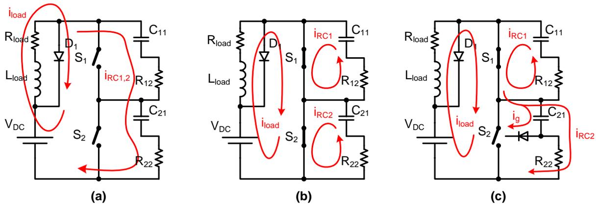
**Figure 4.36:** (a) Balanced off state, (b) Balanced on state and (c) Non balanced turn off transient. Switch  $S_2$  turns off earlier than  $S_1$ .
