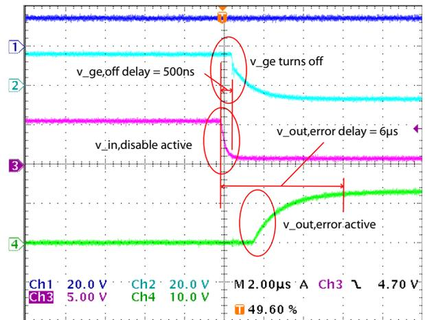
**Figure 7.30:** Zoom of gate driver signals with disable input active. Blue:  $v_{out,DSP}$ , magenta:  $v_{ge}$ , purple:  $v_{in,disable}$  and green:  $v_{out,error}$ .
