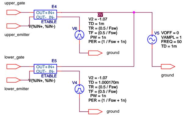
**Figure 4.43:** Simulation schematic for sinusoidal PWM circuit with  $t_d = 170ns$  and  $f_{mod} = 50Hz$ .
