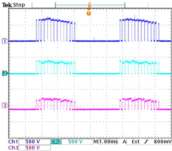
**Figure 9.18:** Voltage sharing of switch pair  $S_{a3}$ . Dark blue =  $v_{S_{a3}}$ , light blue =  $v_{S_{a31}}$ , purple =  $v_{S_{a32}}$ .
