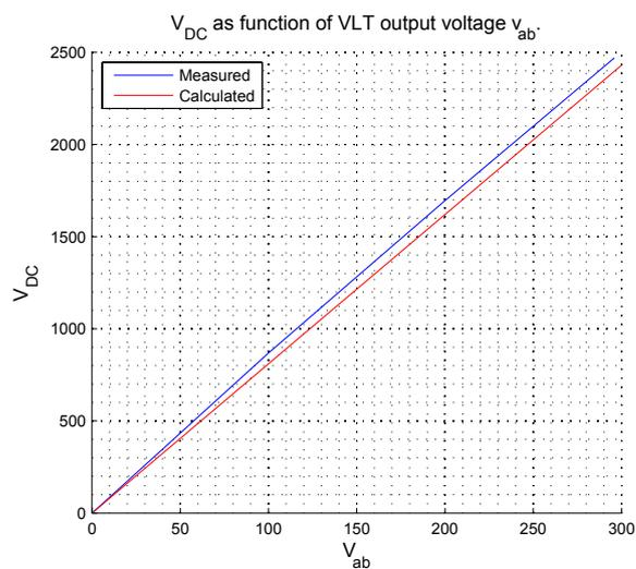
**Figure D.23:** DC link voltage as function of the VLT output. Equation (D.6) is plotted for reference (red).
