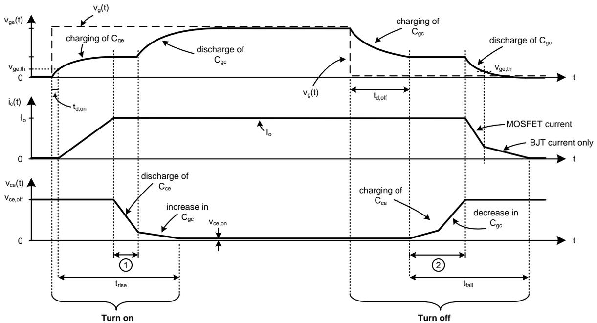
Figure A.4: Turn on and off waveforms for the IGBT.
