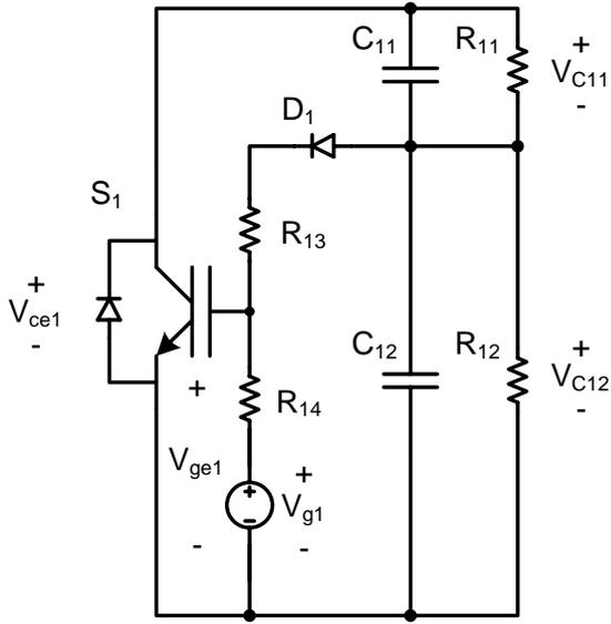
**Figure 4.34:** Schematic of one single active gate snubber.
