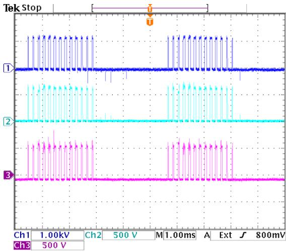
**Figure 9.33:** Voltage sharing of switch pair  $S_{b3}$ . Dark blue =  $v_{S_{a3}}$ , light blue =  $v_{S_{a31}}$ , purple =  $v_{S_{a32}}$ .
