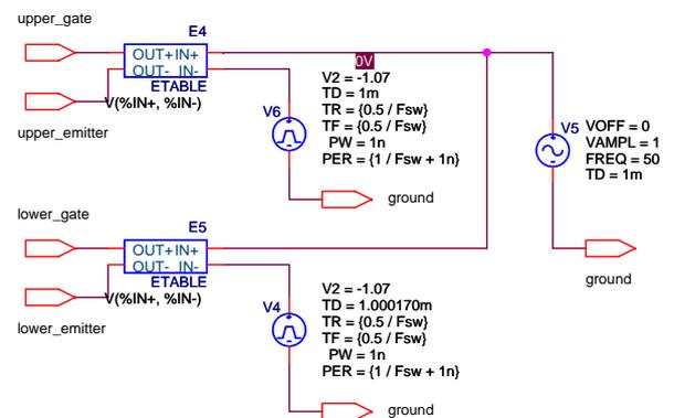
**Figure 4.38:** Simulation schematic for sinusoidal PWM circuit with  $t_d = 170ns$  and  $f_{mod} = 50Hz$ .
