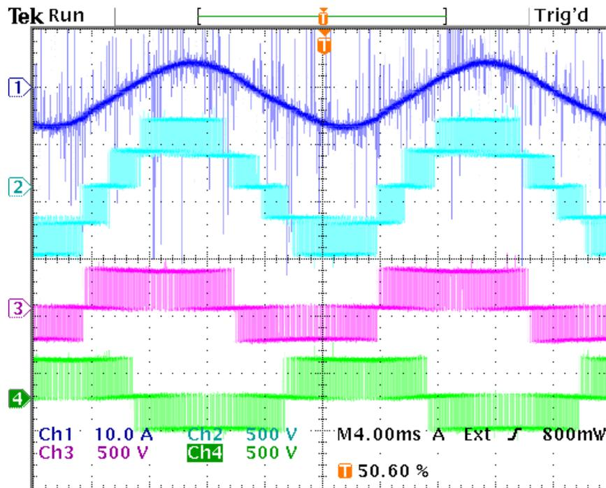
**Figure 9.2:** Output waveforms for initial test. Dark blue =  $i_{load}$ , light blue =  $v_{ab}$ , purple =  $v_{aN}$  and green =  $v_{bN}$ .
