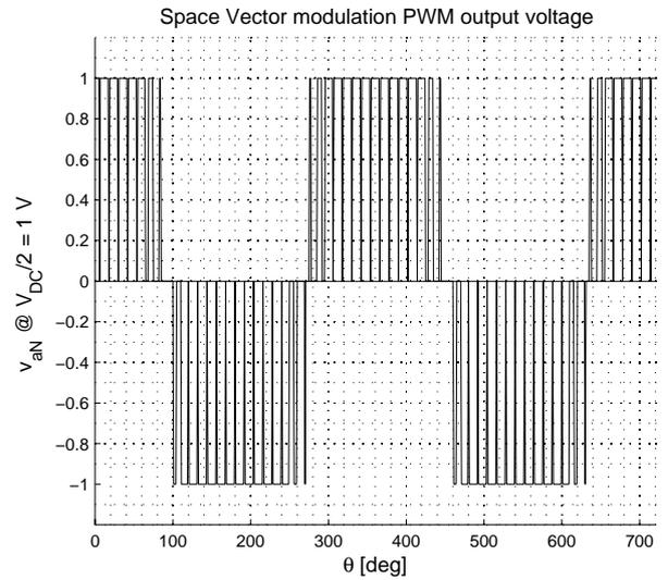
**Figure 2.13:** PWM output voltage for space vector modulation.
