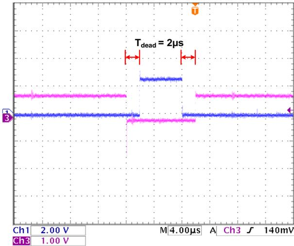
**Figure 7.18:** Measured dead time  $t_{dead} = 2\mu s$  on DSP output. Blue: switch A1, purple: switch A3. The voltage levels and offset is shifted slightly for clarity.
