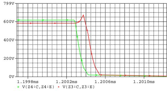
**Figure 3.9:** Turn on transition with added gate emitter capacitance. See schematic in figure 3.3.
