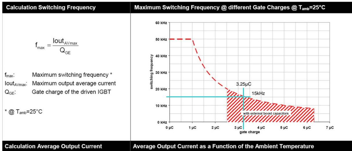
**Figure 7.21:** Maximum rating for output charge per pulse [Semikron, 2007a].
