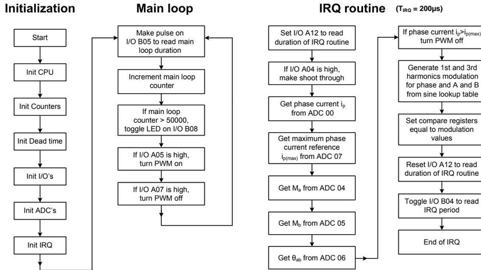
Figure 7.14: Flow chart of the DSP code.
