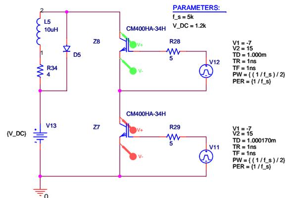
**Figure 3.5:** Schematic with added gate signal delay  $TD = 170ns$  in the gate signal source  $V_{11}$ . Results are shown in figures 3.12 and 3.13.
