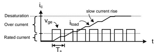
**Figure 5.2:** Desaturation by slow fault with large inductance. Desaturation occurs after a sequence of switching periods.
