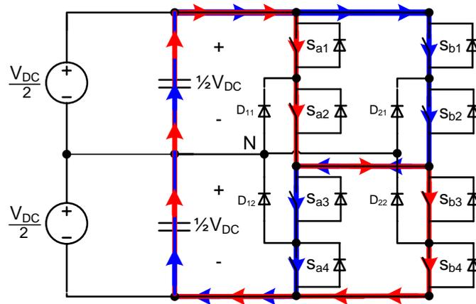
**Figure 9.54:** Schematic of short circuit test. The red line is the current path for test 1, and the blue line is the current path for test 2.
