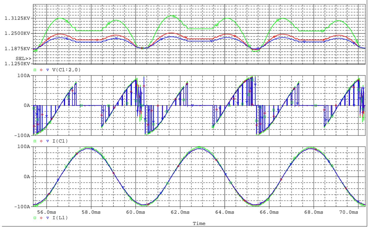
**Figure D.26:** Initial simulation results. The colors represents: green =  $400\mu F$ , red =  $825\mu F$  and blue =  $1100\mu F$ . The top graph shows the voltage across the top DC link capacitor, the middle shows the capacitor current and the bottom graph shows the load current.
