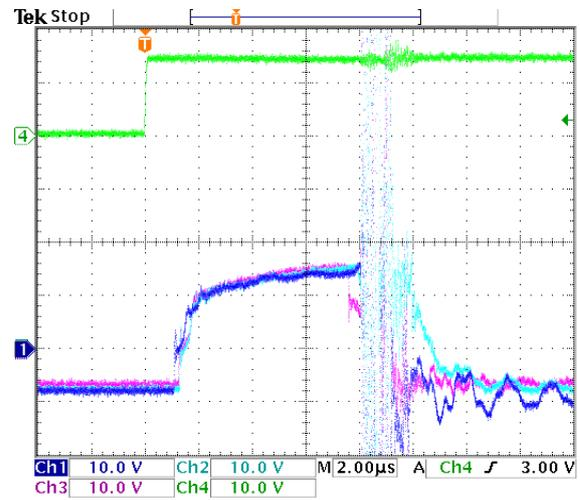
**Figure 9.60:** Gate signals of short circuit test 1. Dark blue =  $v_{ge,Sb32}$ , light blue =  $v_{ge,Sb41}$ , purple =  $v_{ge,Sb42}$ , green = gate trigger signal.
