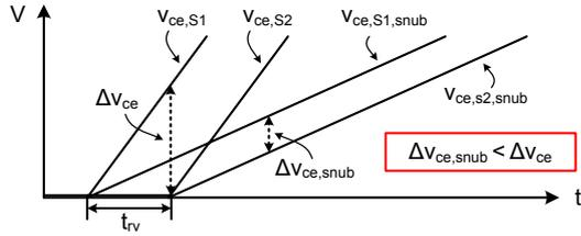
**Figure 4.10:** Voltage waveforms in turn off transient with and without snubber.
