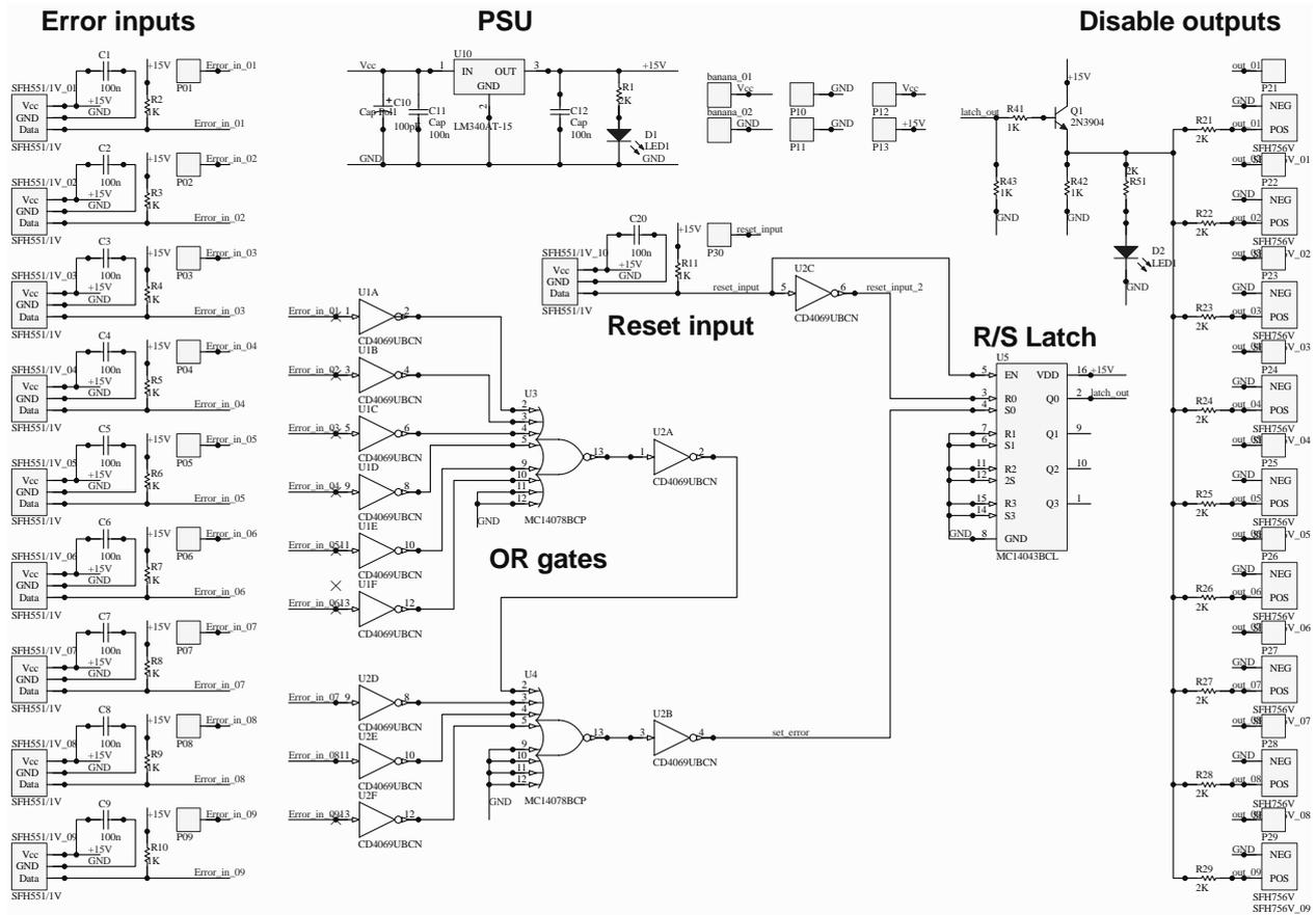
Figure 7.32: Schematic of the optical hub used for fast fault protection.
