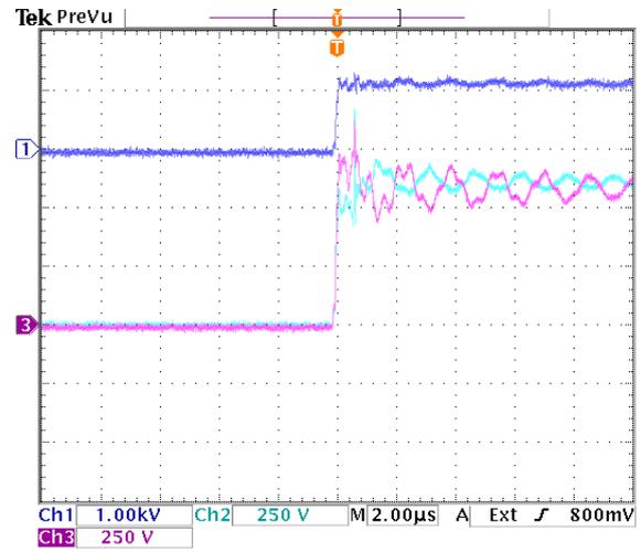
**Figure 9.34:** Zoom of turn off transition of switch pair  $S_{a3}$ . Dark blue =  $v_{S_{a3}}$ , light blue =  $v_{S_{a31}}$ , purple =  $v_{S_{a32}}$ .
