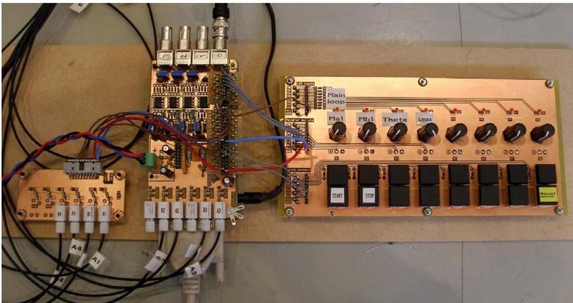
**Figure 7.13:** Picture of DSP board, extension I/O board and extra optical transmitters.
