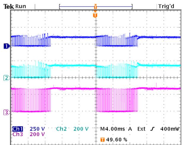
**Figure 9.6:** Voltage sharing of switch pair  $S_{a4}$ . Dark blue =  $v_{Sa41}$ , light blue =  $v_{Sa42}$ , purple =  $v_{Sa4}$ .
