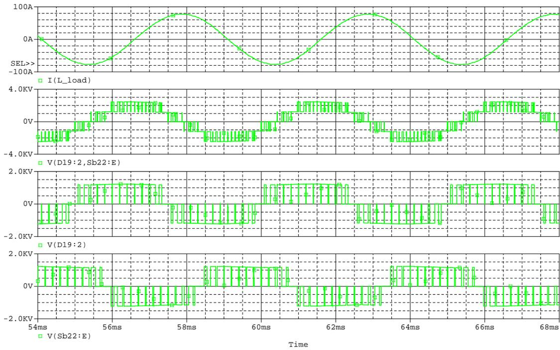
**Figure 8.2:** Simulated output waveforms. From the top: (1) Load current  $i_{load}$ ; (2) phase to phase voltage  $v_{ab}$ ; (3) phase a to neutral point voltage  $v_{aN}$ ; and bottom (4) phase b to neutral point voltage  $v_{bN}$ .
