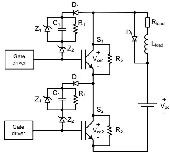
**Figure 4.6:** Voltage clamping by two zener diodes and an RC network [N.Y.A. Shamma & Chamud, February 2006].
