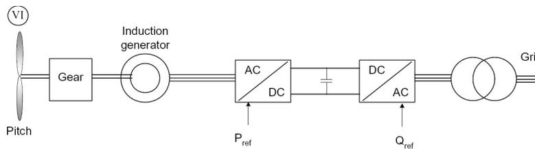
**Figure 1.3:** *Electrical system in a turbine with squirrel cage induction generator [Blaabjerg, 2006].*
