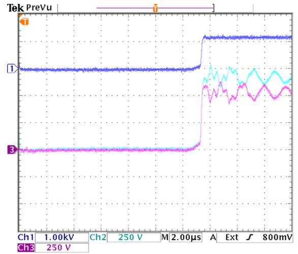
**Figure 9.32:** Zoom of turn off transition of switch pair  $S_{a2}$ . Dark blue =  $v_{Sa2}$ , light blue =  $v_{Sa21}$ , purple =  $v_{Sa22}$ .
