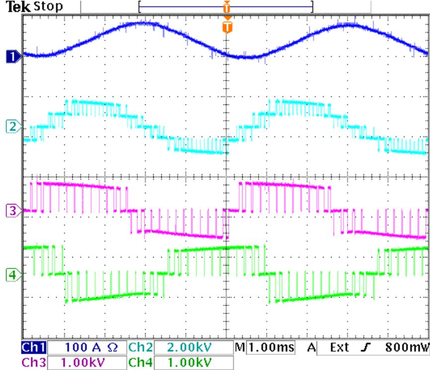
**Figure 9.15:** Output waveforms for 1.2kV test. Dark blue =  $i_{load}$ , light blue =  $v_{ab}$ , purple =  $v_{aN}$  and green =  $v_{bN}$ . Notice the offset in the current.
