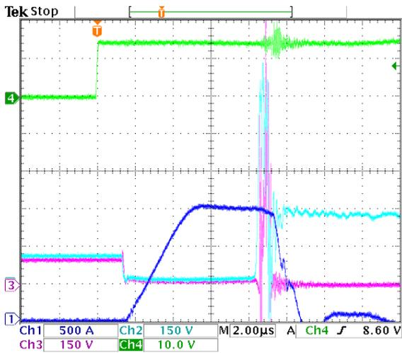
**Figure 9.61:** Short circuit test 2. Dark blue =  $i_{load}$ , light blue =  $v_{ce,Sb11}$ , purple =  $v_{ce,Sb12}$ , green = gate trigger signal.
