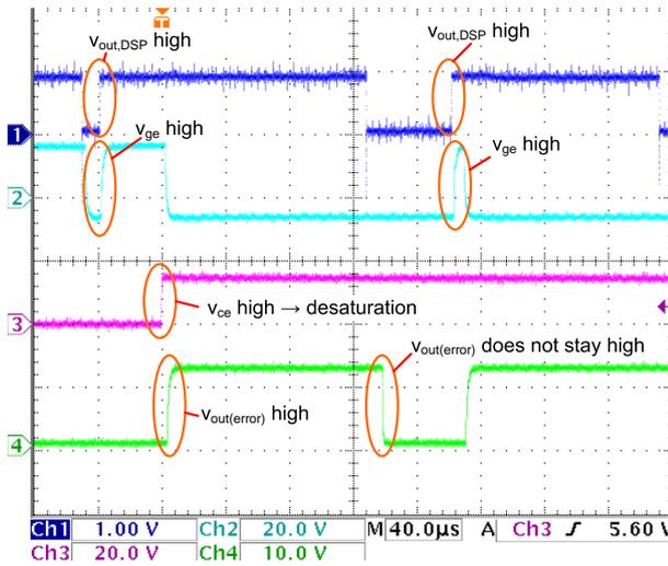
**Figure 7.27:** Measured gate driver signals in desaturation situation. Blue:  $v_{out,DSP}$ , magenta:  $v_{ge}$ , purple:  $v_{ce}$  and green:  $v_{out,error}$ .
