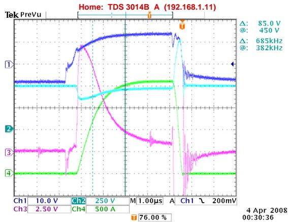
Figure D.7: Short circuit test for  $V_{in} = 500V$ . Dark blue =  $v_{ge}$ , light blue =  $v_{ce}$ , purple =  $v_{eke}$ , green =  $i_C$ .
