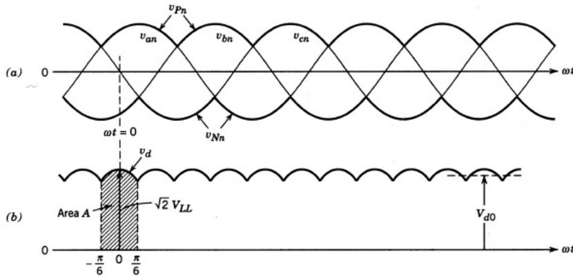
Figure D.15: Three phase rectifier voltages. [Ned Mohan, 2003]
