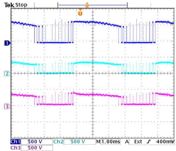
**Figure 9.19:** Voltage sharing of switch pair  $S_{a4}$ . Dark blue =  $v_{S_{a4}}$ , light blue =  $v_{S_{a41}}$ , purple =  $v_{S_{a42}}$ .
