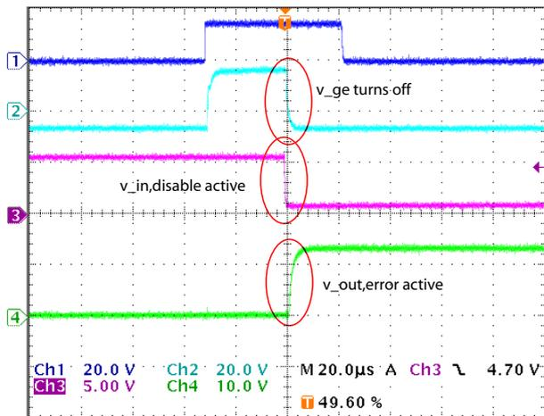
**Figure 7.29:** Measured gate driver signals with disable input active. Blue:  $v_{out,DSP}$ , magenta:  $v_{ge}$ , purple:  $v_{in,disable}$  and green:  $v_{out,error}$ .
