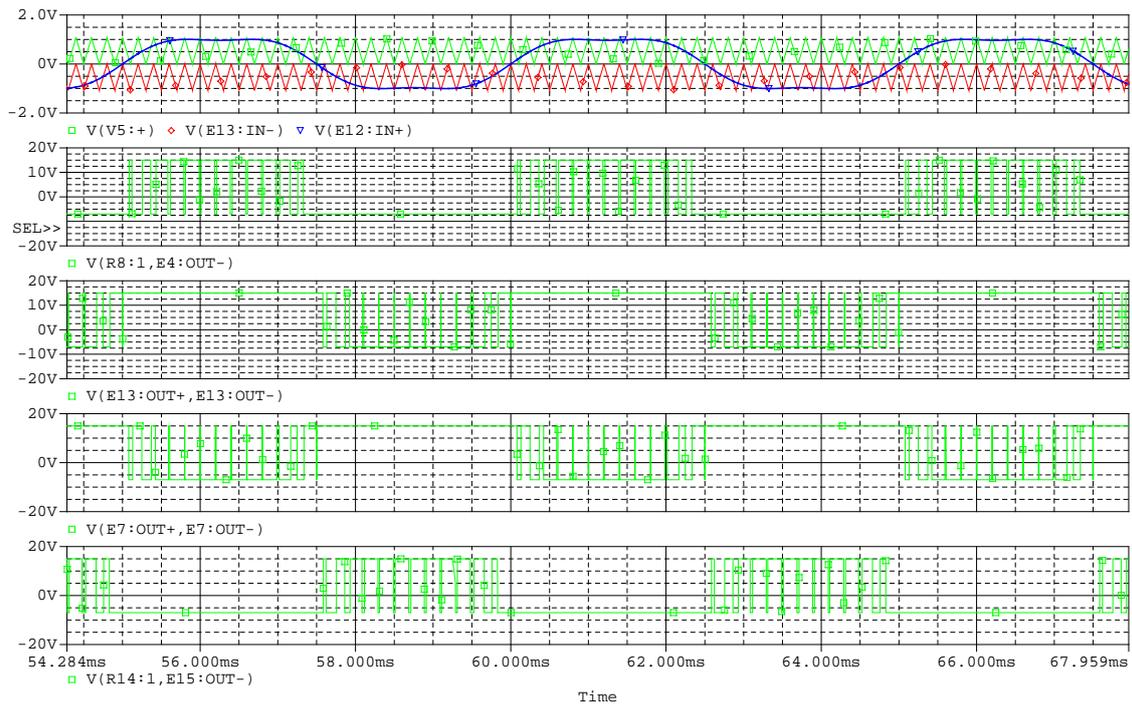
**Figure 8.3:** Gate signals for phase a. From the top: (1) Modulation signals green=upper triangle, red lower triangle and blue modulation with third harmonic injection. (2)  $v_{ge}$  for  $S_{a11}, S_{a12}$ . (3)  $v_{ge}$  for  $S_{a21}, S_{a22}$ . (4)  $v_{ge}$  for  $S_{a31}, S_{a32}$  and bottom (5)  $v_{ge}$  for  $S_{a41}, S_{a42}$ .
