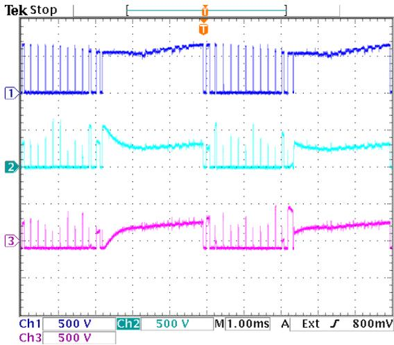
**Figure 9.16:** Voltage sharing of switch pair  $S_{a1}$ . Dark blue =  $v_{S_{a1}}$ , light blue =  $v_{S_{a11}}$ , purple =  $v_{S_{a12}}$ .
