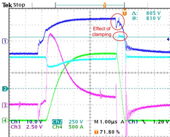
**Figure 5.18:** Short circuit test with added clamping protection for  $V_{in} = 500V$ . Dark blue =  $v_{ge}$ , light blue =  $v_{ce}$ , purple =  $v_{eke}$  and green =  $i_c$ .
