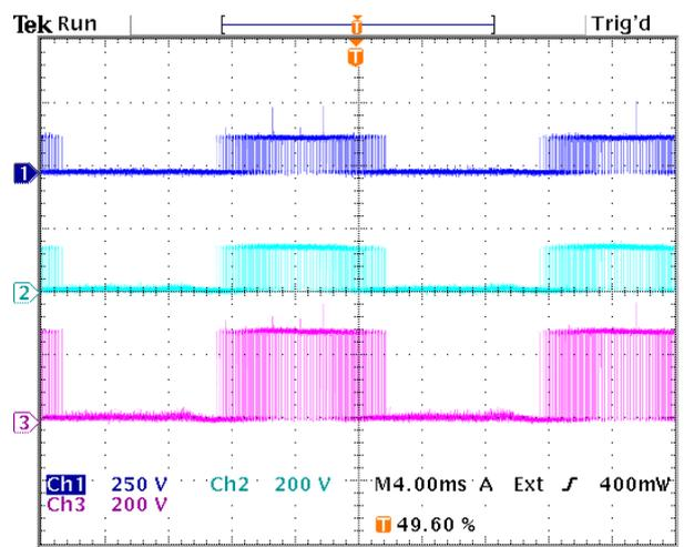
**Figure 9.14:** Voltage sharing of diode pair  $D_{b2}$ . Dark blue =  $v_{Db21}$ , light blue =  $v_{Db22}$ , purple =  $v_{Db2}$ .
