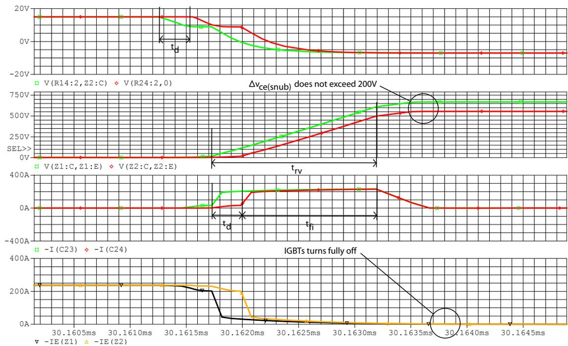
**Figure 4.16:** Simulation of off transition of passive snubber for series connected IGBTs. (1)  $v_{ge1}$  and  $v_{ge2}$ , (2)  $v_{ce,Z1}$  and  $v_{ce,Z2}$ , (3)  $i_{Cs1}$  and  $i_{Cs2}$  and (4)  $i_{c,Z1}$  and  $i_{c,Z2}$ .
