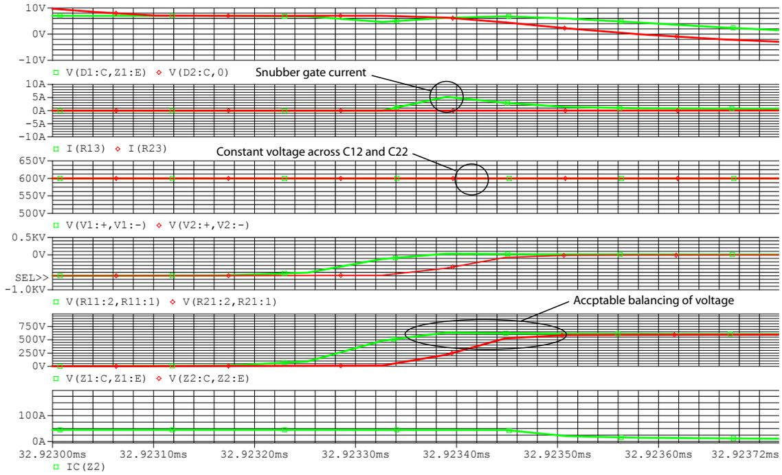
**Figure 4.41:** Zoom in of simulation of an off transition by the ideal active gate control (constant voltage across  $C_{11}$  and  $C_{21}$ ). (1)  $v_{ge1}$  and  $v_{ge2}$ , (2)  $i_{R13}$  and  $i_{R23}$ , (3)  $v_{C12}$  and  $v_{C22}$ , (4)  $v_{R11}$  and  $v_{R21}$ , (5)  $v_{ce,Z1}$  and  $v_{ce,Z2}$  and (6)  $i_{c,Z1}$ .
