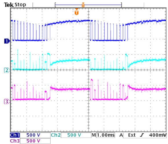
**Figure 9.23:** Voltage sharing of switch pair  $S_{b4}$ . Dark blue =  $v_{S_{b4}}$ , light blue =  $v_{S_{b41}}$ , purple =  $v_{S_{b42}}$ .
