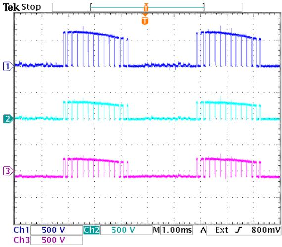
**Figure 9.24:** Voltage sharing of diode pair  $D_{a1}$ . Dark blue =  $v_{D_{a1}}$ , light blue =  $v_{D_{a11}}$ , purple =  $v_{D_{a12}}$ .
