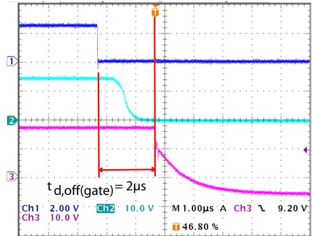
**Figure 7.26:** Measured gate driver signals in turn off transition. Blue:  $v_{out,DSP}$ , magenta:  $v_{in,gate}$  and purple:  $v_{ge}$ .
