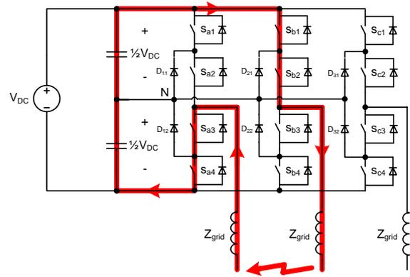
**Figure 5.4:** Slow fault with phase to phase short circuit. Characterized by slow current rise.
