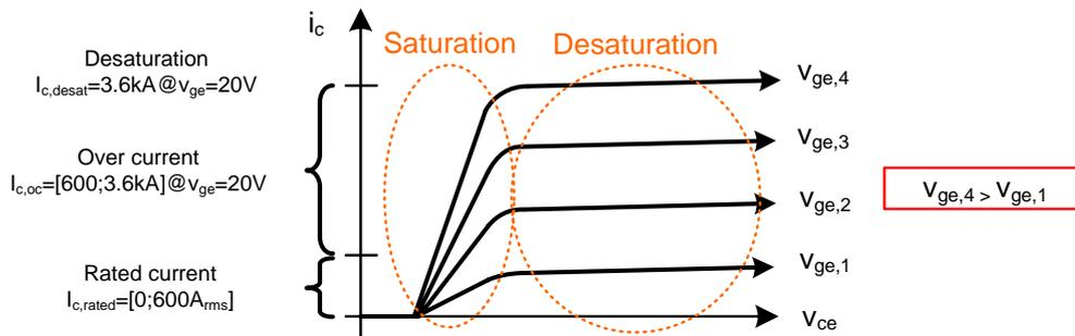
**Figure 5.5:**  $i/v$  characteristic under fault conditions for the Semikron IGBT.
