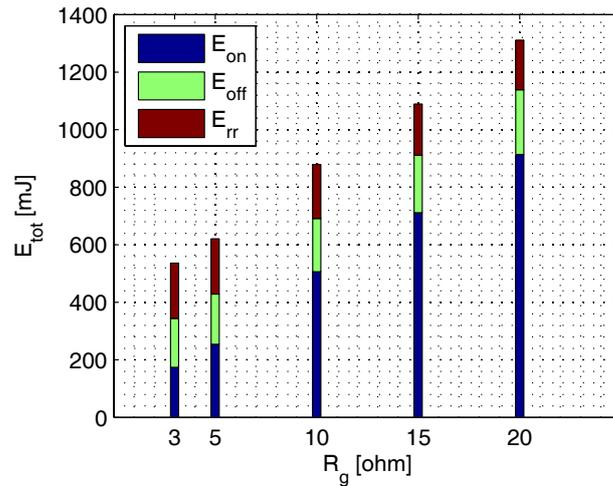
**Figure A.9:** Estimate of sum of turn on, turn off and reverse recovery loss energy for one single transition estimated for  $I_c = 400A$  and  $V_{ce,off} = 1.2kV$ .
