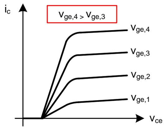
**Figure A.3:** Output characteristics for the n-channel IGBT.
