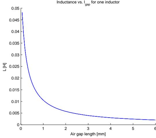
**Figure 7.7:** Inductance for one inductor as function of  $l_{gap}$ .
