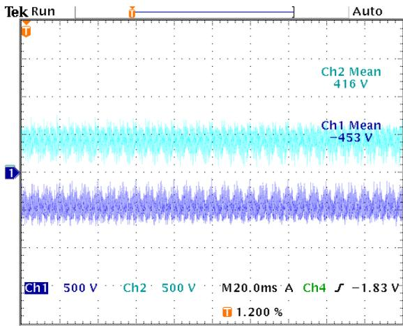
Figure D.20: DC link voltage for  $V_{ab} = 100V$ .
