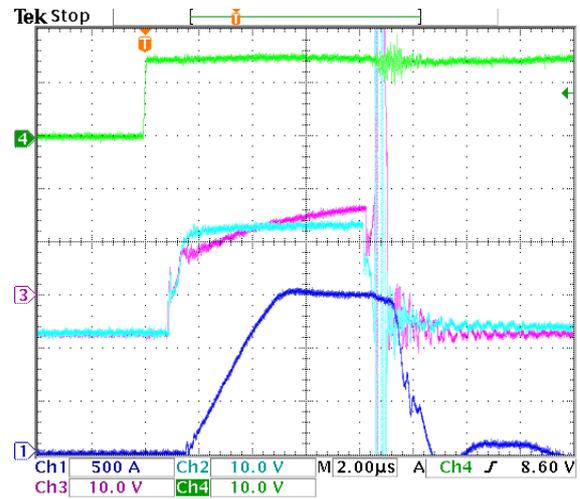
**Figure 9.62:** Gate signals of short circuit test 2. Dark blue =  $i_{load}$ , light blue =  $v_{ge,Sb11}$ , purple =  $v_{ge,Sb12}$ , green = gate trigger signal.
