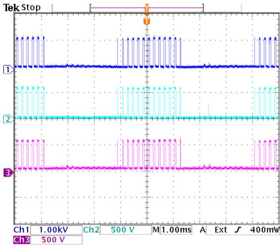
**Figure 9.39:** Voltage sharing of diode pair  $D_{a2}$ . Dark blue =  $v_{Da2}$ , light blue =  $v_{Da21}$ , purple =  $v_{Da22}$ .
