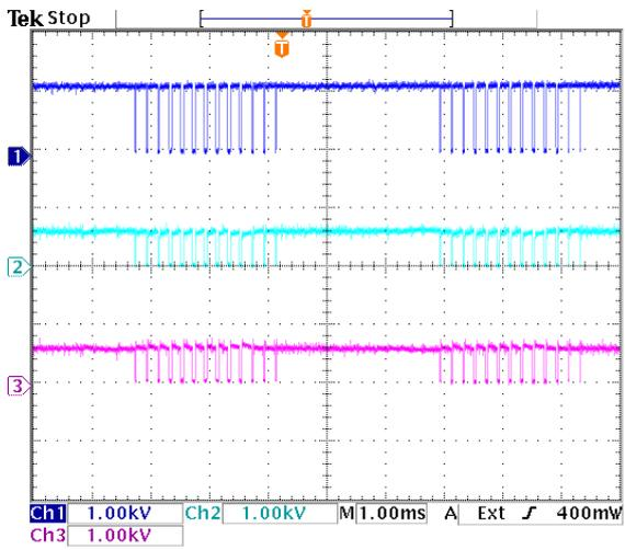
Figure 9.41: Voltage sharing of switch pair  $S_{b1}$ . Dark blue =  $v_{S_{b1}}$ , light blue =  $v_{S_{b11}}$ , purple =  $v_{S_{b12}}$ .
