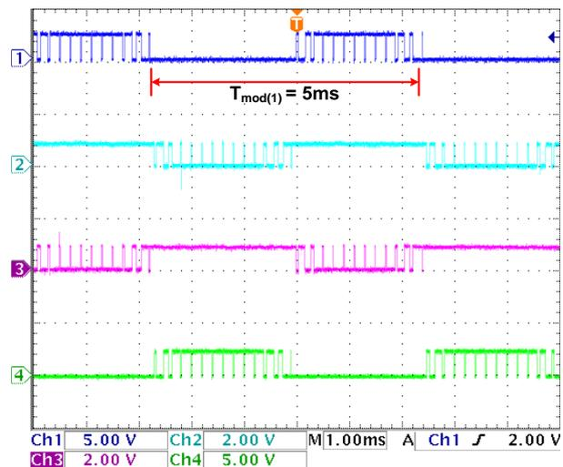
**Figure 7.17:** Measured PWM signals for phase B. From the top:  $B_1$  to  $B_4$ .
