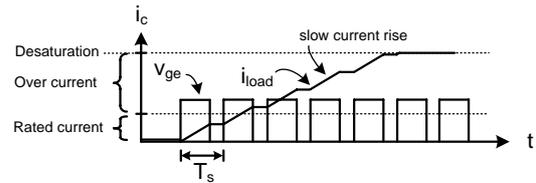
**Figure B.2:** Desaturation by slow fault with large inductance. Desaturation occurs after a sequence of switching periods.
