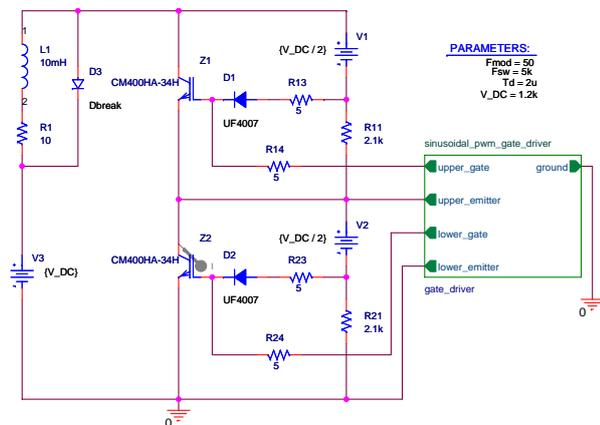
**Figure 4.37:** Simulation schematic for ideal active gate control snubber.
