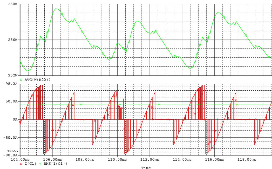
Figure 7.12: Simulation results for power dissipation caused by the  $R_{ESR}$  of  $0.156\Omega$ . The top graph show the average power dissipation, and the bottom graph shows the capacitor current (red), and the RMS capacitor current (green).
