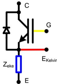
**Figure 5.9:** Schematic view of the impedance  $Z_{ek_e}$  impedance.
