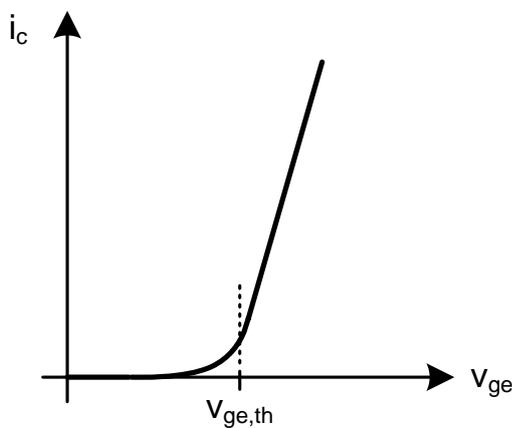
**Figure A.2:** Transfer characteristic for an n-channel IGBT.
