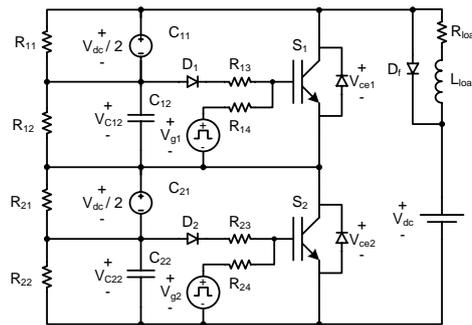
Figure 4.26: Schematic of the balancing circuit for two switches.
