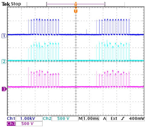
**Figure 9.29:** Voltage sharing of switch pair  $S_{a1}$ . Dark blue =  $v_{Sa1}$ , light blue =  $v_{Sa11}$ , purple =  $v_{Sa12}$ .
