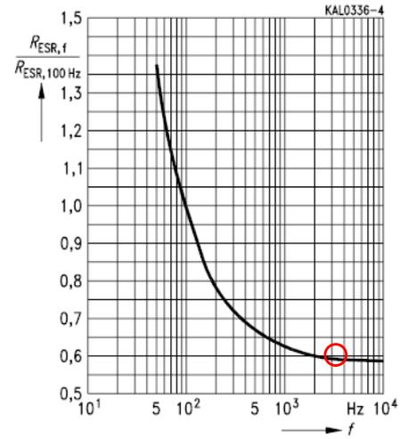
Figure 7.11:  $R_{ESR}$  versus frequency from capacitor data sheet [Siemens, -]. Red circle shows relative  $R_{ESR}$  at  $f = 5\text{kHz}$ .
