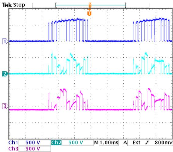
**Figure 9.22:** Voltage sharing of switch pair  $S_{b3}$ . Dark blue =  $v_{S_{b3}}$ , light blue =  $v_{S_{b31}}$ , purple =  $v_{S_{b32}}$ .
