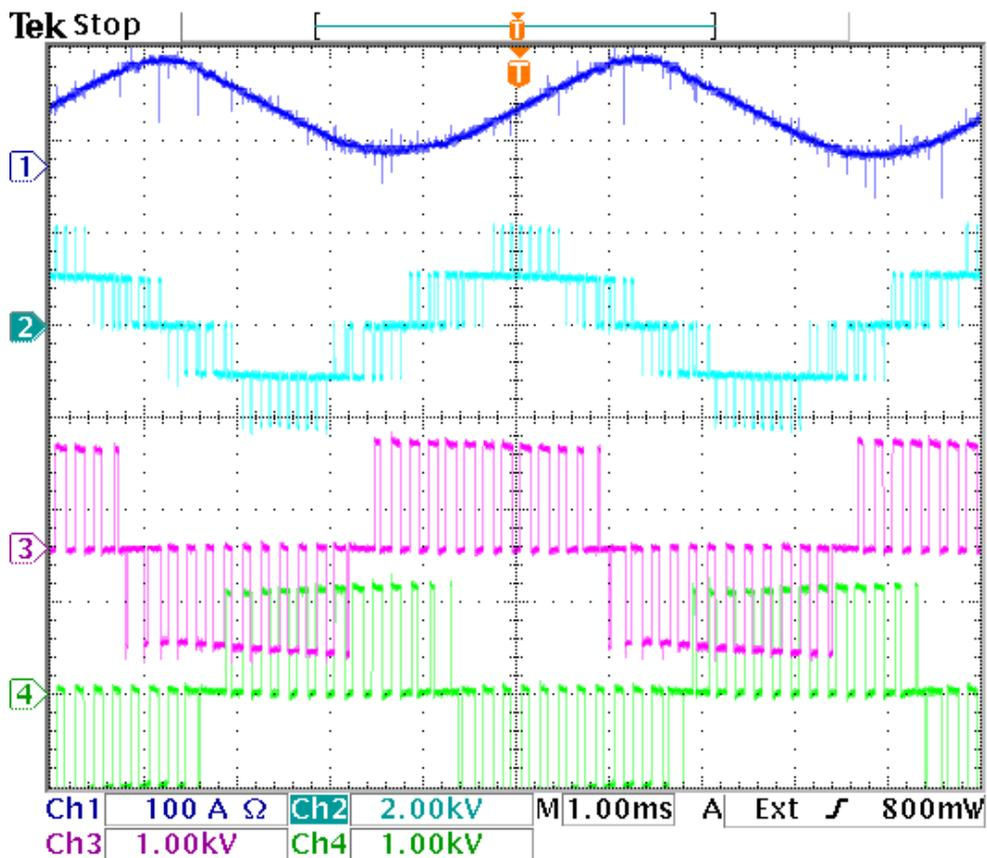
Figure 9.28: Output waveforms for final test. Dark blue =  $i_{load}$ , light blue =  $v_{ab}$ , purple =  $v_{aN}$  and green =  $v_{bN}$ .
