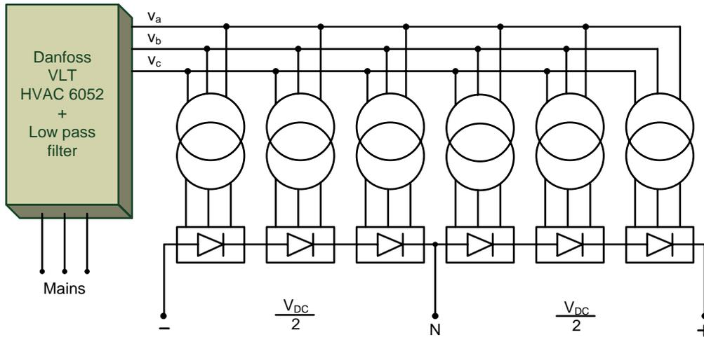
**Figure 7.2:** *Medium voltage DC supply schematic.*
