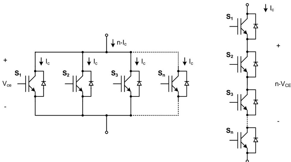
**Figure 3.16:** IGBTs in parallel (left) and series connections (right).
