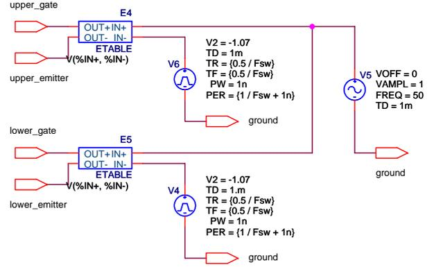
**Figure 4.19:** Simulation schematic for sinusoidal PWM circuit.
