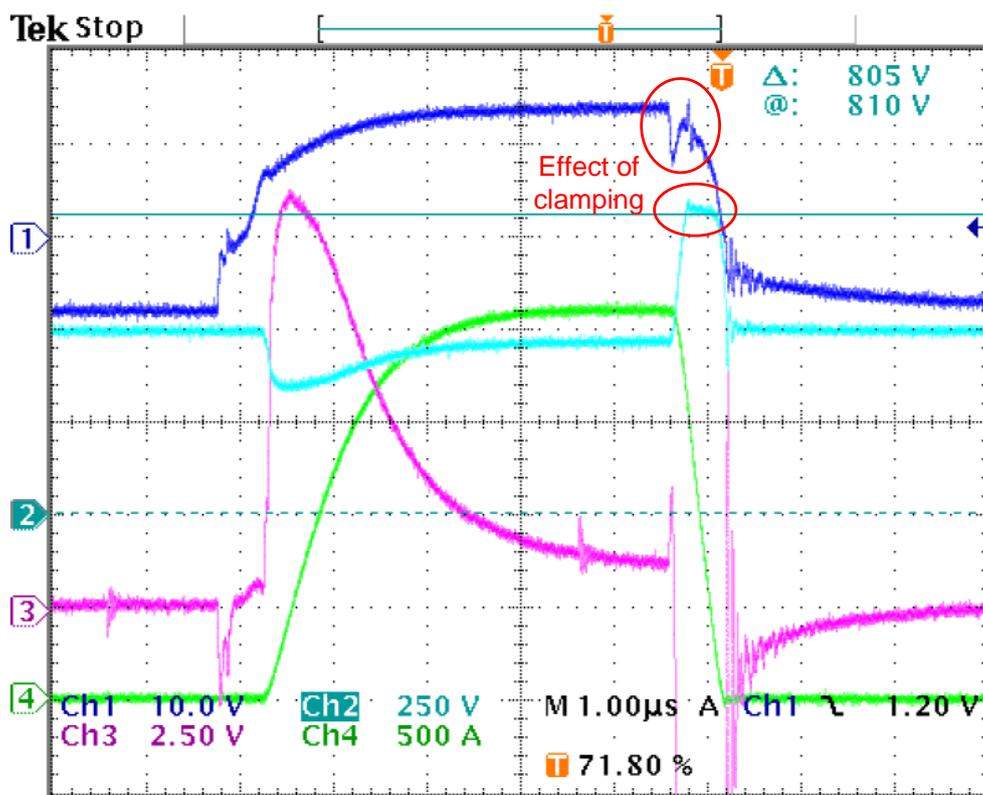
**Figure D.12:** Short circuit test for  $V_{in} = 500V$  with added clamping protection. Dark blue =  $v_{ge}$ , light blue =  $v_{ce}$ , purple =  $v_{ke}$ , green =  $i_c$ .
