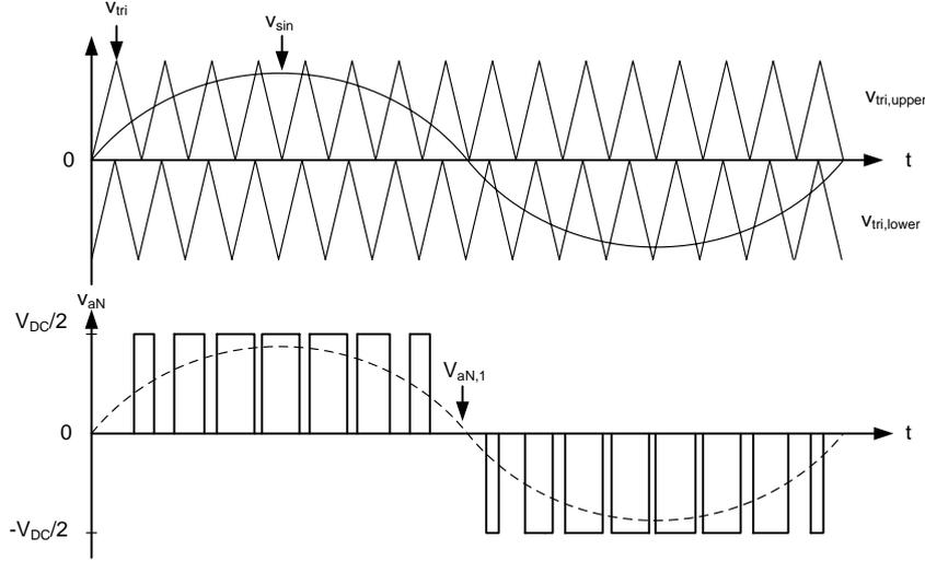
**Figure 2.7:** Carrier based modulation scheme for three-level inverter. Top graph shows the modulation and carrier waveform and bottom graph is the generated output voltage pr. leg for a three-level inverter, and the first harmonic (dotted) waveform  $v_{aN,1}$ .
