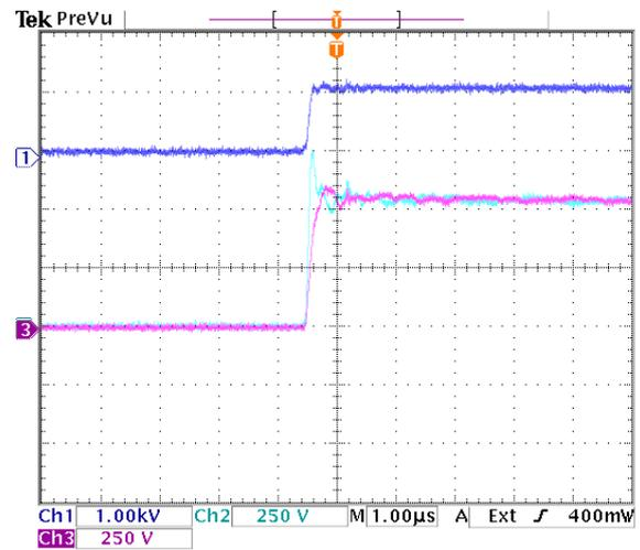
Figure 9.52: Zoom of turn off transition of diode pair  $D_{b2}$ . Dark blue =  $v_{D_{b2}}$ , light blue =  $v_{D_{b21}}$ , purple =  $v_{D_{b22}}$ .
