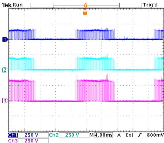
Figure 9.9: Voltage sharing of switch pair  $S_{b3}$ . Dark blue =  $v_{S_{b31}}$ , light blue =  $v_{S_{b32}}$ , purple =  $v_{S_{b3}}$ .
