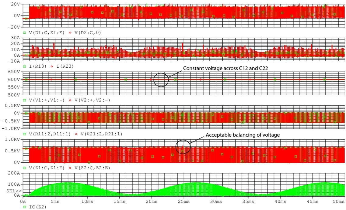
**Figure 4.39:** Simulation of the ideal active gate control with constant voltage across  $C_{11}$  and  $C_{21}$ . (1)  $v_{ge1}$  and  $v_{ge2}$ , (2)  $i_{R13}$  and  $i_{R23}$ , (3)  $v_{C12}$  and  $v_{C22}$ , (4)  $v_{R11}$  and  $v_{R21}$ , (5)  $v_{ce,Z1}$  and  $v_{ce,Z2}$  and (6)  $i_{c,Z1}$ .
