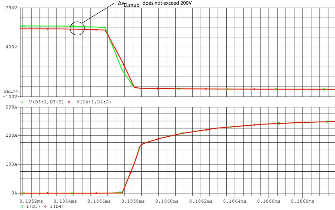
**Figure 4.24:** Simulation of on transition of passive snubber for series connected diodes. (1)  $v_{D3}$  and  $v_{D4}$ , (2)  $i_{D3}$  and  $i_{D4}$ .
