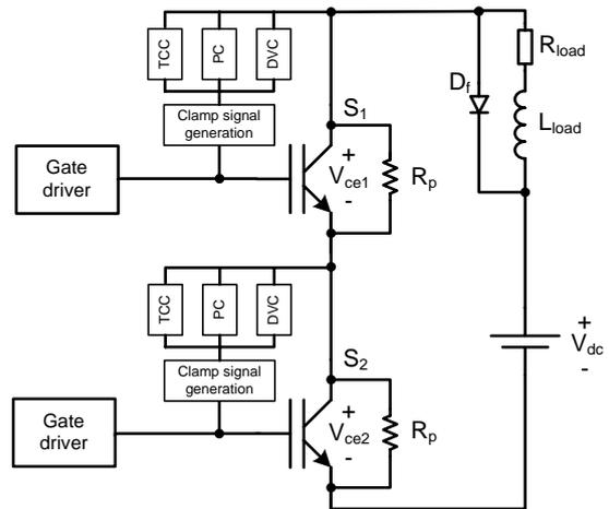
**Figure 4.8:** Multi level voltage clamping [N.Y.A. Shamma & Chamud, February 2006].
