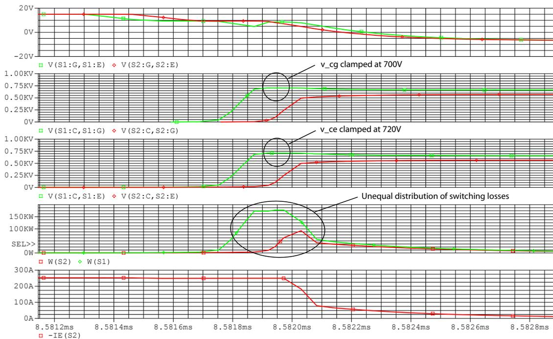
**Figure 4.53:** Zoom in of simulation of an off transition by the zener clamped snubber. (1)  $v_{ge1}$  and  $v_{ge2}$ , (2)  $v_{cg1}$  and  $v_{cg2}$ , (3)  $v_{ce1}$  and  $v_{ce2}$ , (4)  $W_{S1}$  and  $W_{S2}$  and (5)  $i_{c,S2}$ .
