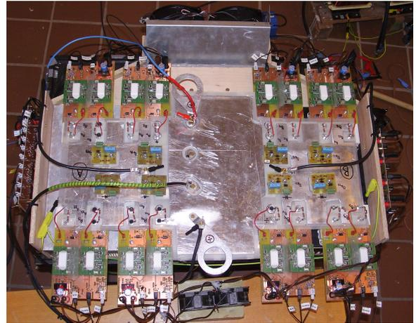
**Figure 8.11:** Layer five: Static voltage sharing resistors, fiber optical connections, diode snubbers and optical hub.
