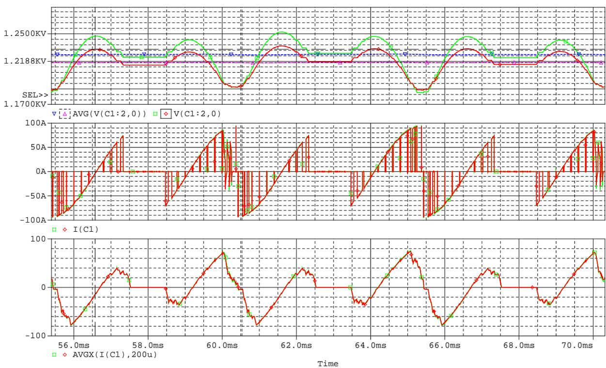
**Figure D.27:** Initial simulation results. The colors represents: green/blue =  $825\mu F$  and red/purple =  $1100\mu F$ . The top graph shows the voltage across the top DC link capacitor (red/green) together with the DC value of the voltage (blue/purple). The middle graph shows the capacitor current (red/green). The bottom graph shows the average waveform of the capacitor current (blue/purple).
