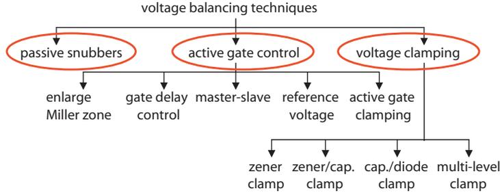
**Figure 4.1:** Classification of different voltage balancing methods for series connected semiconductors [N.Y.A. Shamas & Chamud, February 2006].
