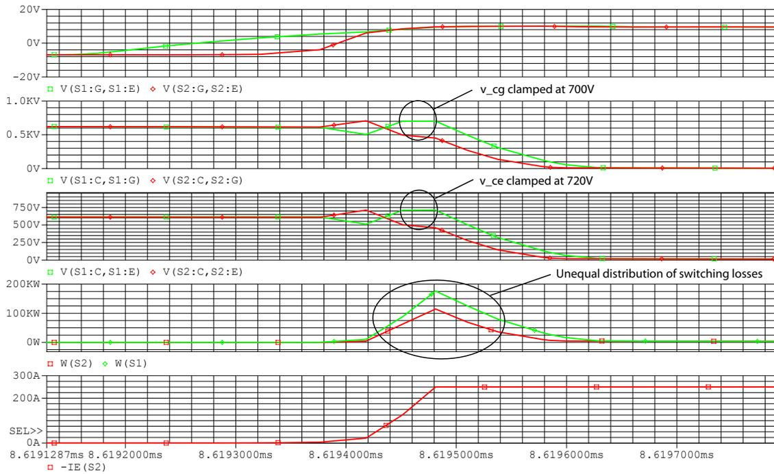
**Figure 4.52:** Zoom in of simulation of an on transition by the zener clamped snubber. (1)  $v_{ge1}$  and  $v_{ge2}$ , (2)  $v_{cg1}$  and  $v_{cg2}$ , (3)  $v_{ce1}$  and  $v_{ce2}$ , (4)  $W_{S1}$  and  $W_{S2}$  and (5)  $i_{c,S2}$ .
