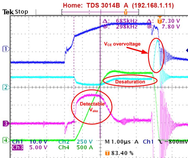
**Figure 5.11:** Short circuit test for  $V_{in} = 150V$ . Dark blue =  $v_{ge}$ , light blue =  $v_{ce}$ , purple =  $v_{ek_e}$ , green =  $i_c$ .
