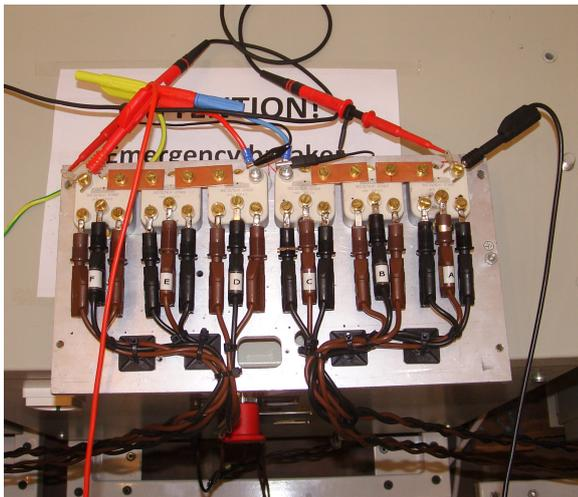
Figure D.17: Diode bridge rectifier and high voltage probes.
