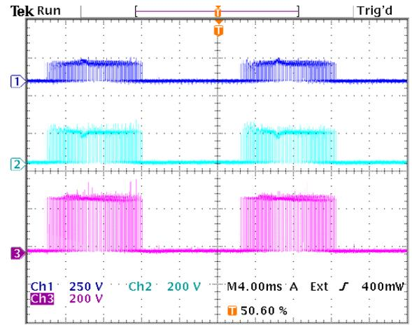
**Figure 9.4:** Voltage sharing of switch pair  $S_{a2}$ . Dark blue =  $v_{Sa21}$ , light blue =  $v_{Sa22}$ , purple =  $v_{Sa2}$ .
