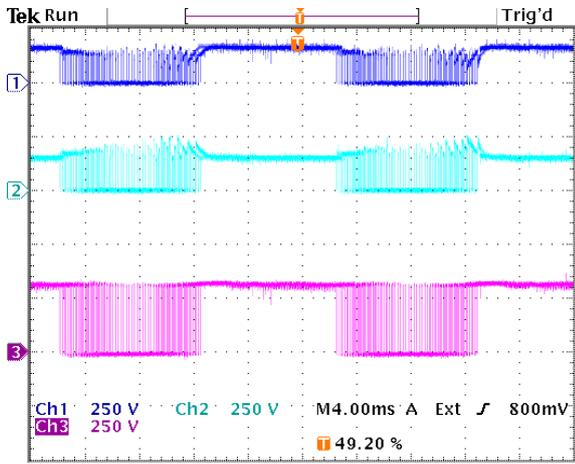
**Figure 9.3:** Voltage sharing of switch pair  $S_{a1}$ . Dark blue =  $v_{Sa11}$ , light blue =  $v_{Sa12}$ , purple =  $v_{Sa1}$ .
