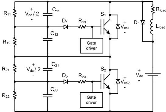
**Figure 4.3:** Active gate control by closed loop feedback with passive components [N.Y.A. Shamma & Chamud, February 2006].
