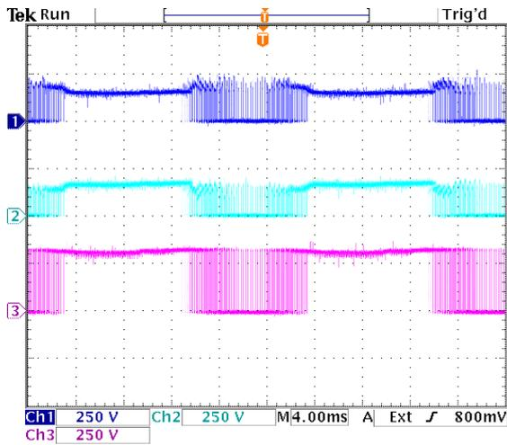
Figure 9.7: Voltage sharing of switch pair  $S_{b1}$ . Dark blue =  $v_{S_{b11}}$ , light blue =  $v_{S_{b12}}$ , purple =  $v_{S_{b1}}$ .
