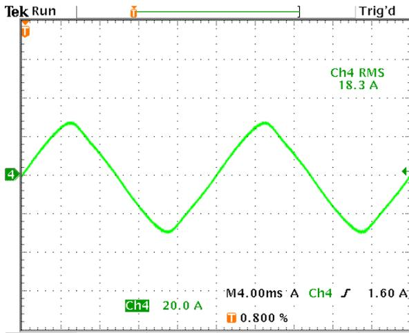
**Figure 7.5:** Measured current for one inductor. Notice, that the waveform becomes quasi triangular because it is near saturation.
