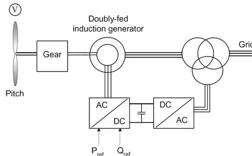
**Figure 1.4:** *Electrical system in a turbine with doubly fed induction generator [Blaabjerg, 2006].*
