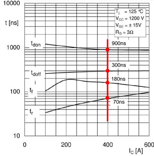
**Figure A.10:** Rise and fall times as function of collector current  $I_c$  for the SKM600GA176D with  $R_g = 3\Omega$  and  $v_{ce} = 1.2kV$  [Semikron, 2006].
