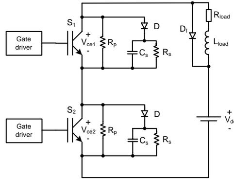
**Figure 4.2:** Schematic of two series connected IGBTs with passive snubbers.
