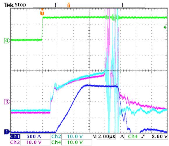
**Figure 9.56:** Gate signals of short circuit test 1. Dark blue =  $i_{load}$ , light blue =  $v_{ge,Sa11}$ , purple =  $v_{ge,Sa12}$ , green = gate trigger signal.
