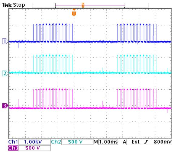
Figure 9.49: Voltage sharing of diode pair  $D_{b1}$ . Dark blue =  $v_{D_{b1}}$ , light blue =  $v_{D_{b11}}$ , purple =  $v_{D_{b12}}$ .
