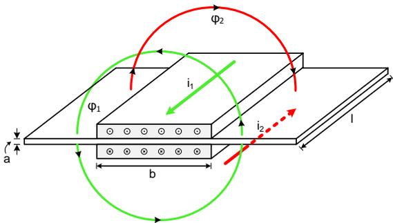
Figure C.3: One flat wire with identical return path
