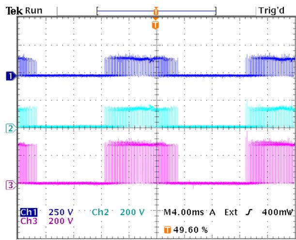
Figure 9.8: Voltage sharing of switch pair  $S_{b2}$ . Dark blue =  $v_{S_{b21}}$ , light blue =  $v_{S_{b22}}$ , purple =  $v_{S_{b2}}$ .
