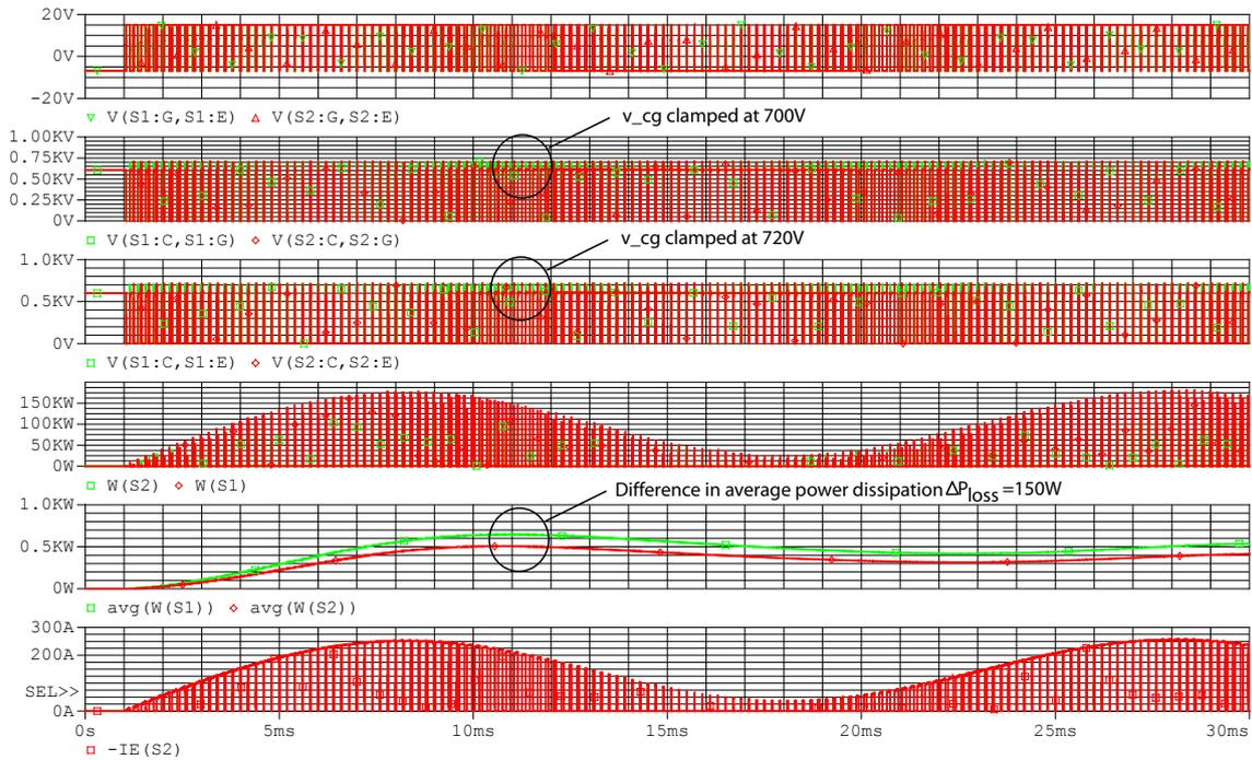
Figure 4.51: Simulation of the zener clamped snubber. (1)  $v_{ge1}$  and  $v_{ge2}$ , (2)  $v_{cg1}$  and  $v_{cg2}$ , (3)  $v_{ce1}$  and  $v_{ce2}$ , (4)  $W_{S1}$  and  $W_{S2}$ , (5)  $W_{S1,avg}$  and  $W_{S2,avg}$  and (6)  $i_{c,S2}$ .
