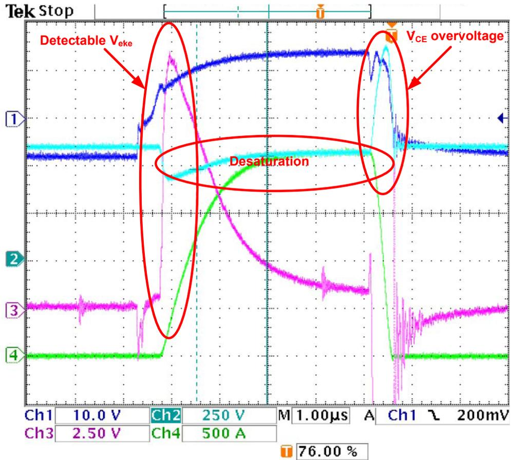
**Figure D.10:** Short circuit test for  $V_{in} = 600$ . Dark blue =  $v_{ge}$ , Light blue =  $v_{ce}$ , purple =  $v_{cke}$ , green =  $i_C$ . Notice that the offset for  $v_{ce}$  has changed, and that the desaturation occurs immediately.
