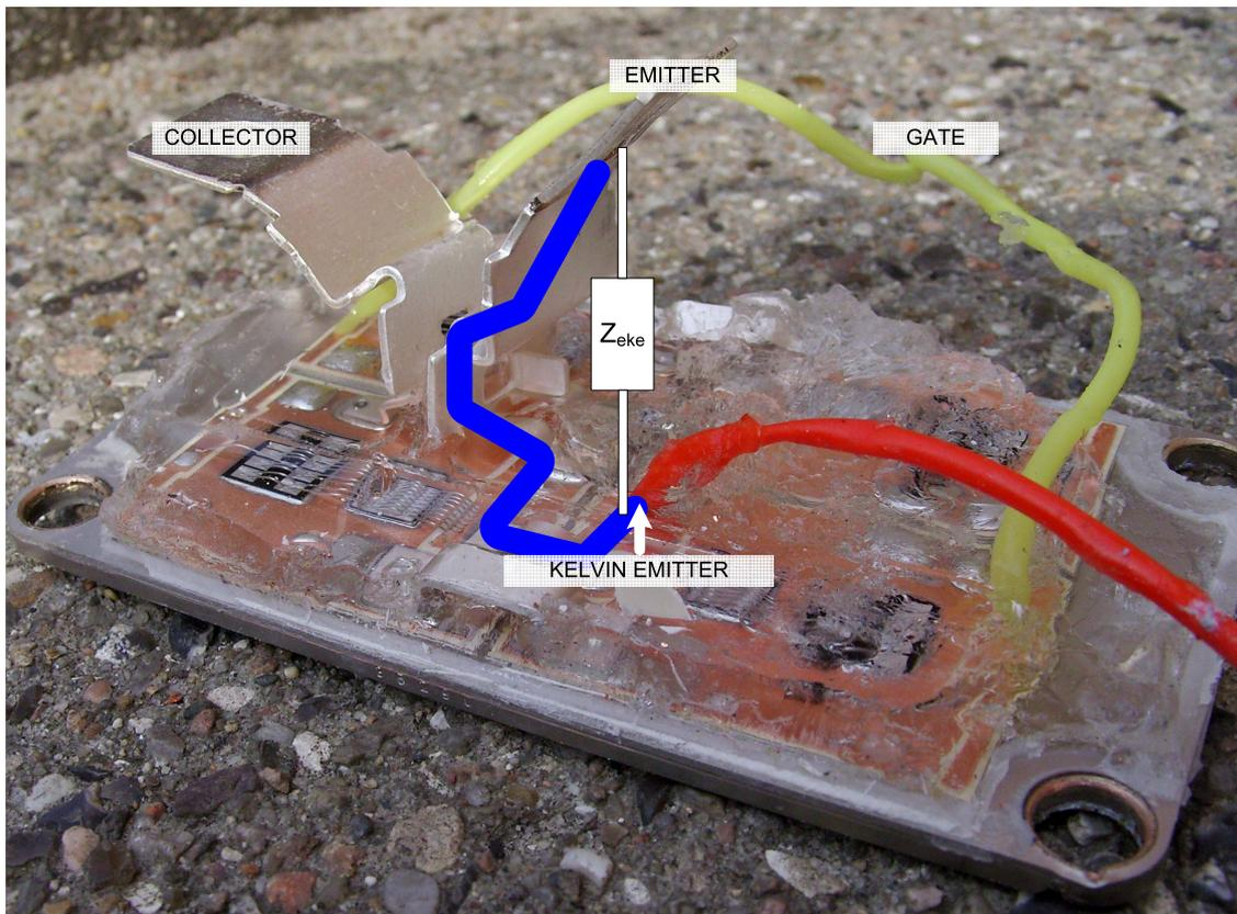
**Figure D.1:** Picture of the internal of a Semikron IGBT.  $Z_{eke}$  is shown by the blue line.
