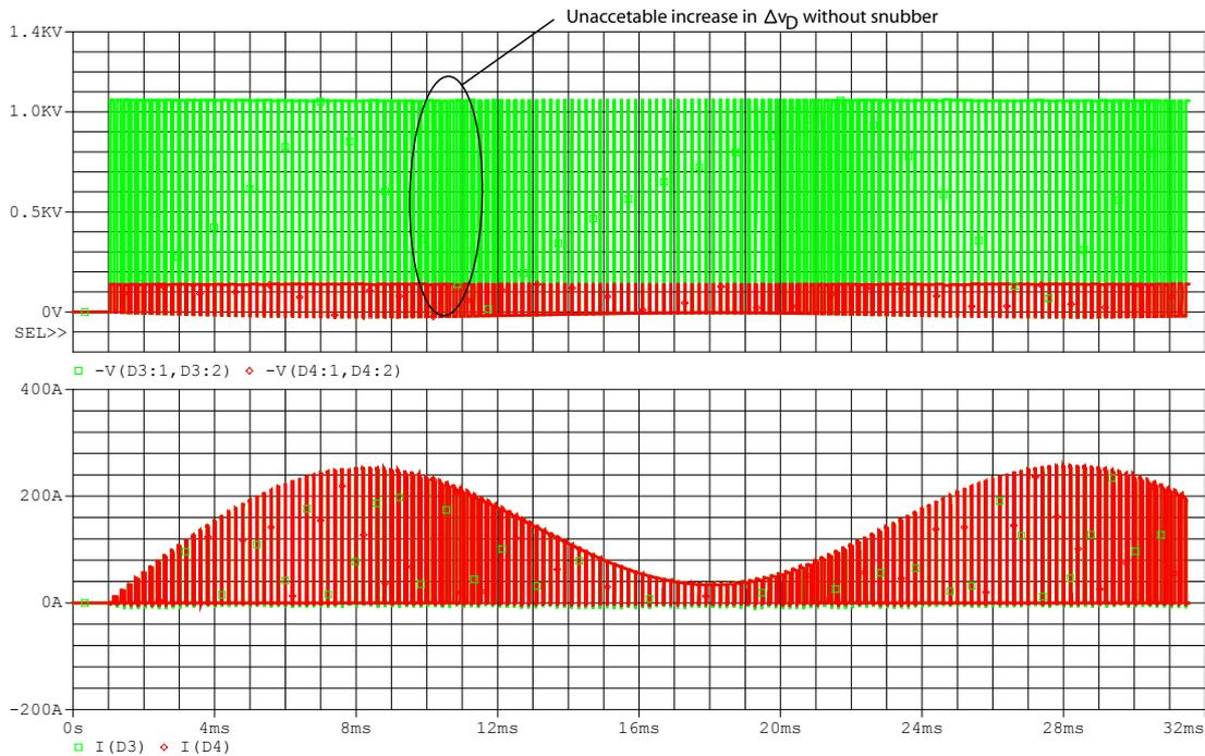
**Figure 4.21:** Simulation of series connected diodes *without* passive snubbers. (1)  $v_{D3}$  and  $v_{D4}$ , (2)  $i_{D3}$  and  $i_{D4}$ .
