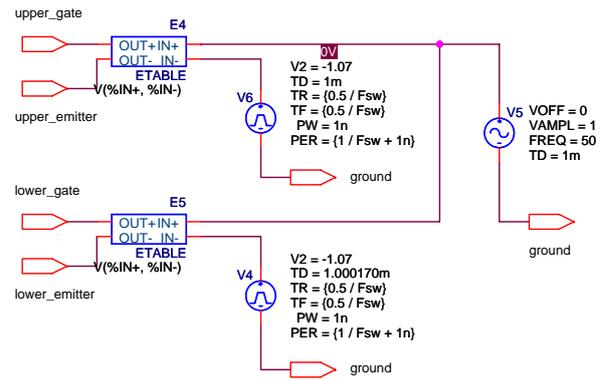
Figure 4.14: Simulation schematic for sinusoidal PWM circuit with  $t_d = 170ns$  and  $f_{mod} = 50Hz$ .
