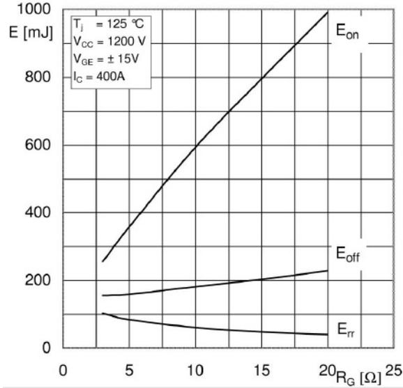
**Figure A.7:** Turn on and off energy as function of gate resistance for the SKM600GA176D [Semikron, 2006].
