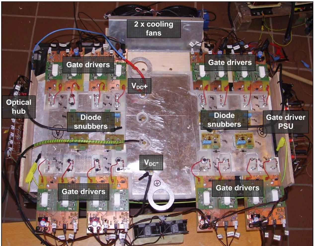
**Figure 8.12:** Final layout of the two-phased three-level inverter.
