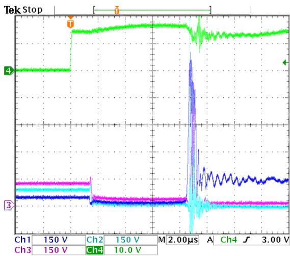
**Figure 9.65:** Short circuit test 2. Dark blue =  $v_{ce,Sa32}$ , light blue =  $v_{ce,Sa41}$ , purple =  $v_{ce,Sa42}$ , green = gate trigger signal.
