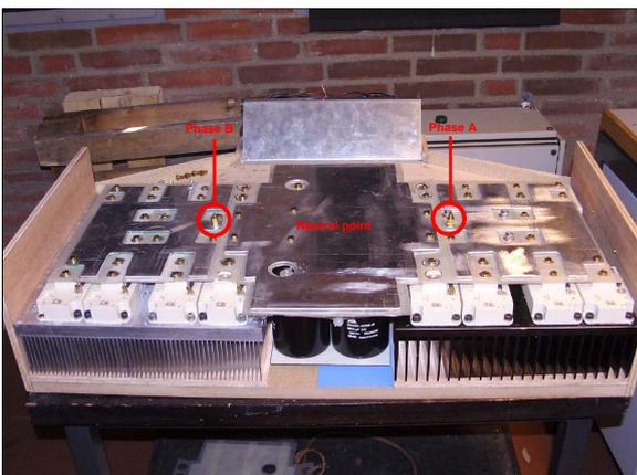
**Figure 8.8:** Layer two: The two phase outputs and the neutral point N.
