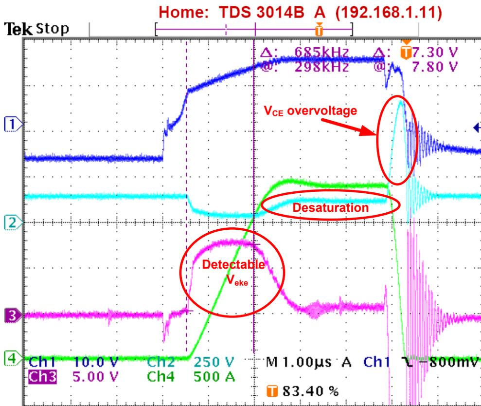
Figure D.9: Short circuit test for  $V_{in} = 150V$ . Dark blue =  $v_{ge}$ , light blue =  $v_{ce}$ , purple =  $v_{eke}$ , green =  $i_C$ .
