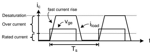
**Figure B.1:** Desaturation by fast fault with small inductance. Desaturation occurs immediately after short circuit.
