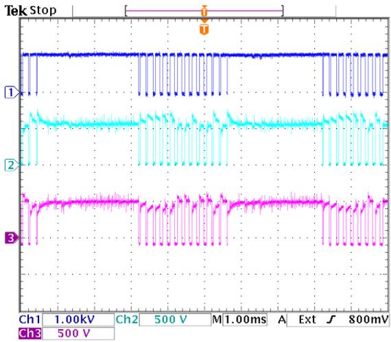
**Figure 9.31:** Voltage sharing of switch pair  $S_{a2}$ . Dark blue =  $v_{Sa2}$ , light blue =  $v_{Sa21}$ , purple =  $v_{Sa22}$ .
