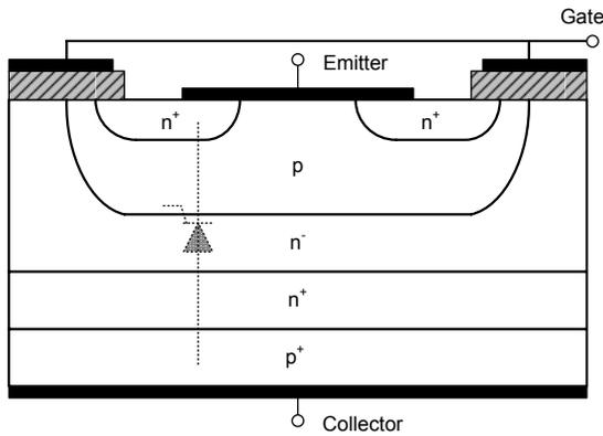
**Figure 5.7:** Physical structure of IGBT (freely after [Ned Mohan, 2003]).
