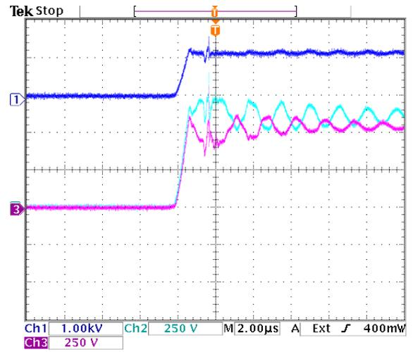
**Figure 9.30:** Zoom of turn off transition of switch pair  $S_{a1}$ . Dark blue =  $v_{Sa1}$ , light blue =  $v_{Sa11}$ , purple =  $v_{Sa12}$ .
