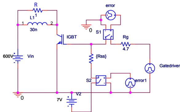
**Figure 5.14:** Simulation schematic of soft shut down protection.  $R_{SS} = 4.7\Omega(Y)$ ,  $15\Omega(\diamond)$ ,  $50\Omega(\nabla)$ ,  $75\Omega(\Delta)$ ,  $100\Omega(*)$ ,  $263\Omega(+)$  used for parameter sweep analysis.
