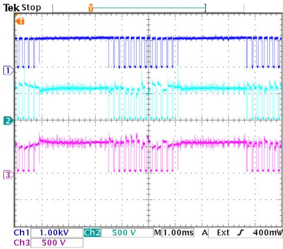
Figure 9.47: Voltage sharing of switch pair  $S_{b4}$ . Dark blue =  $v_{S_{b4}}$ , light blue =  $v_{S_{b41}}$ , purple =  $v_{S_{b42}}$ .
