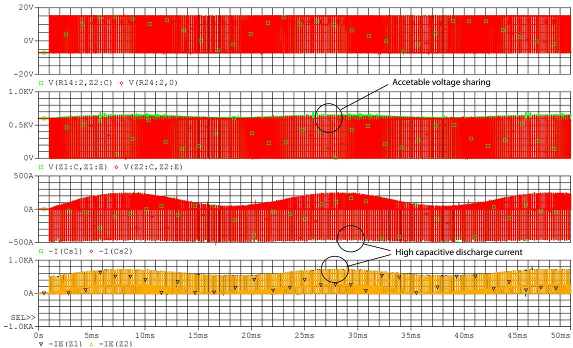
**Figure 4.15:** Simulation of passive snubber for series connected IGBTs. (1)  $v_{ge1}$  and  $v_{ge2}$ , (2)  $v_{ce,Z1}$  and  $v_{ce,Z2}$ , (3)  $i_{Cs1}$  and  $i_{Cs2}$  and (4)  $i_{c,Z1}$  and  $i_{c,Z2}$ .
