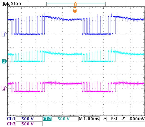
**Figure 9.20:** Voltage sharing of switch pair  $S_{b1}$ . Dark blue =  $v_{S_{b1}}$ , light blue =  $v_{S_{b11}}$ , purple =  $v_{S_{b12}}$ .
