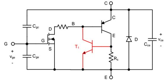
**Figure 5.8:** Circuit model including latch up transistor  $T_1$ .
