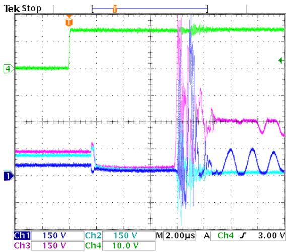
**Figure 9.59:** Short circuit test 1. Dark blue =  $v_{ce,Sb32}$ , light blue =  $v_{ce,Sb31}$ , purple =  $v_{ce,Sb32}$ , green = gate trigger signal.
