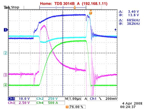
**Figure D.6:** Short circuit test for  $V_{in} = 400V$ . Dark blue =  $v_{ge}$ , light blue =  $v_{ce}$ , purple =  $v_{eke}$ , green =  $i_C$ .
