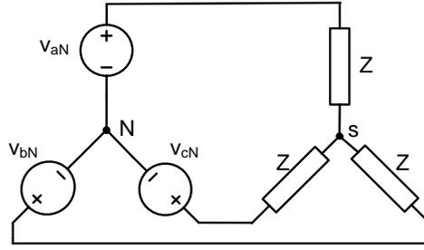
**Figure 2.4:** Three phase voltage source with star connected load.
