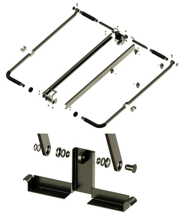
The exploded view of joint at the bottom rear end part shows the principle of how all the joint ares made. This principle gives the cart joints with no play and this is ensures that the Compact Cleaning Cart is stable.
