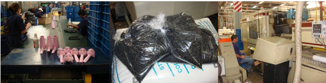
Figure 35 – (From left) Hair dryer casing shells; Plastic pellets for injection molding; Injection molding machine (Own photos).
