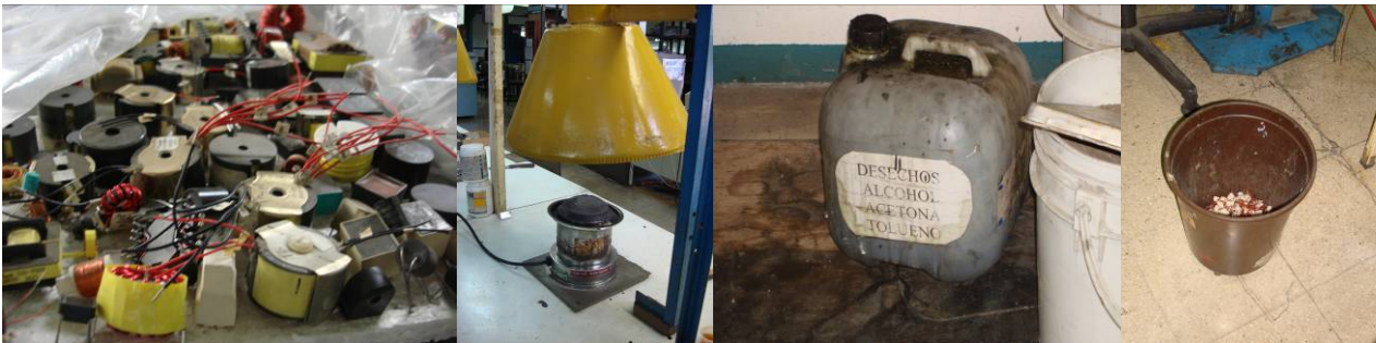
Figure 36 – (From left) Toroidal inductors; Soldering station with fume exhaust; Chemical waste collection canister for alcohol and acetone; Discarded products (Own photos).
