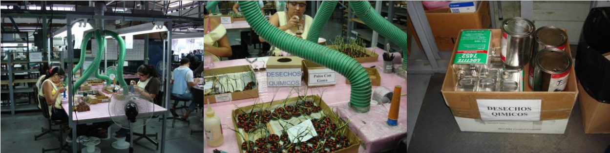
Figure 39 – (From left) Production line, plant 1; Production line close-up, showing fume exhaust; Chemical waste collection (Own photos).
