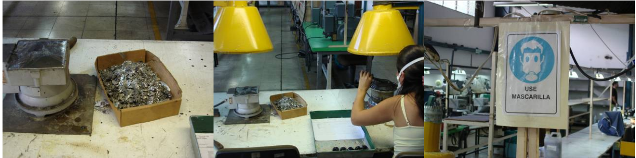
Figure 37 – (From left) Solder residue; Soldering process under way; Information notice on use of personal protection equipment (Own photos).
