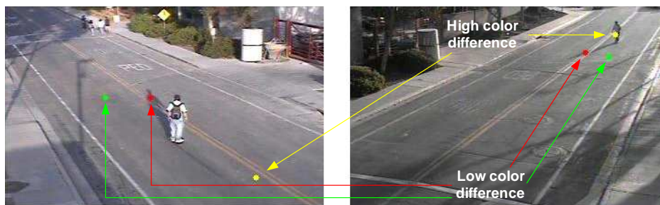
FIGURE B.1: Three points warped using the homography. The multi-view shadow suppression assumes that there is a low color difference between points that are on the ground plane (the red and green points) and a high difference for pixels mapping to an off-plane object (the yellow point).
