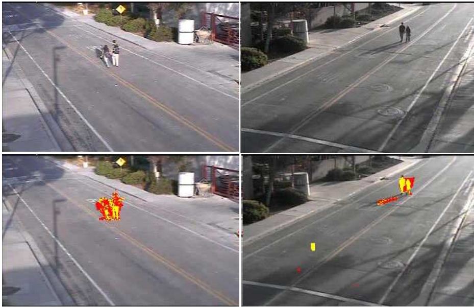
FIGURE B.4: Result of the shadow segmentation. Foreground is marked as yellow and foreground removed by the shadow suppression is marked as red.
