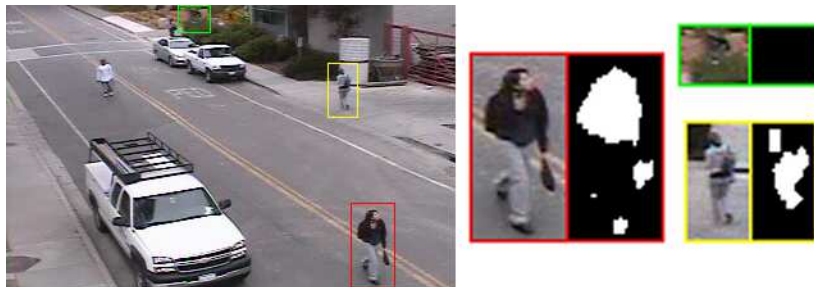
FIGURE 5.24: Example of objects that are difficult to segment. The green box shows a cyclist which is very hard to see due to his size. Two typical examples of background camouflage of persons with background colored clothes is also shown (yellow and red box).
