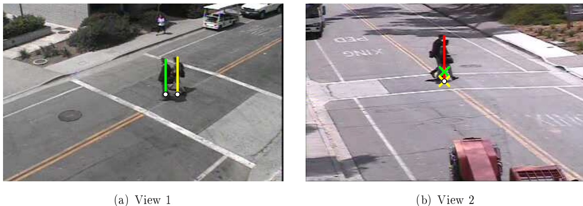
FIGURE 7.5: The problem of groups being tracked as a single object in one view. The crosses in view 2 indicate intersection points obtained by warping the two principal axes in view 1.
