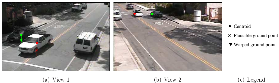
FIGURE 7.12: The plausible ground point can be used to solve ambiguities in the overlap matrix. The many-to-many overlap occurs in this situation because the vehicle with red centroid in view 1 occludes the lower part of the vehicle with the green centroid.
