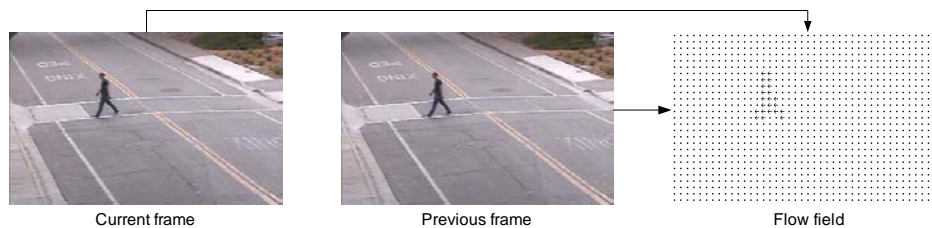
FIGURE 5.5: The concept of optical flow: for each pixel in a frame a motion vector is calculated. If the motion vector is large enough the pixel is considered foreground.
