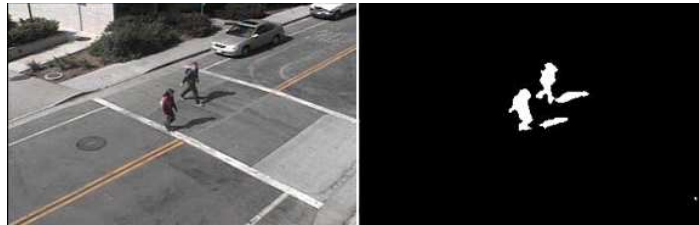
FIGURE 5.11: Though the Codebook method is able to cope with shadows to some extent, it is not able to handle strong cast shadows from moving objects like in the example provided above. Because the allowed illumination variation in the codewords can not be lowered enough to include such shadows without corrupting the background model.
