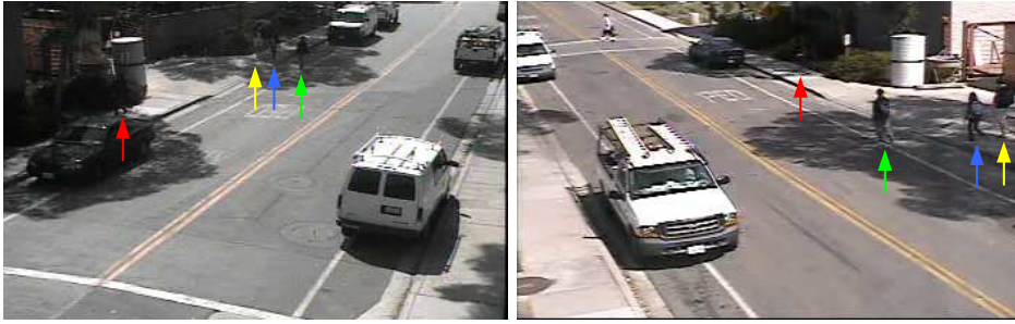
FIGURE 8.9: Example of strong background shadow making detection of human objects hard. Two views are shown with four people. Arrows indicate how the people correspond between the two views. When the objects are visually large in a view they are easier to detect.
