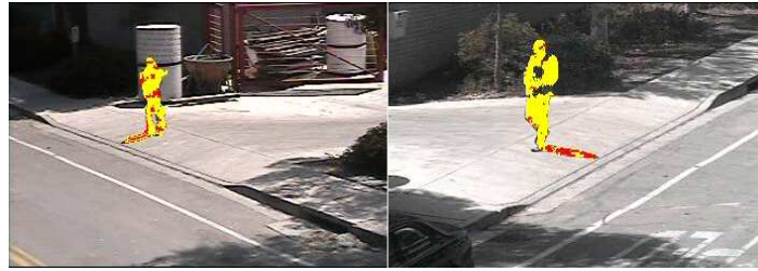
FIGURE 5.15: Result of shadow suppression with non-normalized saturation. The yellow color is the foreground segmented by the Codebook method, and the red is the portion of the foreground classified as shadow. The frames match those in Figure 5.14(a). The thresholds for both views are set to: \alpha_V = 0.25 \beta_V = 0.97 \tau_S = 0.20 \tau_H = 0.20 .
