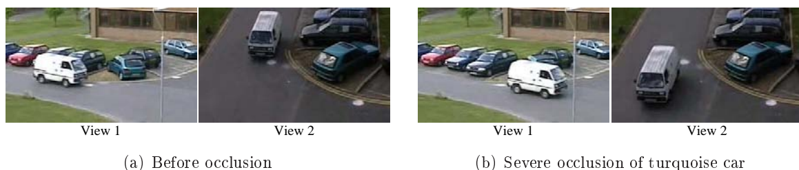
FIGURE 7.13: Example of severe occlusion. The occlusion causes a missing historically expected pairing of the turquoise car in view 1 and view 2.
