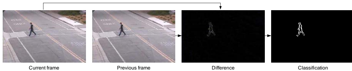
FIGURE 5.4: The concept of temporal differencing: the pixel-wise differences between a number of consecutive frames (usually two or three) is found. Differences above a threshold are classified as foreground.
