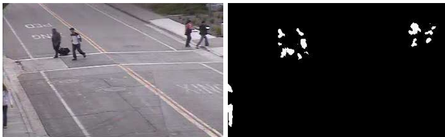
FIGURE 6.2: Example of foreground segmentation errors, where the human objects are divided into multiple disjoint blobs.
